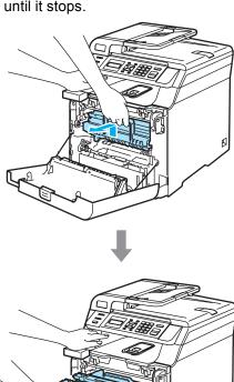
4 Release the gray lock lever (1) that is on the left side of the machine. Lift the front of the drum unit and pull the drum unit completely out of the machine using the green handles on the drum unit.
