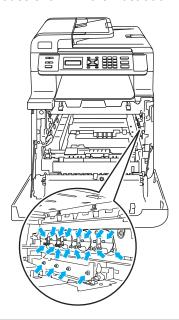
4 Hold the green parts of the belt unit with both hands and lift the belt unit up, then pull it out.
