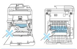
5 Using both hands, gently pull the jammed paper out of the fuser unit.
