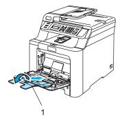
4 Put up to 3 envelopes, thick paper, labels or post cards in the MP tray with the top edge first and the print side face up.
