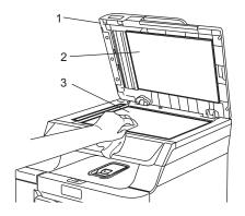
In the ADF unit, clean the white bar (1) and the scanner glass strip (2) underneath it with a soft lint-free cloth moistened with a non-flammable, ammonia-free glass cleaner.
