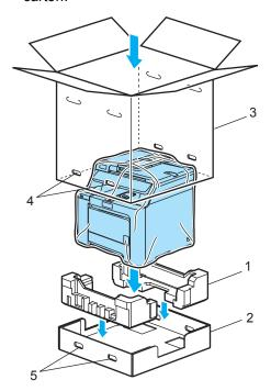
15 Put the two styrofoam pieces for the toner cartridges on the top of the machine. Match the right side of the machine to the "R" mark on one of the styrofoam pieces (1), and the left side of the machine to the "L" mark on the other styrofoam piece (2). Put the toner cartridges in the
