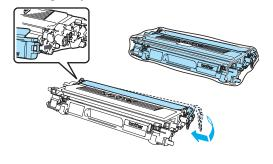
7 Hold the green parts of the belt unit with both hands and lift the belt unit up, then pull it out.
