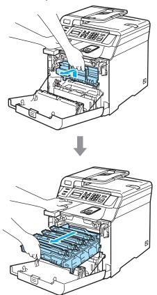
6 Release the gray lock lever (1) that is on the left side of the machine. Lift the front of the drum unit up and pull the drum unit completely out of the machine using the green handles on the drum unit.
