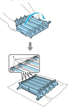
16 See the print sample to identify the color causing the problem. The color of the spots or toner stain is the color of the drum you should clean. For example, if the spots are cyan, you should clean the drum for cyan. Put the print sample in front of the drum, and the find the exact position of the poor print.
