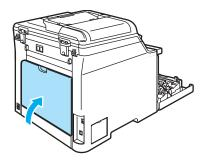
8 Put the drum unit and toner cartridge assembly back in the machine.
