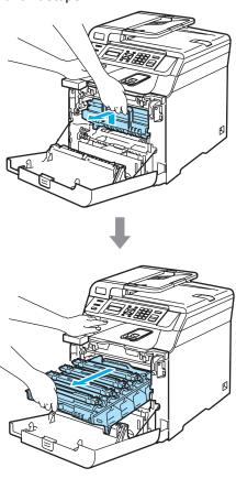
4 Release the gray lock lever (1) that is on the left side of the machine. Lift the front of the drum unit and pull the drum unit completely out of the machine using the green handles on the drum unit.
