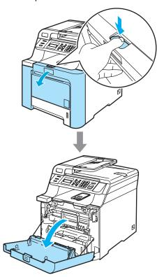
4 Hold the green handle of the drum unit. Lift the drum unit up and then pull it out until it stops.
