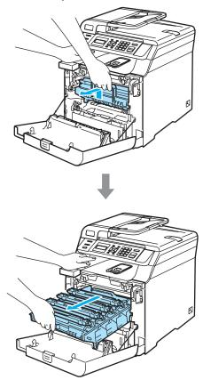
3 Hold the handle of the toner cartridge and pull it out of the drum unit. Repeat this for all the toner cartridges.
