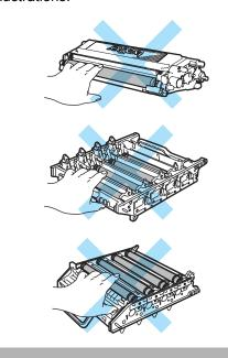
4 Hold the handle of the toner cartridge and pull it out of the drum unit. Repeat this for all the toner cartridges.
