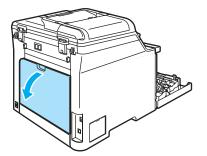
4 Pull down the two green levers, one on the left-hand-side and one on the right-hand-side, as shown in the illustration below, and then fold down the fuser cover (1).
