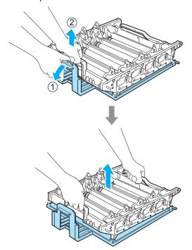
6 Hold the handle of the toner cartridge and slide the toner cartridge into the drum unit. Make sure that you match the toner cartridge color to the same color label on the drum unit, and make sure that you fold down the toner cartridge handle (A) once the toner cartridge is in place. Repeat this for all the toner cartridges.
