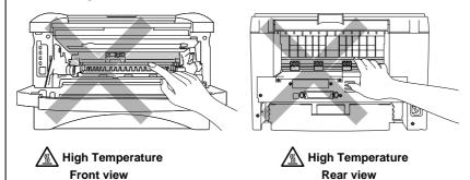
• There are high voltage electrodes inside the printer. Before cleaning the printer, make sure you have turned off the power switch and unplugged the power cord from the power outlet.
