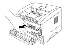
Fig. 4-7 Remove the drum unit assembly
