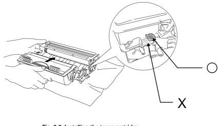
Fig. 3-9 Installing the toner cartridge into the drum unit
