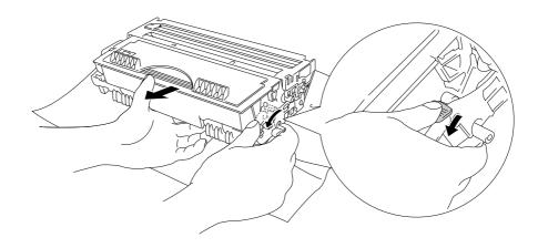
Fig. 3-4 Removing the old toner cartridge
