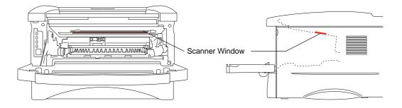
Fig. 3-21 Cleaning the scanner window
