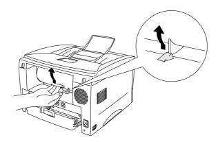
Fig. 1-18 Lift up the rear cover
