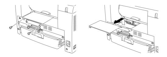
Fig. 2-6 Removing the Main Controller PCB
