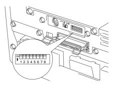
Fig. 2-3 Setting the Serial Interface Parameters
