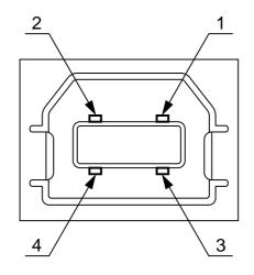
Fig. A-2 USB interface connector
