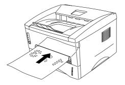
Fig. 1-22 Paper operation for the manual feed slot
