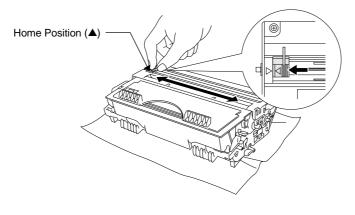
Fig. 3-22 Cleaning the primary corona wire
