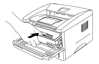
Fig 3-11 Re-install the drum unit assembly
