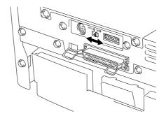
Fig. 2-2 Selecting the RS-422A (Apple) or RS-232C (IBM) Serial Interface
