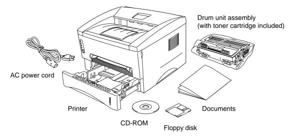
Fig. 1-1 Components in the Printer Carton
