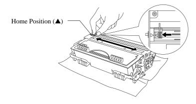
Fig. 3-10 Cleaning the primary corona wire
