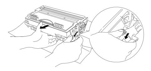
Fig. 3-15 Removing the toner cartridge
