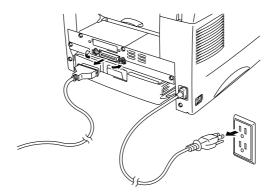
Fig. 2-5 Unplug the AC Cord and Disconnect the Interface Cable
