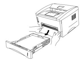
Fig. 4-6 Pull the jammed paper up and out
