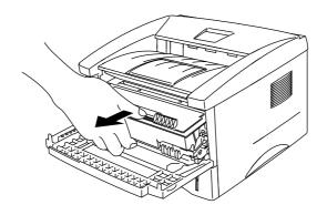
Fig. 3-13 Removing the drum unit assembly
