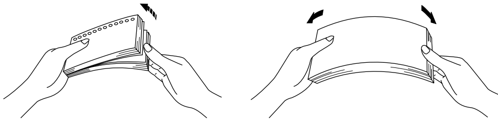
Fig. 1-5 Fan the Paper and Straighten the Paper
