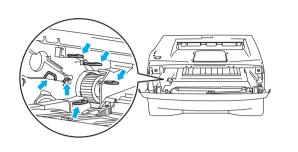
4 Push down the blue lock lever and take the toner cartridge out of the drum unit.
