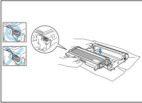
11) Put the drum unit and toner cartridge assembly back in the printer.
