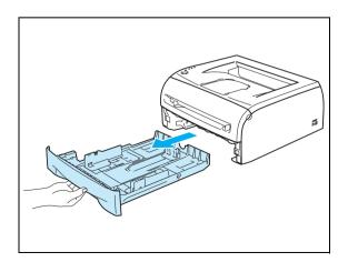
3 While pressing the blue paper-guide release lever, slide the paper guides to fit the paper size. Check that the guides are firmly in the slots.
