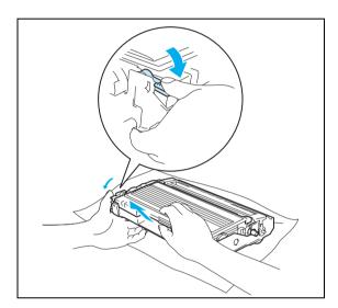
10 Put the toner cartridge back into the drum unit until you hear it lock into place. If you put it in properly, the lock lever will lift automatically.
