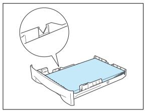
6 Put the paper tray firmly back in the printer. Check that it is completely in the printer.
