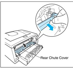
Pull the jammed paper out of the fuser unit. If the jammed paper cannot be pulled out easily, push down the tab with one hand as you gently pull the paper out with other.
