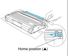
8 Put the drum unit and toner cartridge assembly back in the printer. Close the front cover of the printer.
