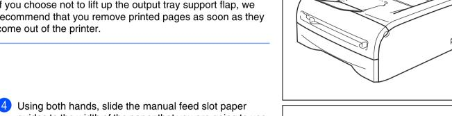
Using both hands, slide the manual feed slot paper guides to the width of the paper that you are going to use.
