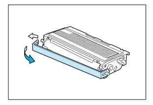
6 Put the new toner cartridge firmly into the drum unit until you hear it lock into place. If you put it in properly, the lock lever will lift automatically.
