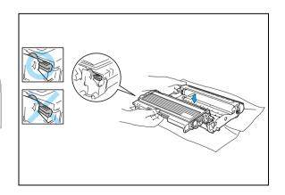
7 Put the drum unit and toner cartridge assembly in the printer.
