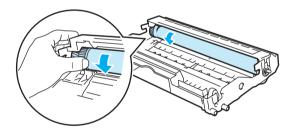
When you have located the mark on the drum that matches the print sample, wipe the surface of the OPC drum with a cotton swab until the dust or paper powder on the surface comes off.
