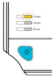
If the LED shows this message, the printer has nearly run out of toner and will continue to print until it has reached the end of its life. Buy a new toner cartridge and have it ready before you get a **Toner Life End** message. To replace the toner cartridge, see *Replacing the toner cartridge* on page 62.
