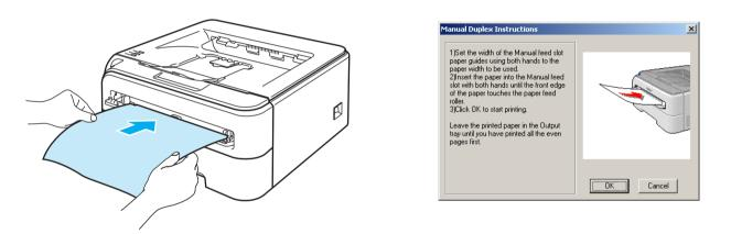
Semove the printed even-numbered pages from the output tray, and then put the first of the printed sheets back into the manual feed slot with the side to be printed on (the blank side) face up. Follow the instructions on the computer screen.
