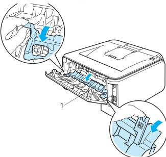
8 Pull the jammed paper out of the fuser unit.
