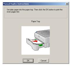
3 Remove the printed even-numbered pages from the output tray and put them back in the paper tray with the side to be printed on (blank side) face down. Follow the instructions on the computer screen.
