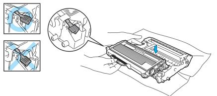
(12) Open the front cover. Put the drum unit and toner cartridge assembly back in the printer.
