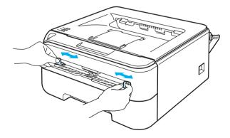
Using both hands, put one piece of paper or one envelope in the manual feed slot until the front edge of the paper or envelope touches the paper feed roller. When you feel the machine pull in the paper, let go.
