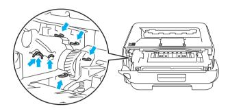
B) Push down the green lock lever and take the toner cartridge out of the drum unit.
