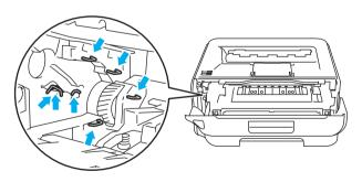
3 Clean the primary corona wire inside the drum unit by gently sliding the green tab from right to left and left to right several times.
