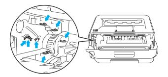
4 Push down the green lock lever and take the toner cartridge out of the drum unit.
