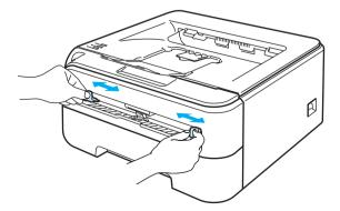
Using both hands, put one piece of paper or one transparency in the manual feed slot until the front edge of the paper or transparency touches the paper feed roller. When you feel the machine pull in the paper, let go.
