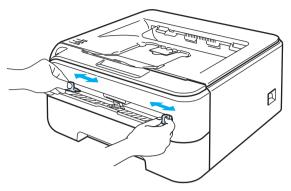
Using both hands put the paper in the manual feed slot with the side that is going to be printed on first facing up. Follow the instructions on the computer screen. Repeat this step until you have printed all the even-numbered pages.
