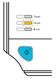
If the LED shows the message, it means the drum unit is near the end of its life. We recommend that you replace the drum unit with a new one before there is a noticeable deterioration in the print quality.
