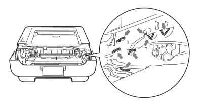
3 Clean the primary corona wire inside the drum unit by gently sliding the green tab from right to left and left to right several times.
