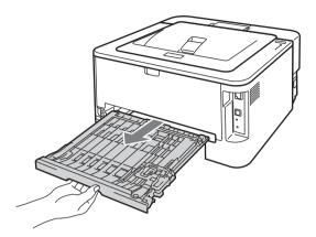
11 Pull the jammed paper out of the machine or the duplex tray.
