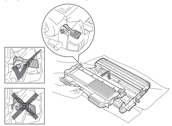
(18) Open the front cover. Put the drum unit and toner cartridge assembly back into the machine.
