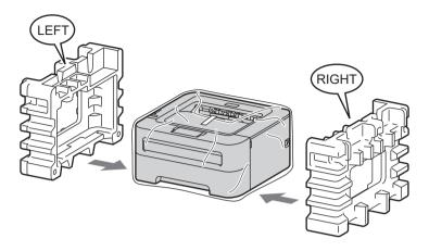
10 Put the machine into the original carton.
