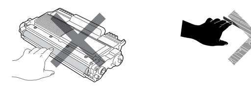
5 Put the print sample in front of the drum unit, and find the exact position of the poor print.
