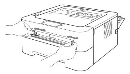
8 Using both hands, put one piece of A4 or Letter size paper in the manual feed slot until the top edge of the paper touches the paper feed roller. When you feel the machine pull in the paper, let go. The machine will start the Drum Cleaning process. The **Ready** LED flashes during the Drum Cleaning process.
