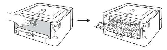
2 <For printing envelopes only> Pull down the two green levers, one on the left-hand side and one on the right-hand side, as shown in the illustration below.
