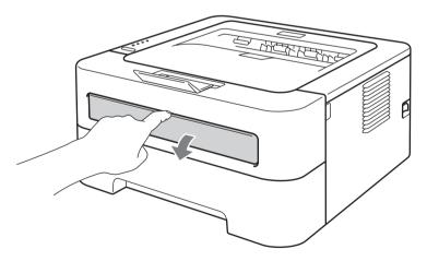
3 Using both hands, slide the manual feed paper guides to the width of the paper that you are going to use.
