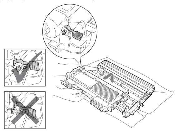
7 Put the drum unit and toner cartridge assembly back into the machine. Do not close the front cover yet.
