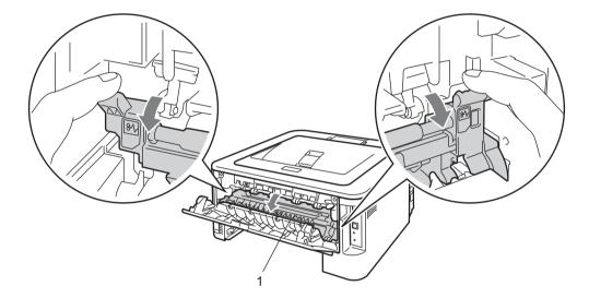
8 Using both hands, gently pull the jammed paper out of the fuser unit.
