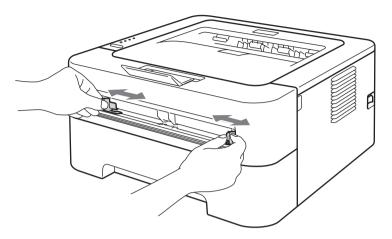
Using both hands, put one piece of paper in the manual feed slot until the front edge of the paper touches the paper feed roller. When you feel the machine pull in the paper, let go.
