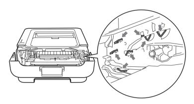
4 Put the protective material in the machine with the "REMOVE" text to the left, as shown in the illustration.
