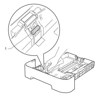
5 Wipe the two paper pick-up rollers (1) inside the machine.
