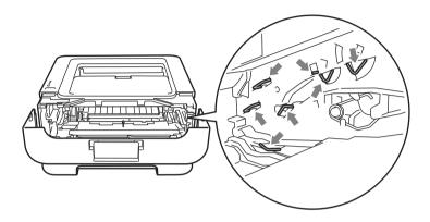
4 Push down the green lock lever and take the toner cartridge out of the drum unit.
