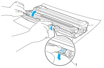
3 Push down the green-labeled lock lever (1) and take the toner cartridge out of the drum unit.
