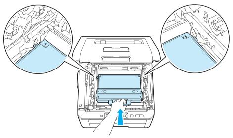
7 Put the belt unit back in the printer.
