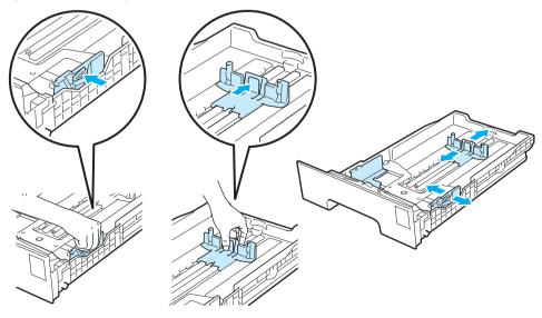
3 Put paper in the tray, and make sure that the paper is below the maximum paper mark (♥♥♥) (1). The side to be printed on must be face down.
