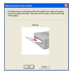
5 Remove the printed even-numbered pages from the output tray and then, in the same order <sup>1</sup>, put them back into the manual feed slot. Put the paper with the side to be printed on (the blank side) face up. Follow the instructions on the computer screen.
