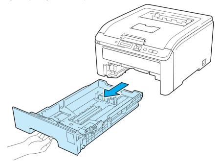
2 While pressing the green paper-guide release lever, slide the paper guides to fit the paper size. Make sure that the guides are firmly in the slots.
