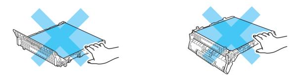
4 Unpack the new belt unit and put the new belt unit in the printer.
