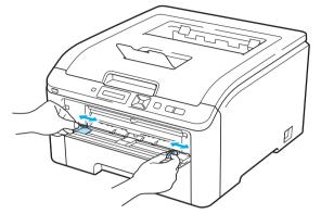
Using both hands, put one piece of paper in the manual feed slot until the front edge of the paper touches the paper feed roller. Wait until the machine automatically feeds the paper. When you feel the machine pull in the paper, let go.
