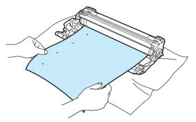
5 Turn the drum unit gear by hand while looking at the surface of the OPC drum (1).
