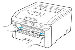
3 Using both hands, put one blank sheet of paper in the manual feed slot until the front edge of the paper touches the paper feed roller. Wait until the machine automatically feeds the paper. When you feel the machine pull in the paper, let go.
