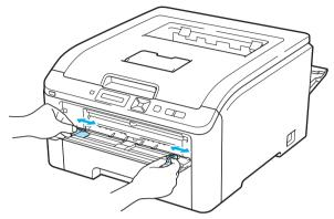
5 Using both hands, put one piece of paper or one envelope in the manual feed slot until the front edge of it touches the paper feed roller. When you feel the machine automatically pull it in, let go.
