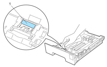
Wipe the two pick-up rollers (1) inside of the printer to remove dust.
