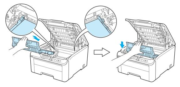
5 Slide each drum unit and toner cartridge assembly into the printer. Make sure that you match the toner cartridge color to the same color label on the printer. Repeat this for all the drum unit and toner cartridge assemblies.
