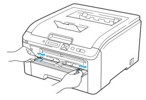
Using both hands put the paper in the manual feed slot with the side that is going to be printed on first facing up. Send the data to the printer, then follow the instructions on the computer screen. Repeat this step until you have printed all the even-numbered pages.
