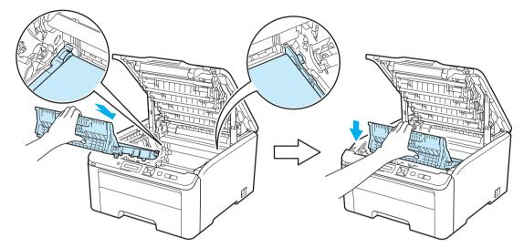
8 Slide each drum unit and toner cartridge assembly into the printer. Make sure that you match the toner cartridge color to the same color label on the printer. Repeat this for all the drum unit and toner cartridge assemblies.
