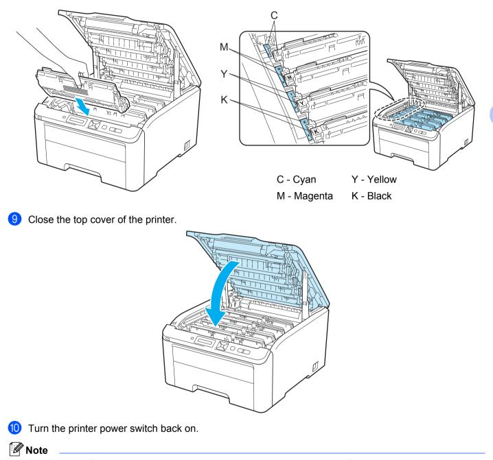
DO NOT turn off the printer power switch or open the top cover until the LCD shows Ready.
