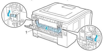
4 Using both hands, gently pull the jammed paper out of the fuser unit.
