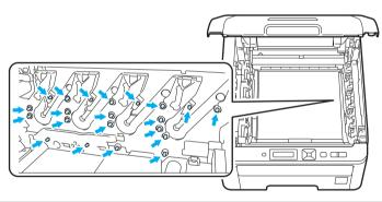
3 Clean the primary corona wire inside the drum unit by gently sliding the green tab from left to right and right to left several times.
