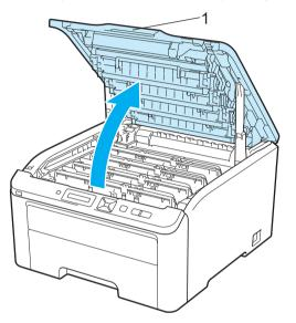
2 Take out the drum unit and toner cartridge assembly for the color shown on the LCD.
