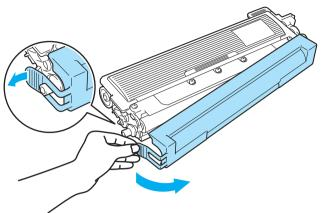
7 Put the new toner cartridge firmly into the drum unit until you hear it lock into place.
