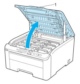
2 Take out the drum unit and toner cartridge assembly for the color shown on the LCD.
