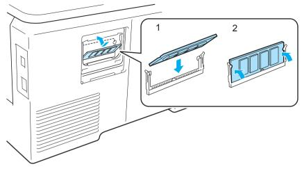
5 Put the metal (2) and then the plastic (1) SO-DIMM covers back on.
