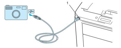
**2** Turn on the camera. The following message appears if Secure Function Lock is on. Press **OK**.
