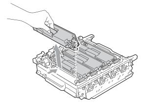
5 Unpack the new drum unit and remove the protective cover.
