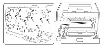
5 Hold the green handle of the belt unit with both hands and lift the belt unit up, then pull it out.
