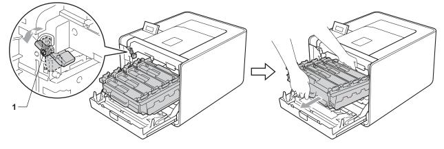
4 Hold the green handle of the belt unit with both hands and lift the belt unit up, then pull it out.
