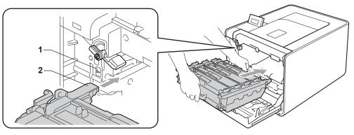
9 Turn the green lock lever (1) clockwise to the lock position.
