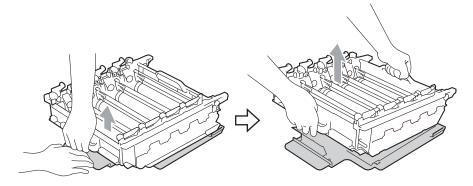
6 Hold the handle of the toner cartridge and slide it into the appropriate colored section of the drum unit until it clicks into place.
