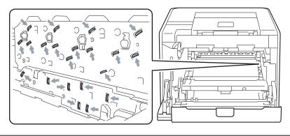
8 Hold the handle of the toner cartridge and slightly push it to unlock. Then pull it out of the drum unit. Repeat this for all the toner cartridges.
