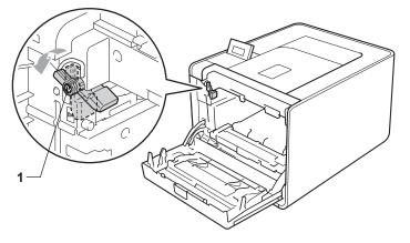
8 Match the guide ends (2) of the drum unit to the ► marks (1) on both sides of the machine, then gently slide the drum unit into the machine until it stops at the green lock lever.
