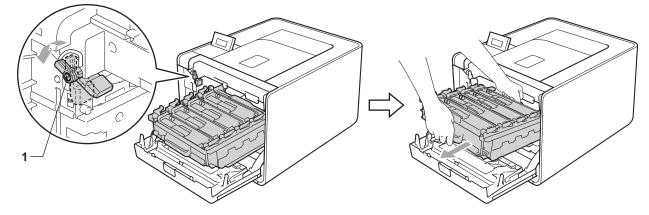
4 Hold the handle of the toner cartridge and slightly push it to unlock. Then pull it out of the drum unit. Repeat this for all the toner cartridges.
