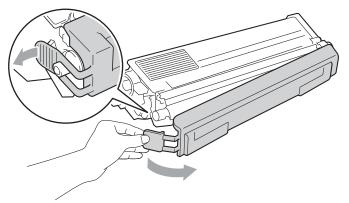
10 Hold the handle of the toner cartridge and slide the toner cartridge into the drum unit then slightly pull it toward you until you hear it click into place. Make sure that you match the toner cartridge color to the same color label on the drum unit. Repeat this for all the toner cartridges.
