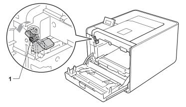
12 Match the guide ends (2) of the drum unit to the ► marks (1) on both sides of the machine, then gently slide the drum unit into the machine until it stops at the green lock lever.
