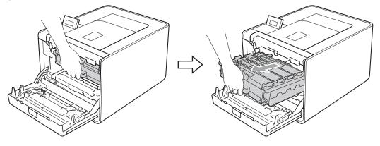
3 Turn the green lock lever (1) at the left of the machine counterclockwise to the release position. Holding the green handles of the drum unit, lift the front of the drum unit and remove it from the machine.
