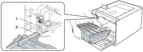
8 Turn the green lock lever (1) clockwise to the lock position.
