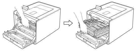
3 Hold the handle of the toner cartridge and slightly push it toward the machine to unlock it. Then pull it out of the drum unit. Repeat this for all the toner cartridges.
