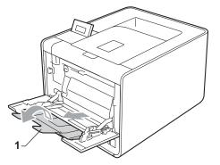
3 Lift up the support flap to prevent paper from sliding off the face-down output tray, or remove each page as soon as it comes out of the machine.
