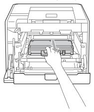
7 Unpack the new waste toner box and put the new waste toner box in the machine using the green handle. Make sure the waste toner box is level and fits firmly into place.
