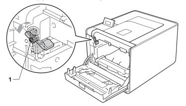
10 Match the guide ends (2) of the drum unit to the ► marks (1) on both sides of the machine, then gently slide the drum unit into the machine until it stops at the green lock lever.
