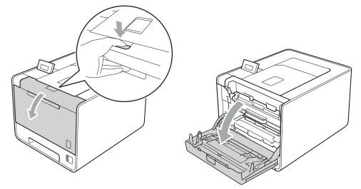
3 Hold the green handle of the drum unit. Pull the drum unit out until it stops.
