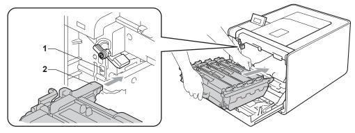
13 Turn the green lock lever (1) clockwise to the lock position.
