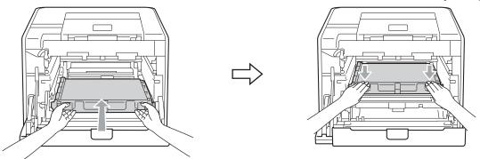
9 Make sure the green lock lever (1) is in the release position as shown in the illustration.
