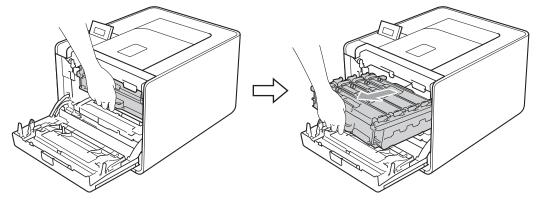
3 Hold the handle of the toner cartridge and slightly push it toward the machine to unlock it. Then pull it out of the drum unit. Repeat this for all the toner cartridges.
