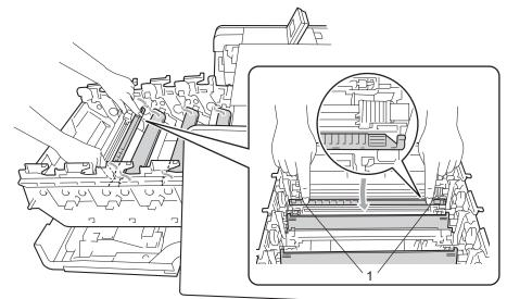
5 Clean the corona wire inside the drum unit by gently sliding the green tab from left to right and right to left several times.
