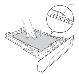
4 Put the paper tray firmly back in the machine. Make sure that it is completely inserted into the machine.
