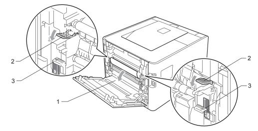
3 Pull the green tabs (2) at the left and right hand sides toward you and fold down the fuser cover (1).
