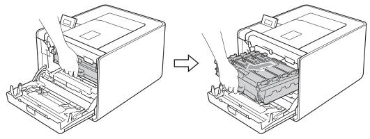
3 Turn the green lock lever (1) at the left of the machine counterclockwise to the release position. Holding the green handles of the drum unit, lift the front of the drum unit and remove it from the machine.
