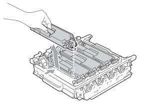
9 Turn the drum unit over by holding the green handles. Make sure that the drum unit gears (1) are on the left hand side.
