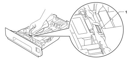
4 Wipe the two pick-up rollers (1) inside of the machine to remove dust.
