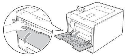
2 Pull out the MP tray support and unfold the flap (1).
