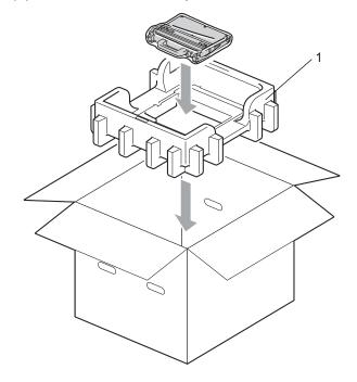
Wrap the machine with a plastic bag. Put the machine on the Styrofoam piece (1) and the Styrofoam piece (2) on the top of the machine. Match the front side of the machine to the "FRONT" mark on each Styrofoam piece.
