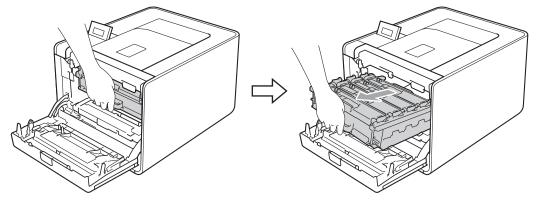
7 Turn the green lock lever (1) at the left of the machine counterclockwise to the release position. Holding the green handles of the drum unit, lift the front of the drum unit and remove it from the machine.
