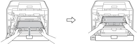
6 Make sure the green lock lever (1) is in the release position as shown in the illustration.
