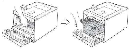
4 Turn the green lock lever (1) at the left of the machine counterclockwise to the release position. Holding the green handles of the drum unit, lift the front of the drum unit and remove it from the machine.
