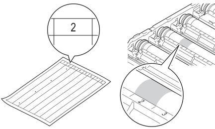
12 Turn the drum unit gear toward you by hand while looking at surface of the suspected area.
