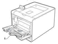
3 Lift up the support flap to prevent envelopes or thick sheets of paper from sliding off the face-down output tray. If the support flap is closed you should remove each envelope as soon as it comes out of the machine.
