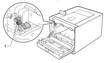
16 Match the guide ends (2) of the drum unit to the ► marks (1) on both sides of the machine, then gently slide the drum unit into the machine until it stops at the green lock lever.
