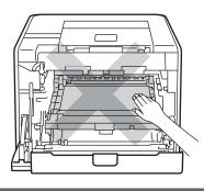
6 Make sure the green lock lever (1) is in the release position as shown in the illustration.
