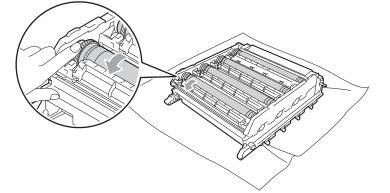
(13) When you have found the mark on the drum that matches the drum dot check sheet, wipe the surface of the drum gently with a cotton swab until the mark on the surface comes off.
