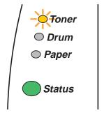
The **Toner** LED alternates turning on for 2 seconds and off for 3 seconds.
