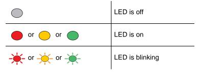
When the power switch is off or the printer is in Sleep mode, all the LEDs are off.
