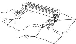
2 Turn the drum unit gear by hand while looking at the surface of the OPC drum
