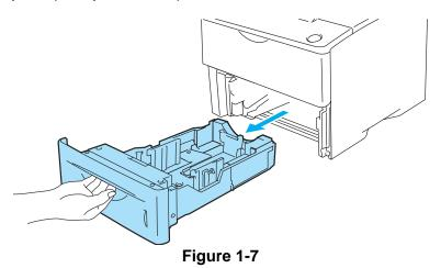
**3** While pressing the blue paper-guide release lever, slide the paper guides to fit the paper size. Check that the guides are firmly in the slots.
