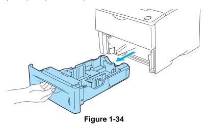
**3** While pressing the blue paper guide release levers, slide the paper guides to fit the transparency size. Check that the guides are firmly in the slots.
