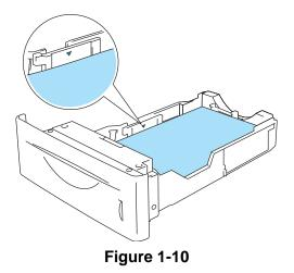
5 Put the paper tray firmly back in the printer. Check that it is inserted fully into the printer.
