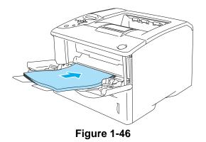
**3** Remove the printed even-numbered pages from the output tray and put them in the same order back into the MP tray. Place the paper with the side which will be printed on (the blank side) face up. Follow the instructions on the computer screen.
