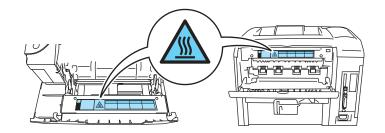
A There are high voltage electrodes inside the printer. Before you clean the printer, clear a paper jam or replace parts, make sure you have turned off the power switch and unplugged the printer from the AC power outlet/socket.
