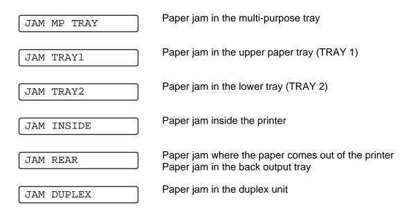
Paper may jam in the paper tray, inside the printer, in the back output tray or where the paper comes out of the printer. Check where the jam is and follow the instructions on the next few pages to remove the jammed paper.
