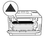
If the gray envelope levers inside the back cover are pulled down to the envelope position, lift these levers to the original position before pulling the green tabs down.
