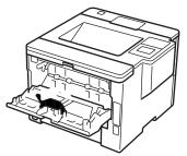
3. On the front of the machine, open the MP tray and lower it gently.
