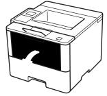
3. Pull out the MP tray support (1) and unfold the flap (2).
