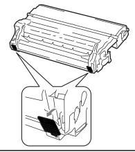
12. Wipe the surface of the drum gently with a dry cotton swab until the mark on the surface comes off.
