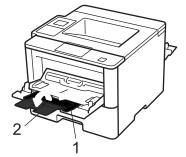
5. Slide the MP tray paper guides to fit the width of the envelopes that you are using. If the paper guide on the right side has a lever, press it and slide the paper guide.
