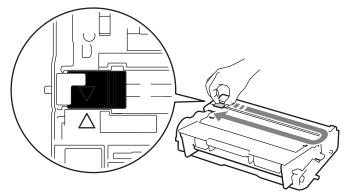
Be sure to return the tab to the Home position (▲). The arrow on the tab must be aligned with the arrow on the drum unit. If it is not, printed pages may have a vertical stripe.
