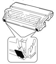
11. Wipe the surface of the drum gently with a dry cotton swab until the mark on the surface comes off.
