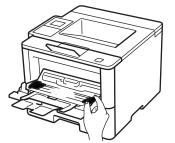
5. Load paper with the printing surface *face up* in the MP tray. When you use Letterhead or Preprinted paper, load the paper in the correct orientation as shown in the illustrations.
