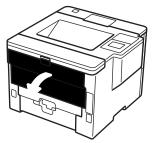
3. Pull the green levers at the left and right sides toward you to release the fuser cover.
