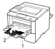
5. Slide the MP tray paper guides to fit the width of the paper that you are using. If the paper guide on the right side has a lever, press it and slide the paper guide.
