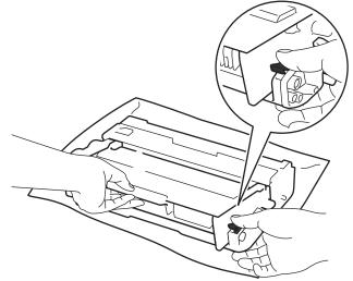
9. Turn the drum unit as shown in the illustration. Make sure that the drum unit gear is on the left side.
