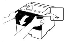
7. Remove the toner cartridge and drum unit assembly from the machine.
