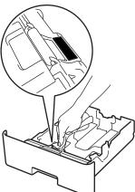
5. Wipe the two pick-up rollers inside the machine to remove dust.
