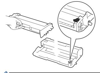
Make sure you put the toner cartridge in correctly or it may separate from the drum unit.
