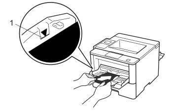
Load up to 10 envelopes in the MP tray with the printing surface face up. Make sure the envelopes are below the maximum paper mark (1). Loading more than 10 envelopes may cause paper jams.
