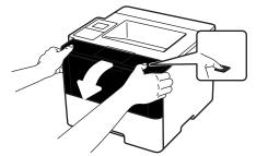
3. Remove the toner cartridge and drum unit assembly from the machine.
