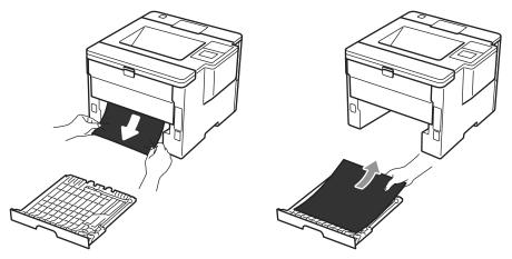
5. Remove paper that may have jammed under the machine due to static electricity.
