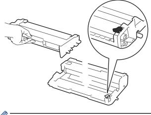
Make sure you put the toner cartridge in correctly or it may separate from the drum unit.
