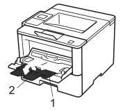
4. Slide the MP tray paper guides to fit the width of the paper you are using. If the paper guide on the right side has a lever, press it and slide the paper guide.
