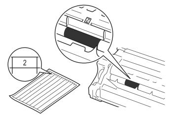
10. Turn the edge of the drum unit toward you while looking at the drum surface to find the mark.
