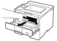
7. Push down the green lock lever and take the toner cartridge out of the drum unit.
