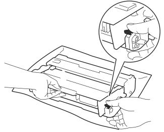
8. Turn the drum unit as shown in the illustration. Make sure that the drum unit gear is on the left side.
