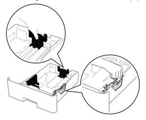
For Legal or Folio size paper, press the release button (1) in the bottom of the paper tray or the release lever (2) in the back of the tray, and then pull out the back of the paper tray. (Legal and Folio size paper are not available in some regions.)
