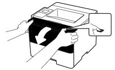
2. Remove the toner cartridge and drum unit assembly from the machine.
