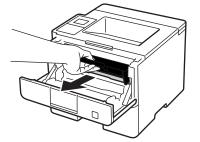
4. Push down the green lock lever and take the toner cartridge out of the drum unit.
