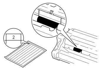
11. Turn the edge of the drum unit toward you while looking at the drum surface to find the mark.
