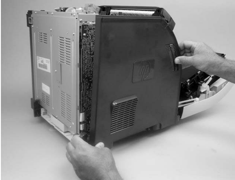
Figure 5-20 Remove the left cover (5 of 5)
