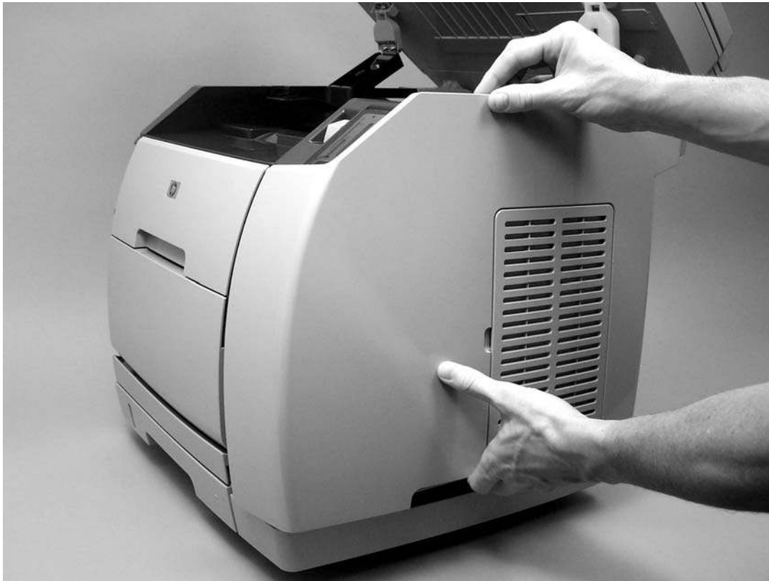
Remove the right-side cover (2 of 2)
