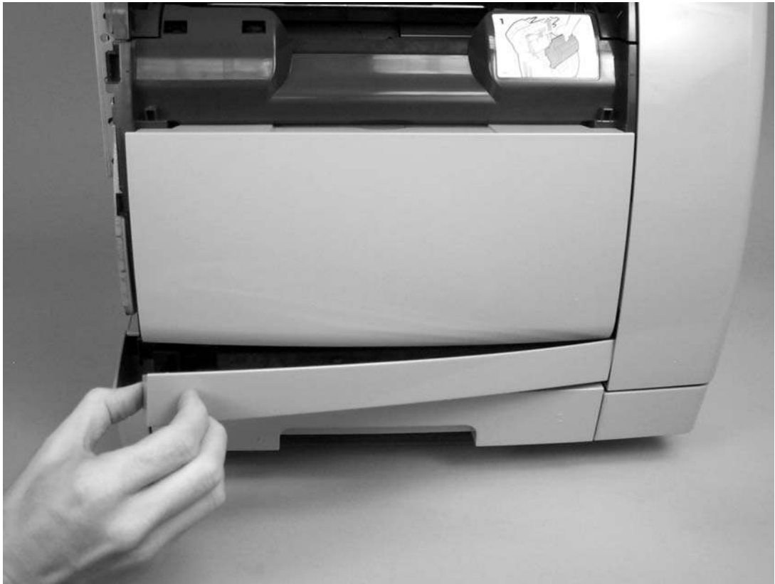
Disengage the right-side latch
