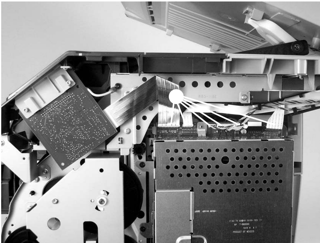
Remove the formatter cage (1 of 3)
