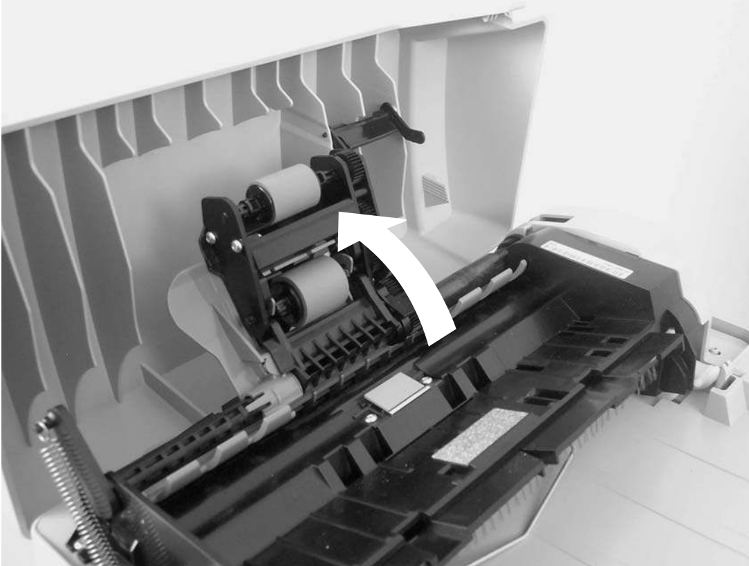
Remove the ADF separation pad (1 of 2)
