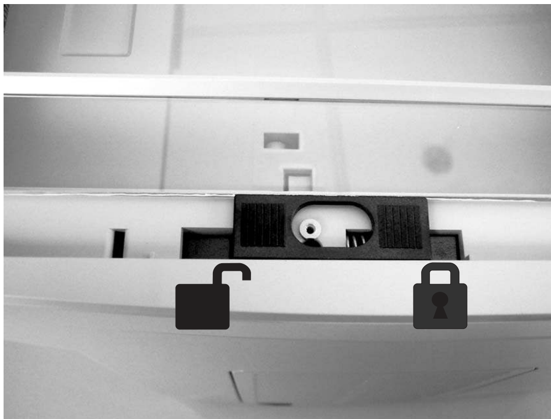
Figure 5-16 Install the ADF scanner glass
