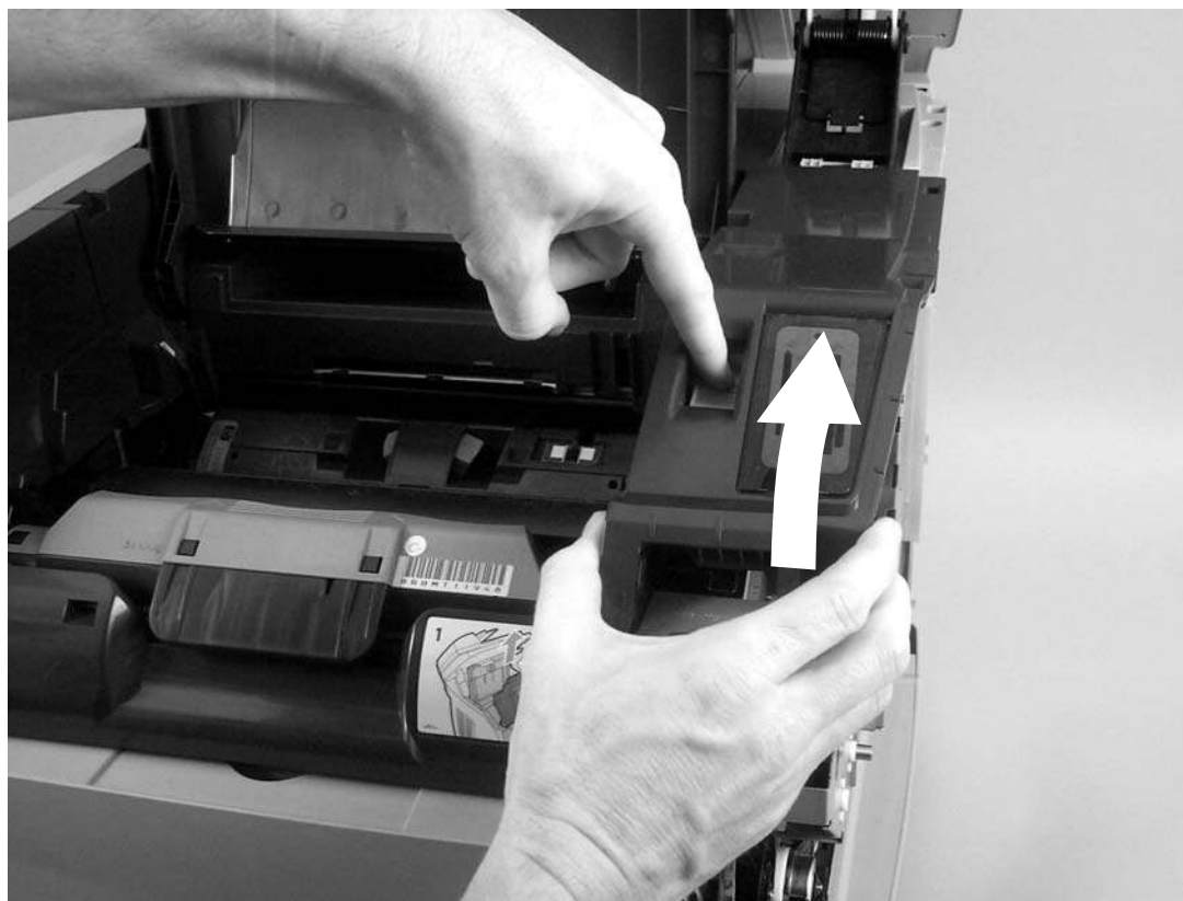
Remove the right upper cover (2 of 2)
