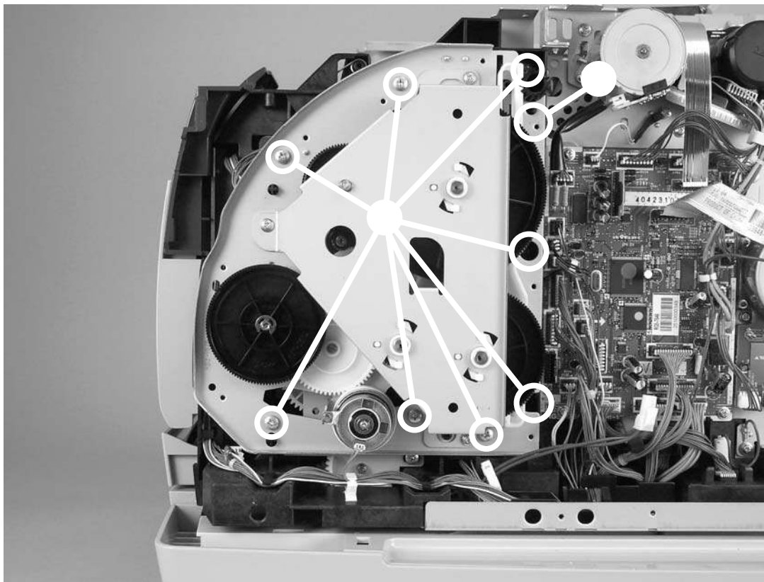
Remove the gear assembly (2 of 2)
