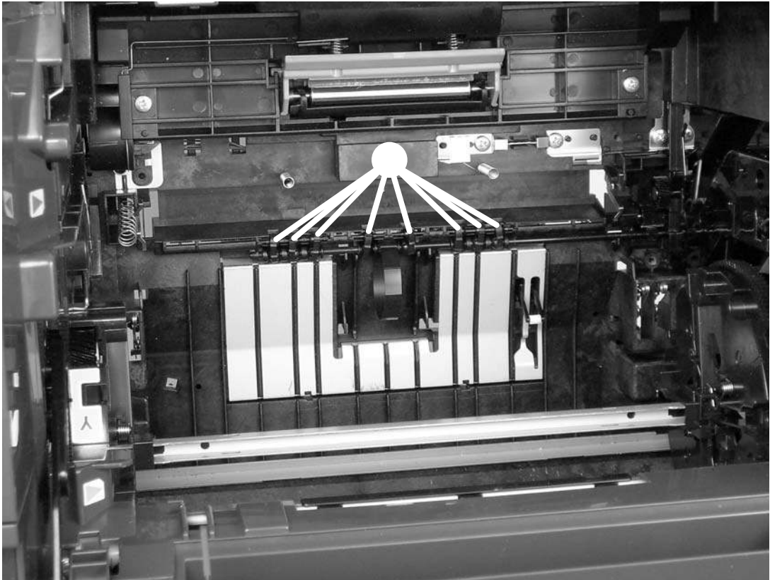
Replacing the feed-drive shaft and belts (7 of 8)
