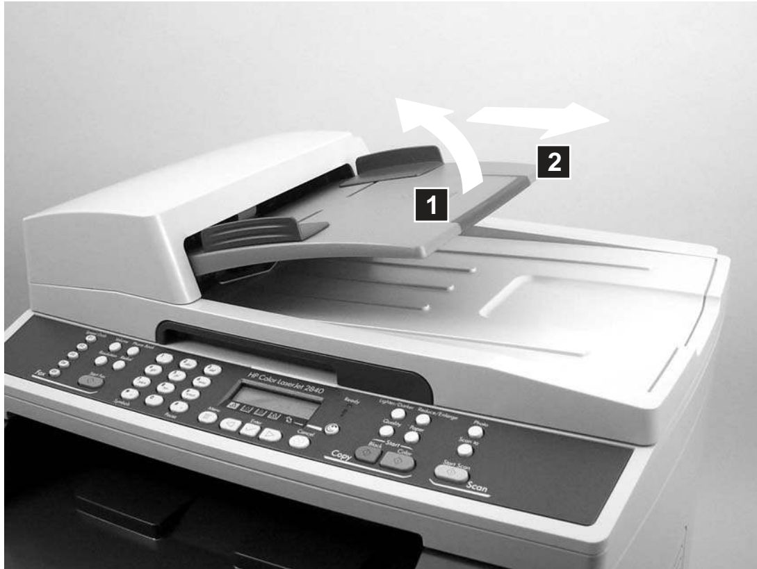
Remove the ADF pickup-roller assembly (1 of 5)
