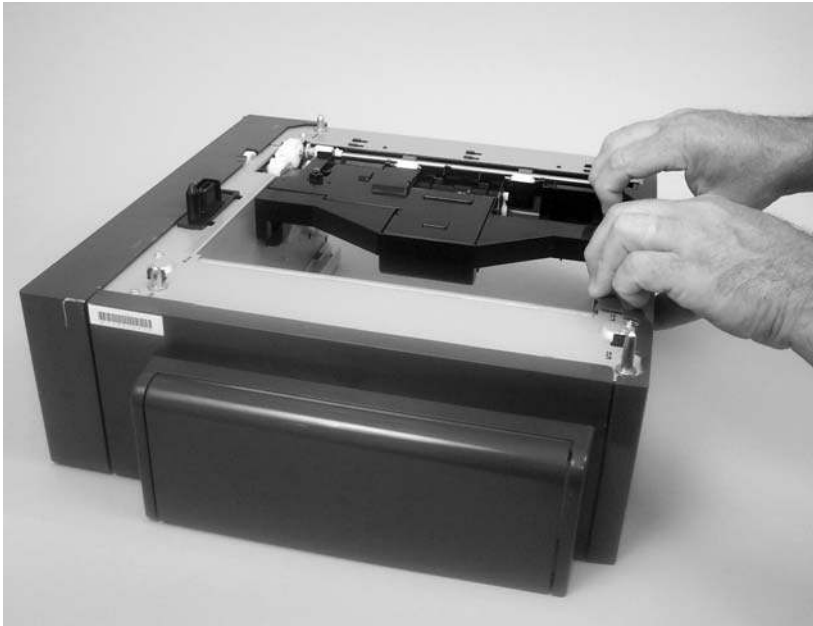
Figure 5-115 Remove the 500-sheet feeder left cover (2 of 5)
