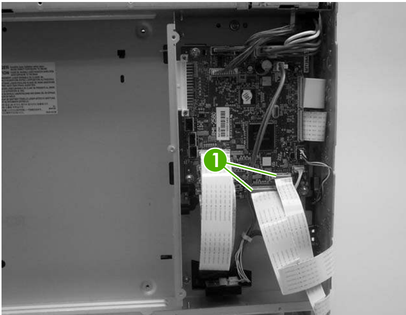
Figure 5-88 Remove the high-voltage power supply (1 of 3)
