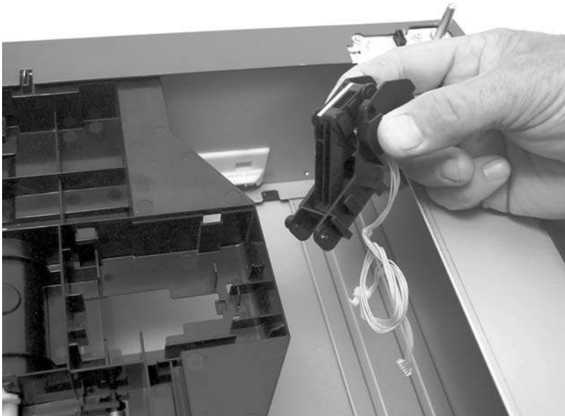
Figure 5-127 Remove the media sensor (500-sheet feeder) (4 of 4)
