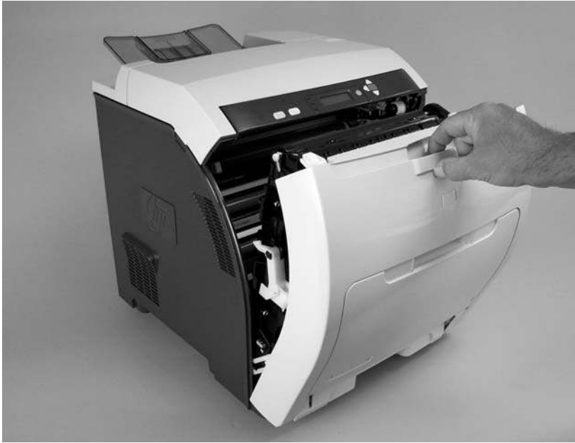
Figure 5-2 Remove the print cartridges (1 of 2)
