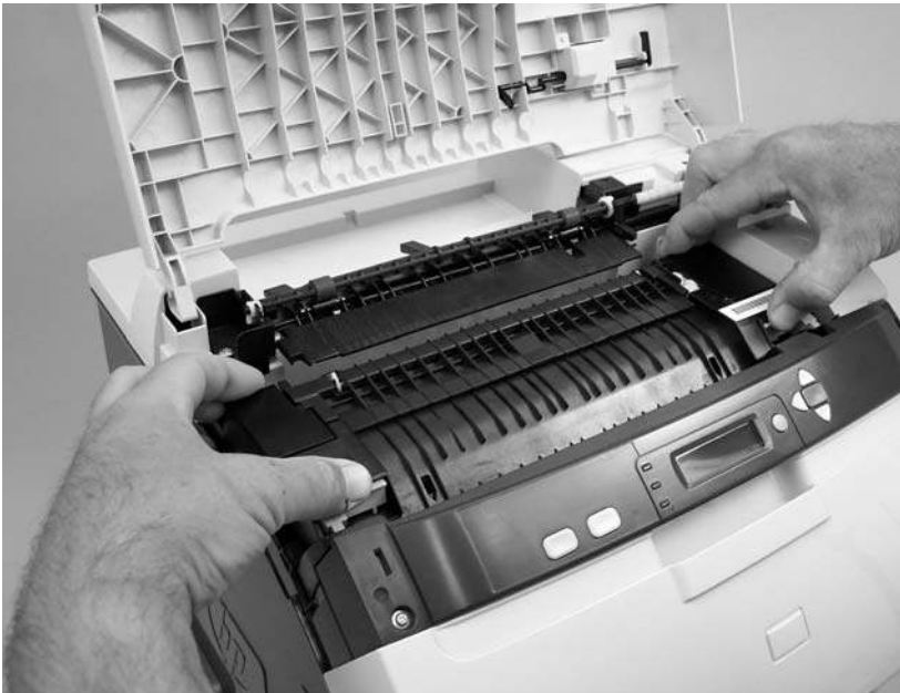
Figure 5-12 Remove the upper cover (2 of 5)
