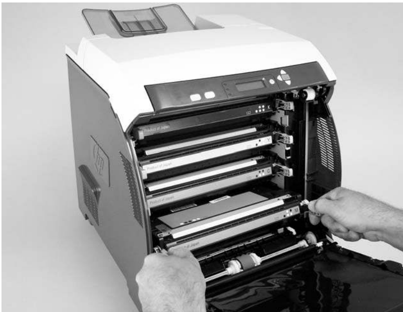
Figure 5-3 Remove the print cartridges (2 of 2)
