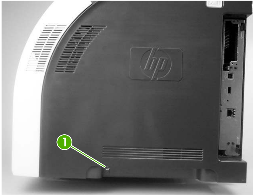
Figure 5-23 Remove the right cover (1 of 4)
