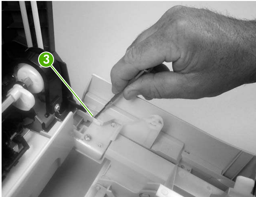
Figure 5-32 Remove the duplex fan (2 of 3)
