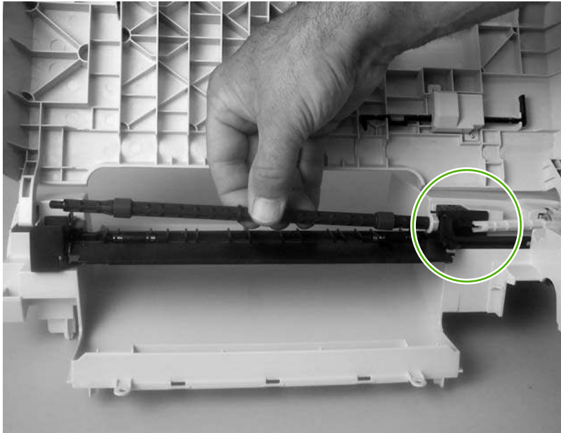
Figure 5-36 Remove the duplex-reverse-drive assembly (2 of 5)
