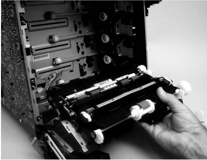
Figure 5-57 Remove the pickup-and-feed assembly (8 of 8)
