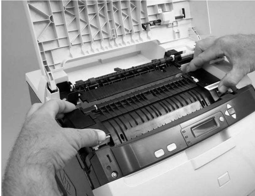
Figure 5-30 Remove the fuser
