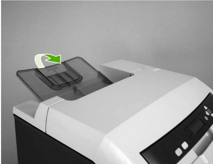
Figure 5-11 Remove the upper cover (1 of 5)
