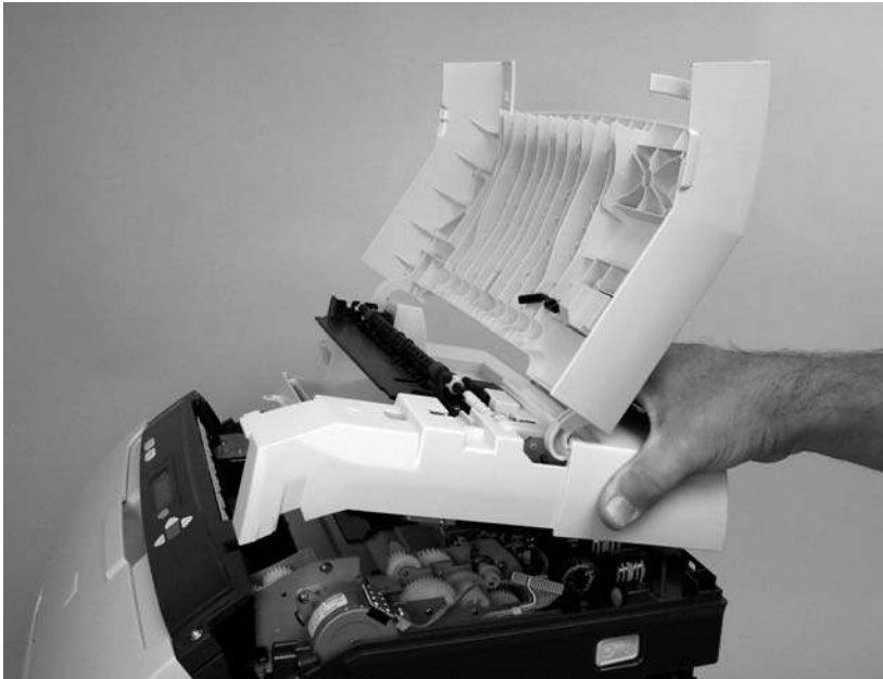
Figure 5-15 Remove the upper cover (5 of 5)
