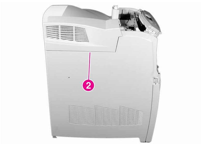
Figure 6-7 Remove the rear top cover (3 of 3)
