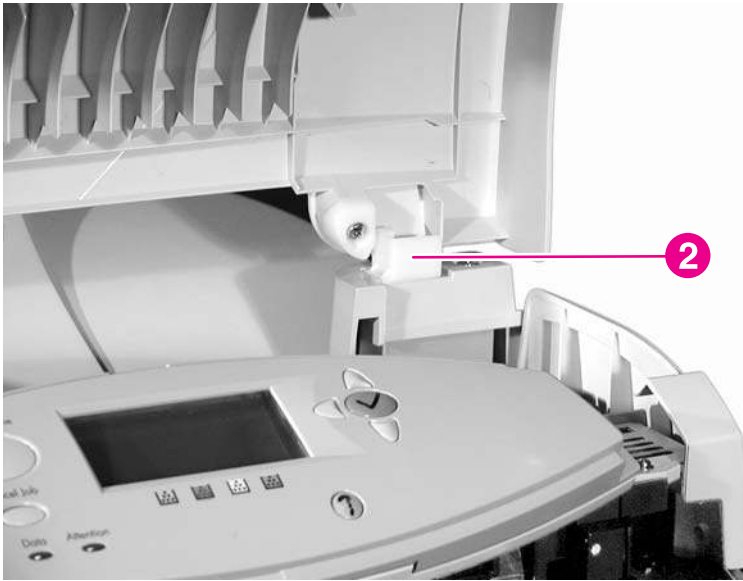
Figure 6-4 Remove the top cover (2 of 2)
