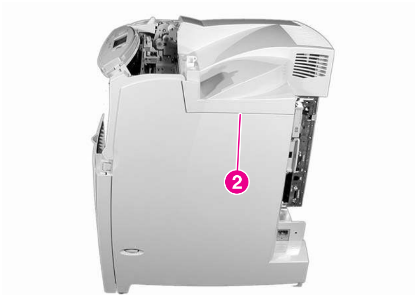
Figure 6-6 Remove the rear top cover (2 of 3)
