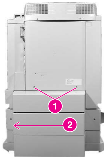
Figure 6-3. Removing and replacing the rear cover
