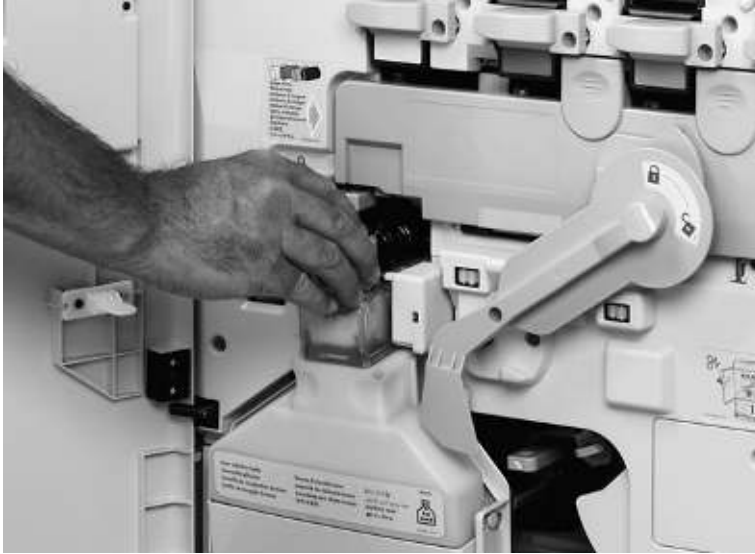
Figure 77. Remove the waste toner bottle
