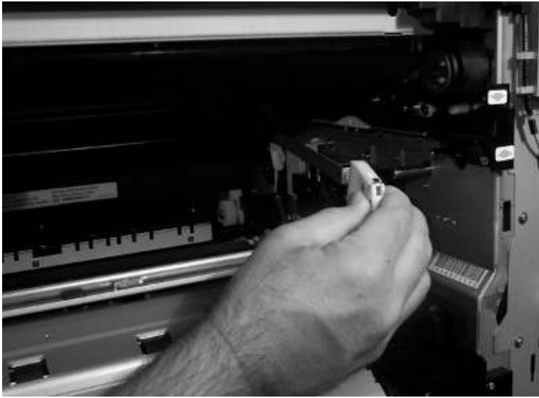
Figure 206. Remove the right back ITB lifting link
