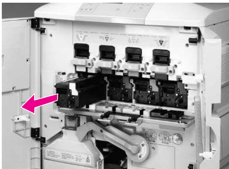
Figure 76. Remove the process cartridges
