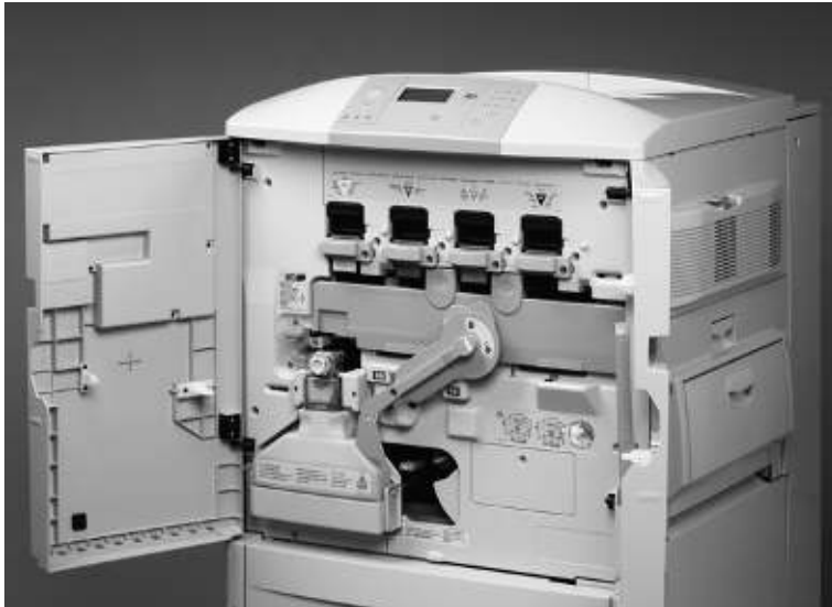
Figure 70. Gain access to the toner cartridges
