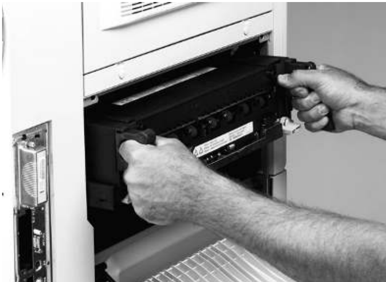
Figure 158. Remove the fuser
