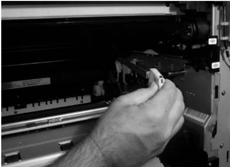
Figure 218. Remove the right back ITB lift link (2 of 2)
