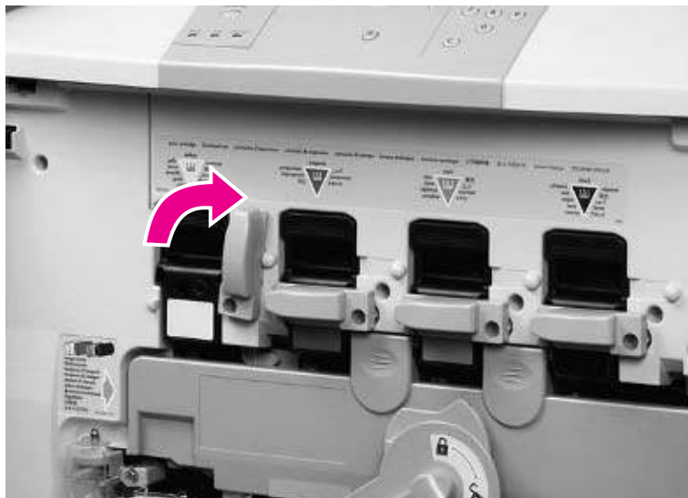
Figure 71. Rotate the toner cartridge lever
