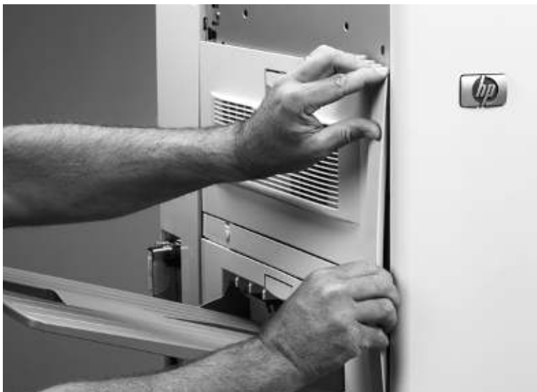
Figure 141. Remove the left side front cover
