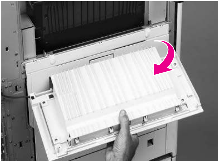
Figure 149. Remove the paper path access door
