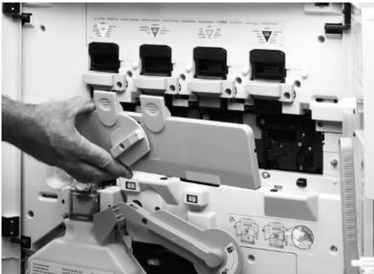
Figure 117. Remove the process cartridge door
