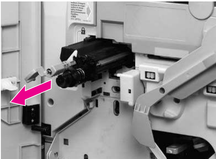
Figure 79. Remove the transfer cleaner
