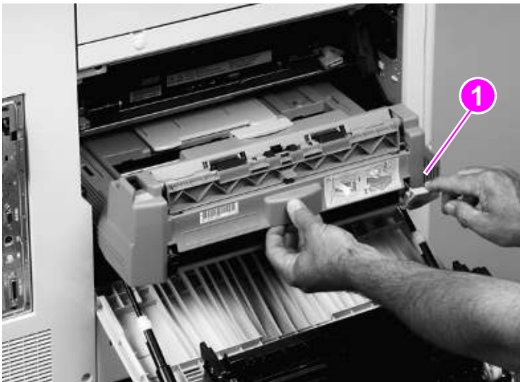
Figure 156. Remove the duplexer
