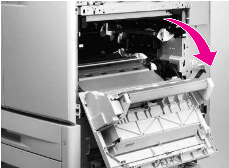
Figure 103. Open the ITB door
