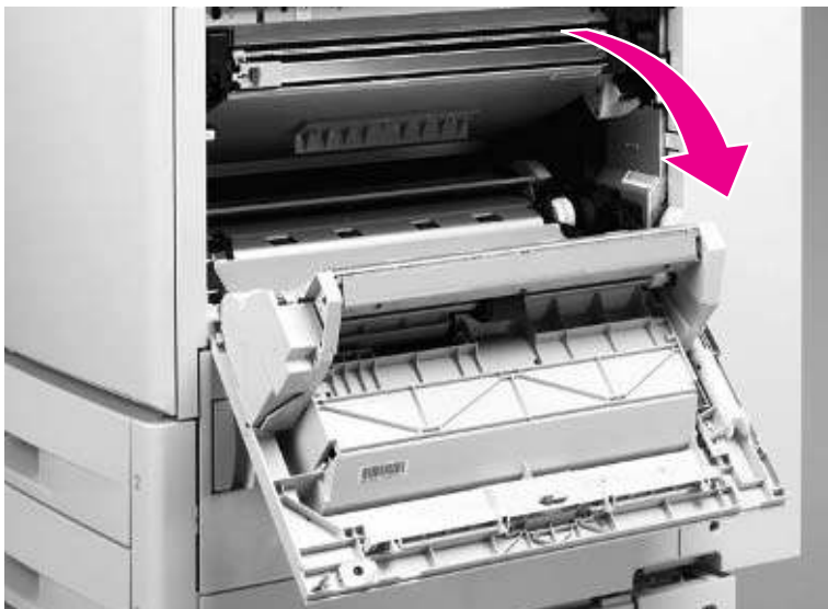
Figure 160. Open the ITB door
