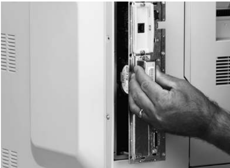
Figure 230. Remove the formatter PCB
