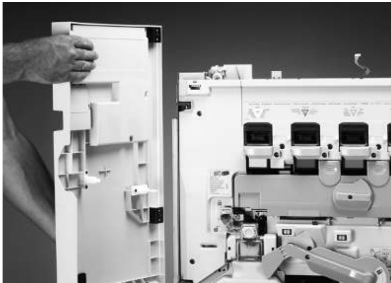
Figure 97. Remove the front doors
