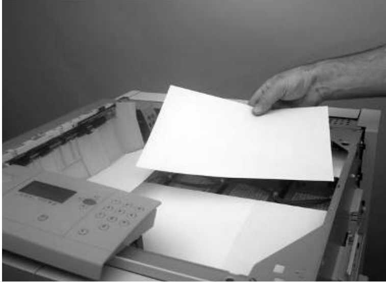
Figure 121. Cover the laser/scanners to prevent a light leak
