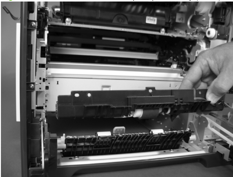
Figure 6-230 Remove the cassette-pickup assembly (3 of 3)
