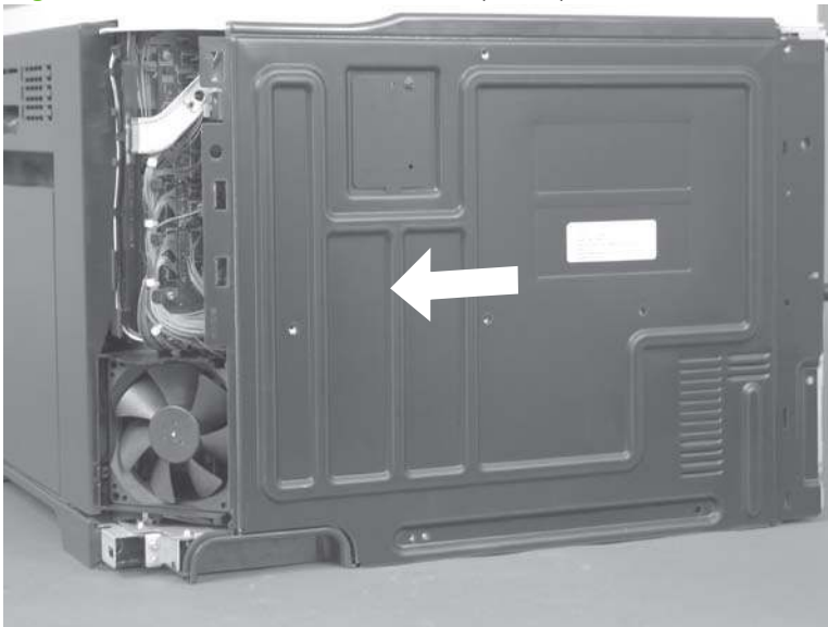
Figure 6-90 Remove the rear cover (2 of 2)
