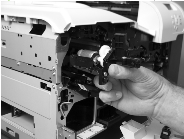
Figure 6-185 Remove the residual-toner-feed motor (7 of 7)
