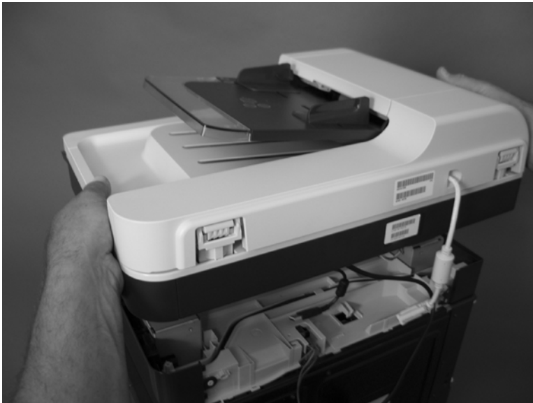
Figure 6-102 Remove the scanner assembly (6 of 6)
