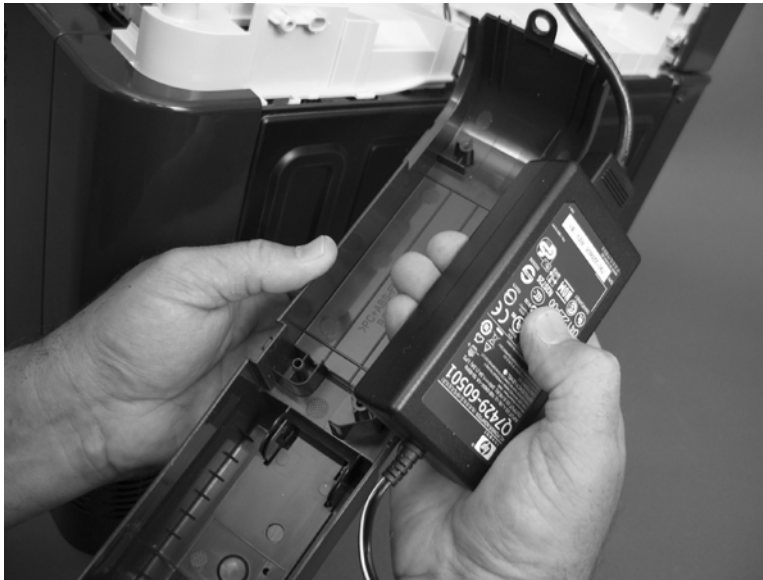
Figure 6-120 Remove the front stapler cover and right-side stapler cover (13 of 13)
