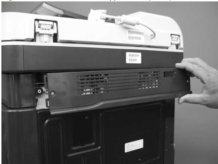
Figure 6-88 Remove the rear-upper cover (4 of 4)
