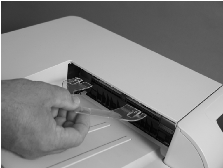
Figure 6-9 Remove the duplex-reverse guide (2 of 2)
