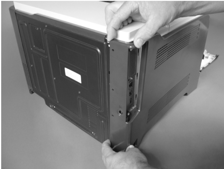
Figure 6-81 Remove the left cover (2 of 5)
