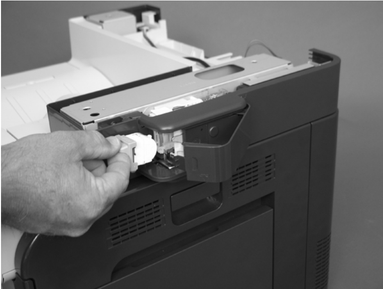
Figure 6-7 Remove the stapler cartridge
