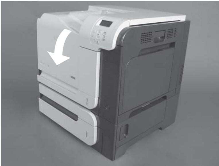
Figure 6-44 Remove the front-door assembly (1 of 2)
