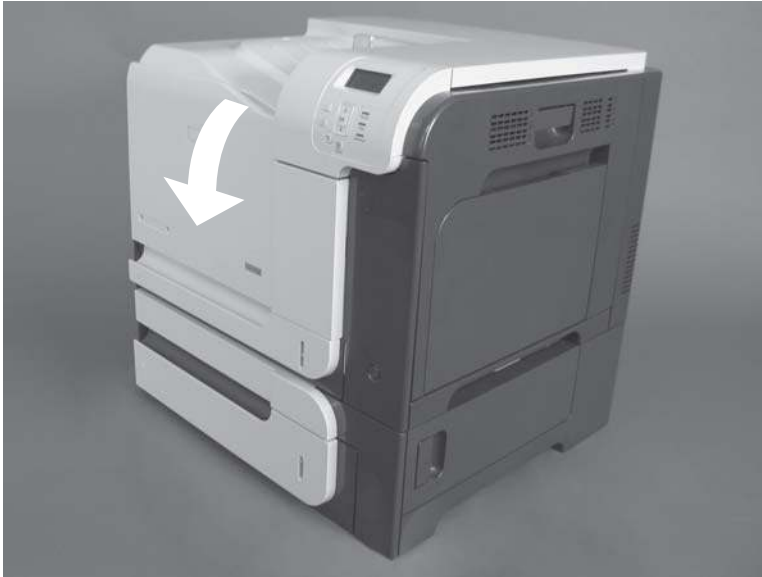
Figure 6-10 Remove the toner-collection unit (1 of 4)
