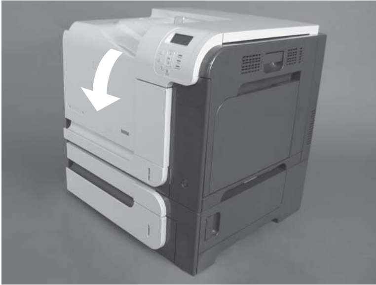
Figure 6-5 Remove the print cartridge (1 of 2)
