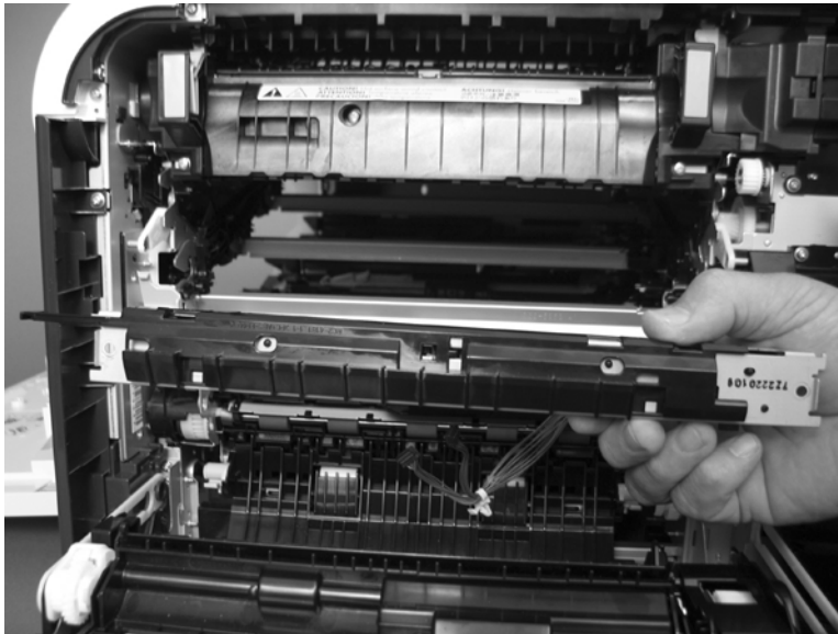
Figure 6-192 Remove the RD sensor assembly (6 of 6)
