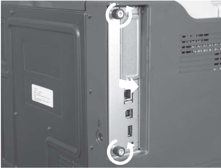
Figure 6-14 Remove the formatter
