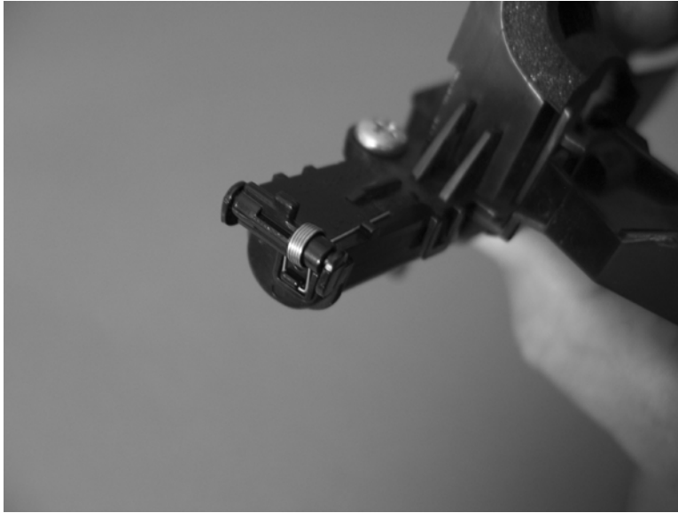
Figure 6-186 Reinstall the residual-toner collection door
