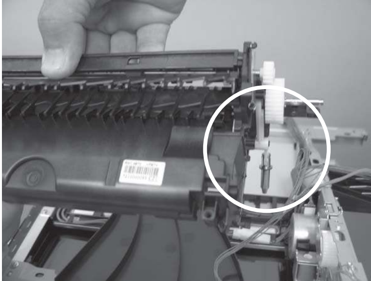
Figure 6-294 Reinstall the delivery assembly (1 of 2)
