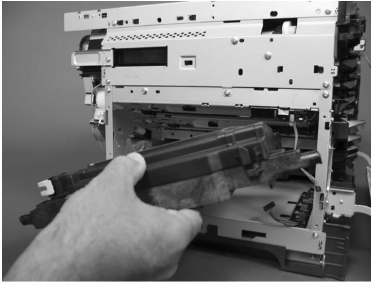
Figure 6-242 Remove the laser/scanner assembly (Y/M) (12 of 12)
