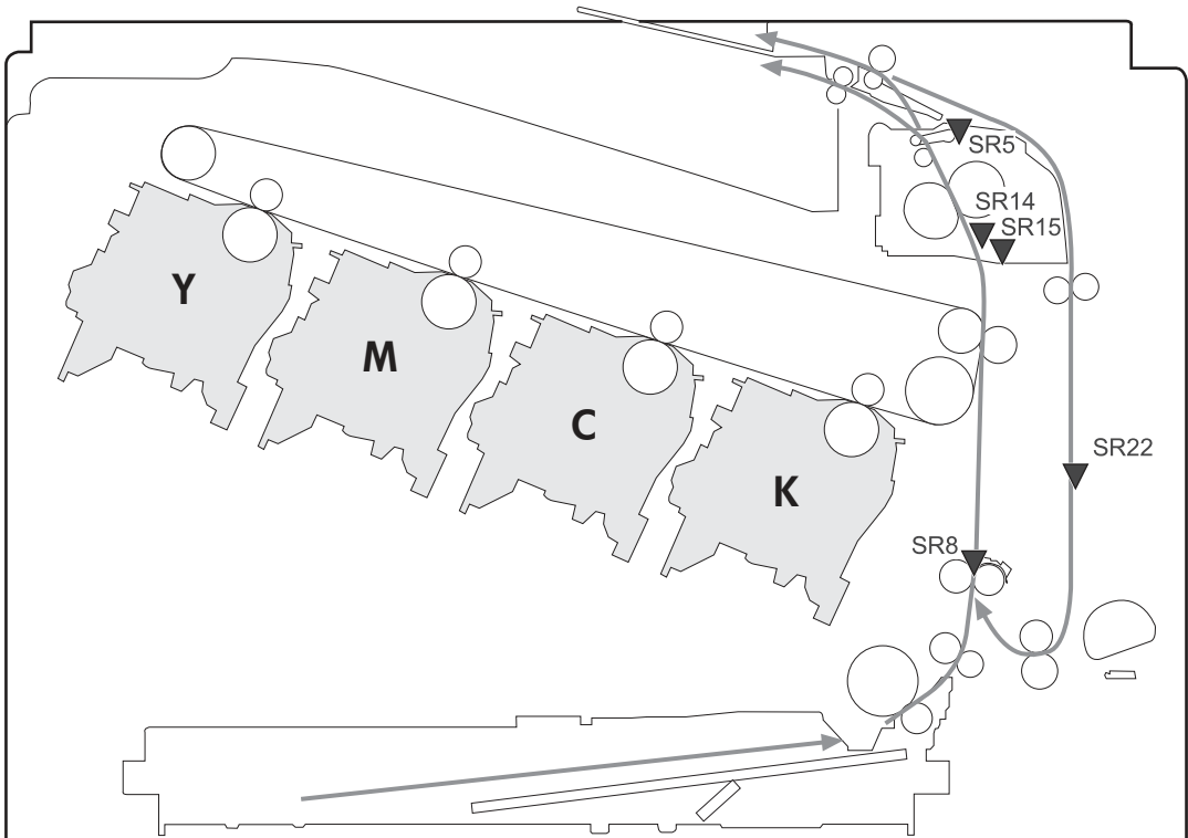
Figure 5-43 Jam detection sensors
