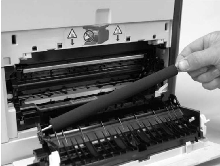
Figure 6-9 Remove the transfer roller (3 of 3)
