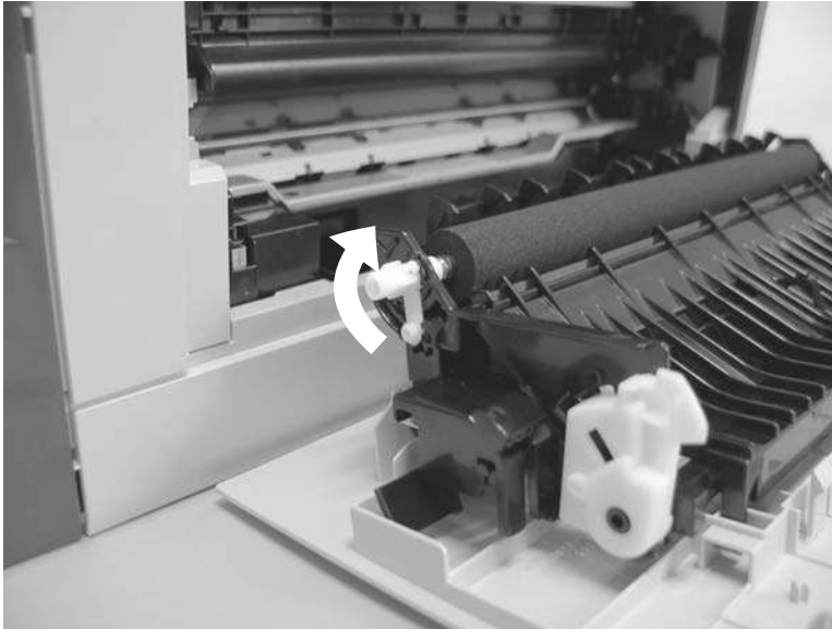
Figure 6-7 Remove the transfer roller (1 of 3)
