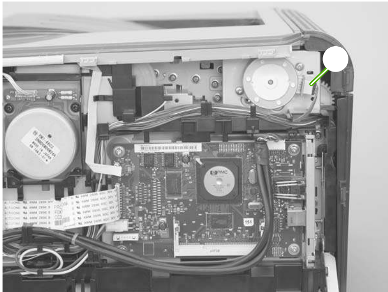
Figure 6-46 Remove the fuser motor (1 of 2)
