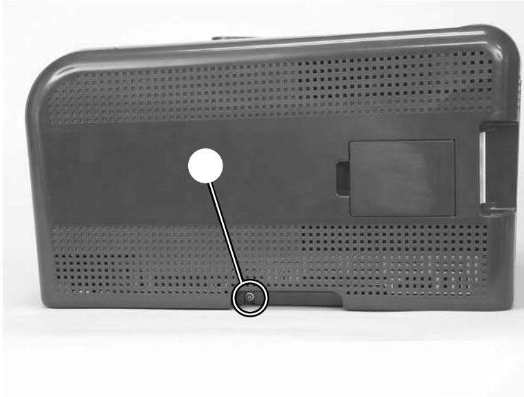
Figure 6-12 Remove the right cover (1 of 4)
