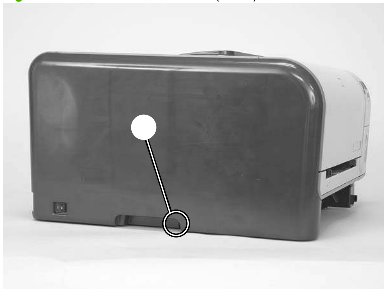
Figure 6-16 Remove the left cover (1 of 4)
