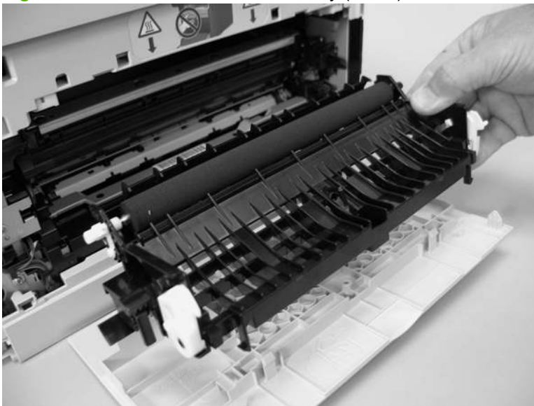
Figure 6-11 Remove the feed assembly (2 of 2)
