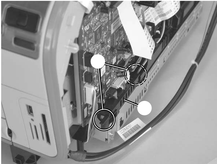
Figure 6-72 Remove the power supply (low-voltage; 3 of 10)
