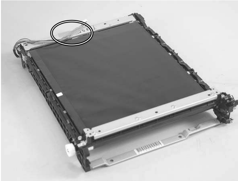
Figure 6-58 Reinstall the ITB (2 of 2)
