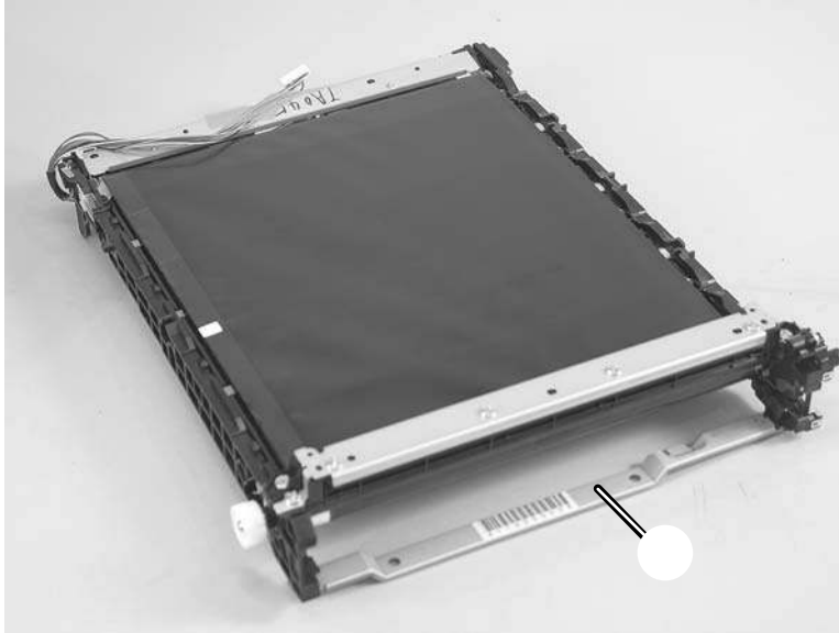
Figure 6-57 Reinstall the ITB (1 of 2)
