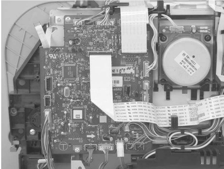
Figure 6-60 Remove the DC controller PCA (2 of 3)
