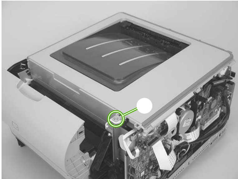
Figure 6-40 Remove the top cover (1 of 4)
