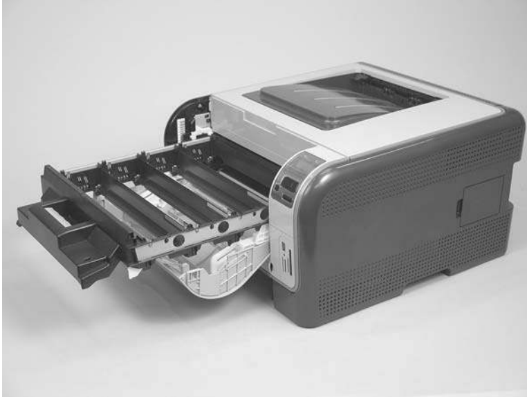
Figure 6-48 Remove the ITB (1 of 9)
