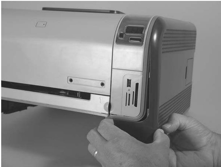
Figure 6-13 Remove the right cover (2 of 4)
