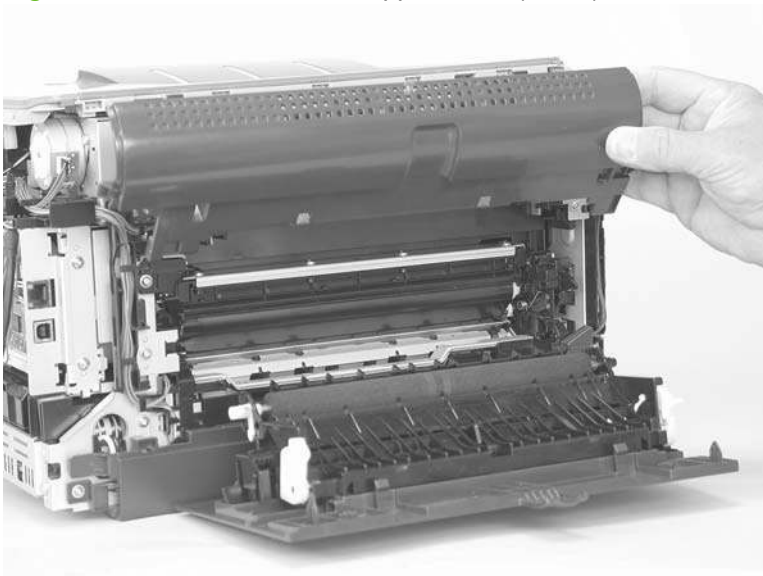
Figure 6-35 Remove the rear-upper cover (2 of 2)
