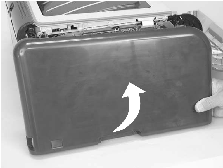
Figure 6-19 Remove the left cover (4 of 4)
