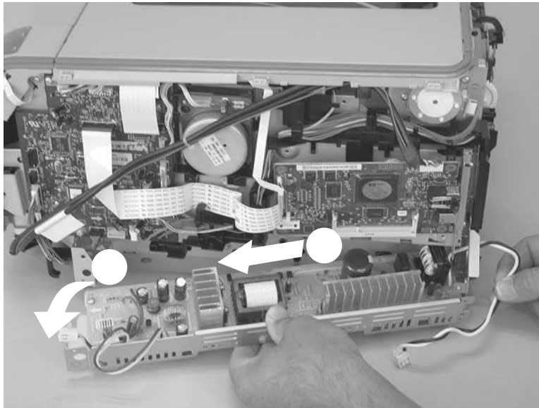
Figure 6-79 Remove the power supply (low-voltage; 10 of 10)
