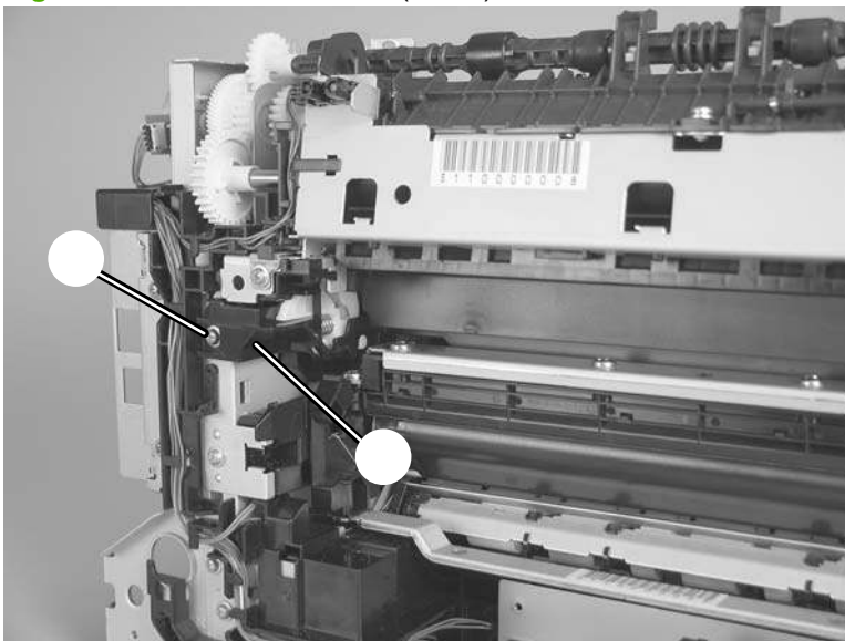
Figure 6-53 Remove the ITB (6 of 9)
