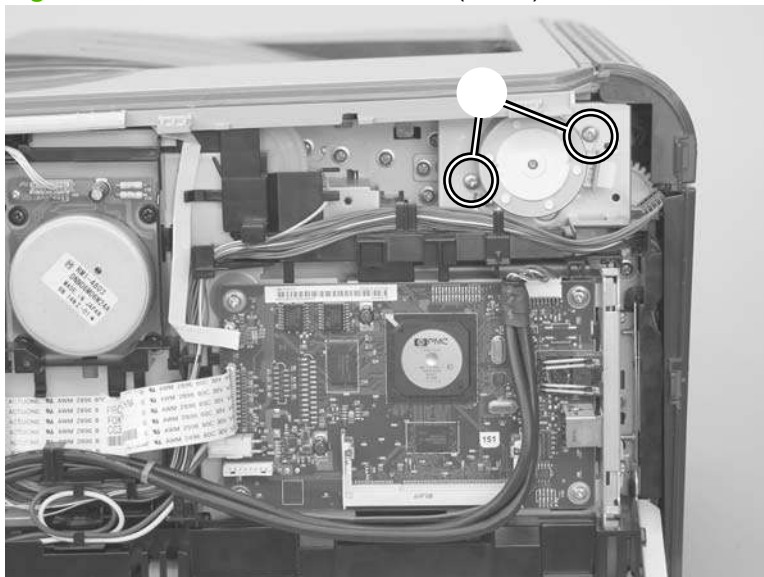
Figure 6-47 Remove the fuser motor (2 of 2)
