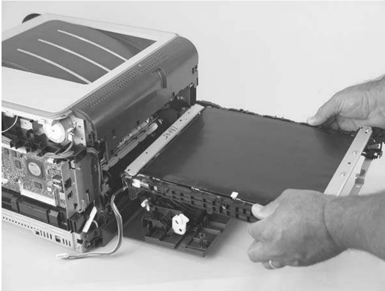
Figure 6-56 Remove the ITB (9 of 9)
