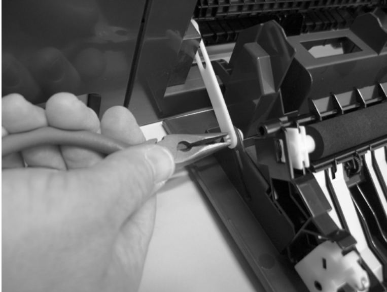
Figure 6-32 Remove the rear door (simplex product) (1 of 4)
