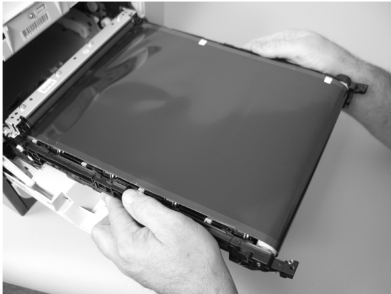
Figure 6-26 Remove the ITB (6 of 6)
