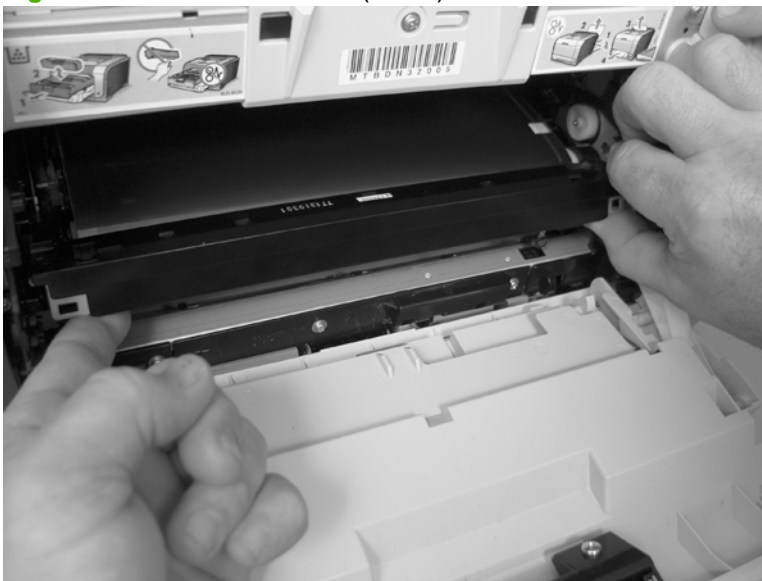
Figure 6-24 Remove the ITB (4 of 6)
