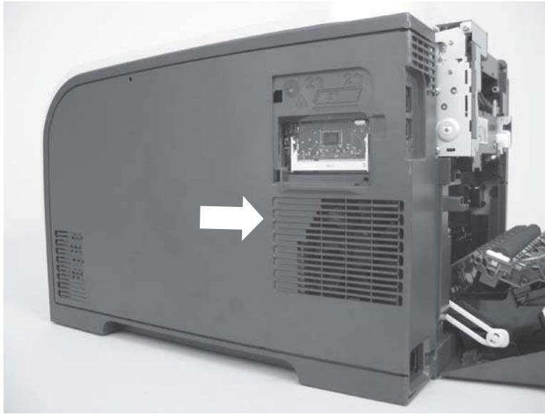
Figure 6-42 Remove the right cover (3 of 5)
