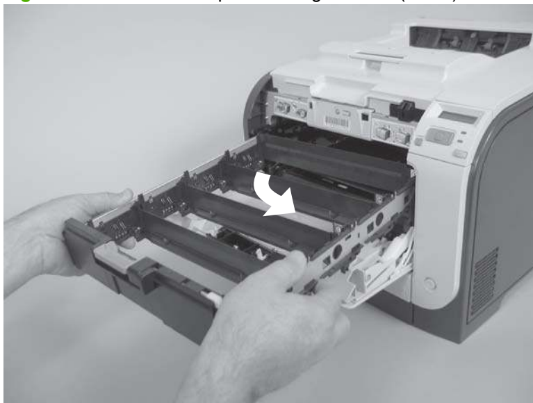
Figure 6-19 Remove the print-cartridge drawer (2 of 3)
