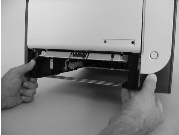
Figure 6-4 Remove the pickup roller (1 of 2)
