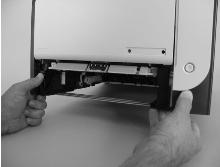
Figure 6-11 Remove the Tray 1 paper-pickup roller (2 of 3)
