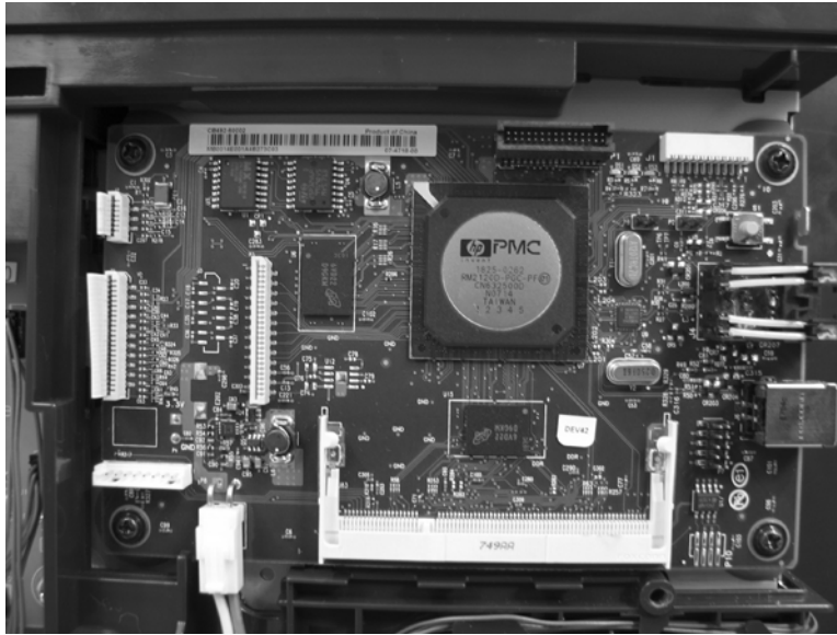
Figure 6-102 Remove the formatter PCA (1 of 2)
