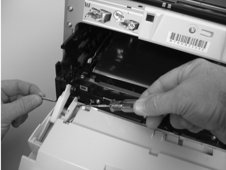
Figure 6-143 Remove the front-door assembly (2 of 10)
