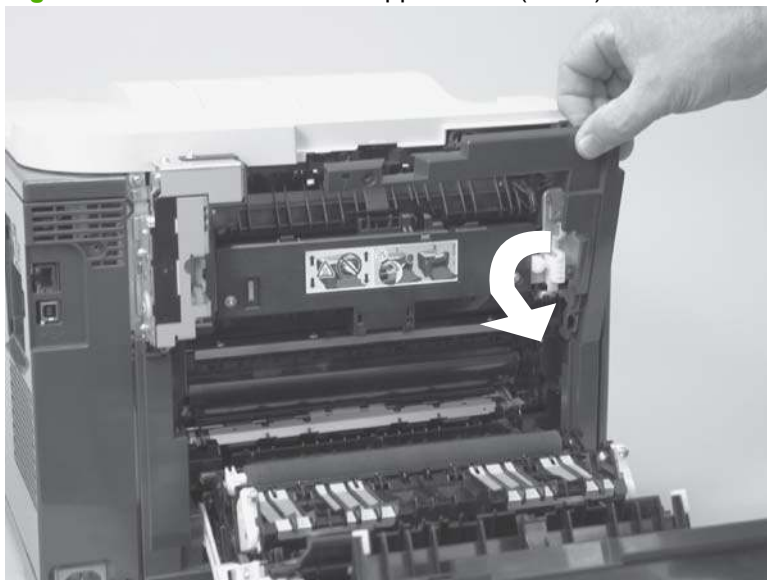
Figure 6-47 Remove the rear-upper cover (2 of 2)
