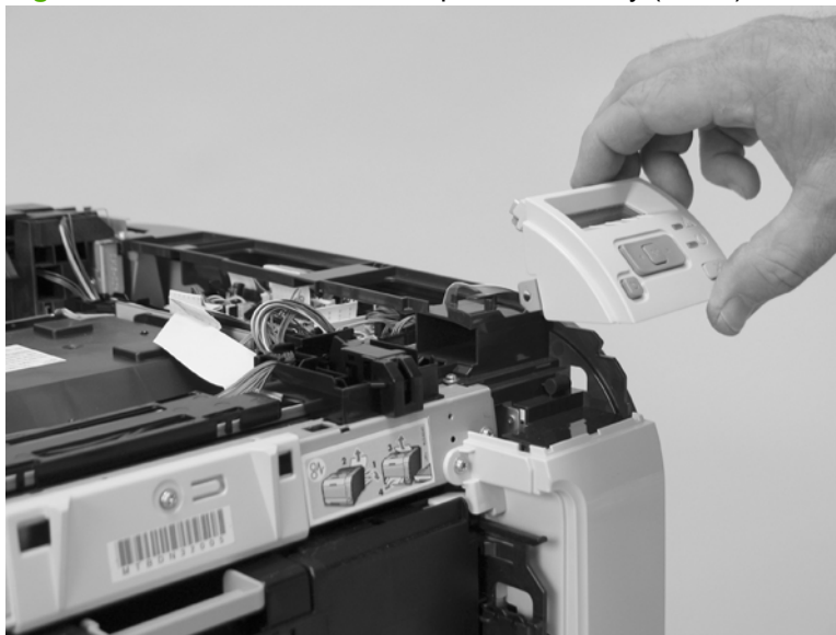
Figure 6-71 Remove the control-panel assembly (3 of 3)
