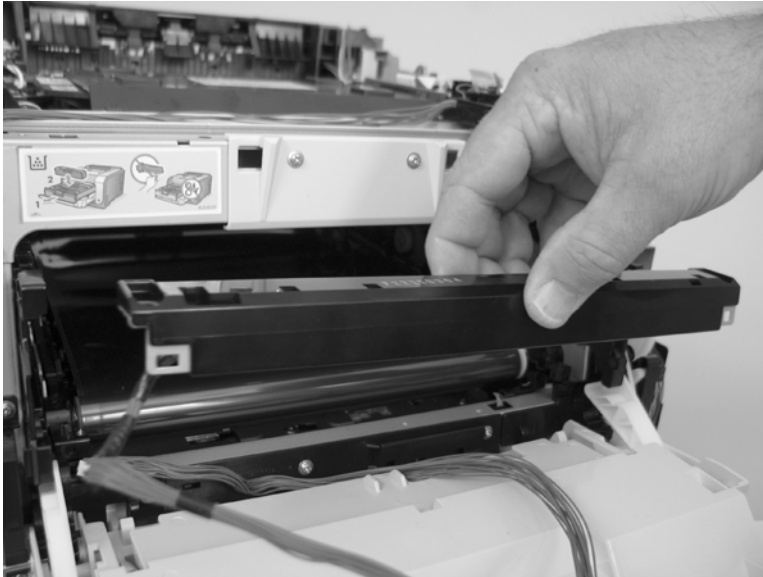
Figure 6-86 Remove the color-misregistration sensor assembly PCA (5 of 5)
