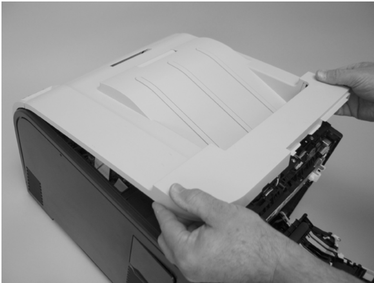
Figure 6-66 Remove the upper-cover assembly (4 of 4)
