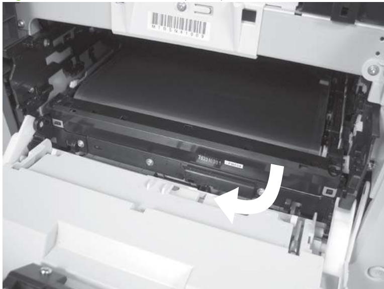
Figure 6-22 Remove the ITB (2 of 6)
