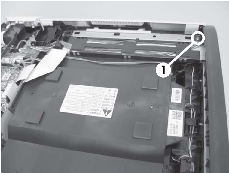
Figure 6-72 Remove the left cover (1 of 3)
