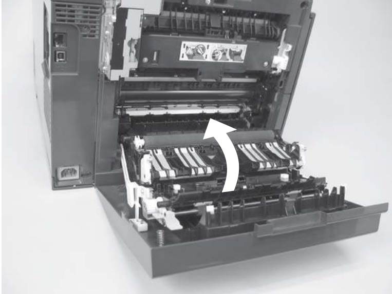
Figure 6-36 Remove the rear door (duplex product) (1 of 4)
