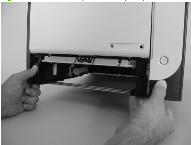
Figure 6-6 Remove the separation roller (1 of 3)
