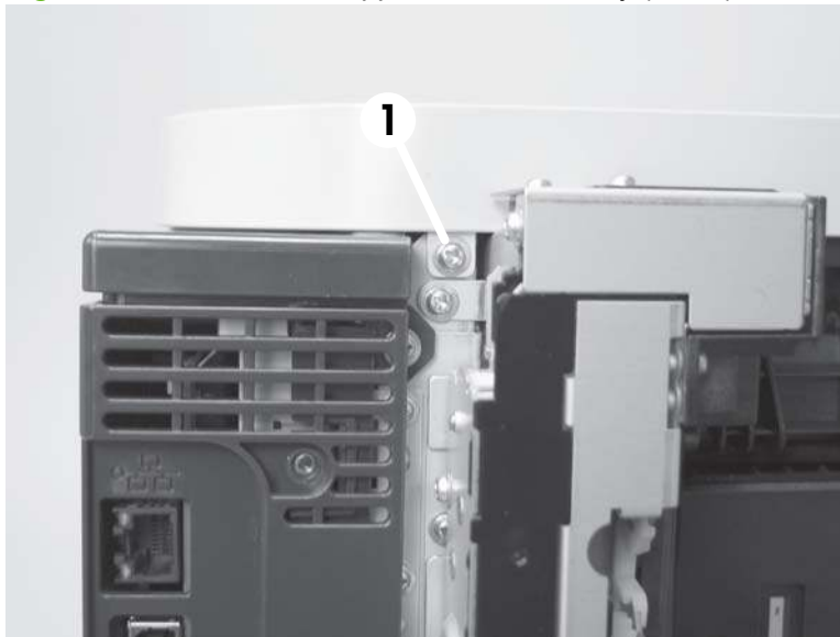
Figure 6-63 Remove the upper-cover assembly (1 of 4)
