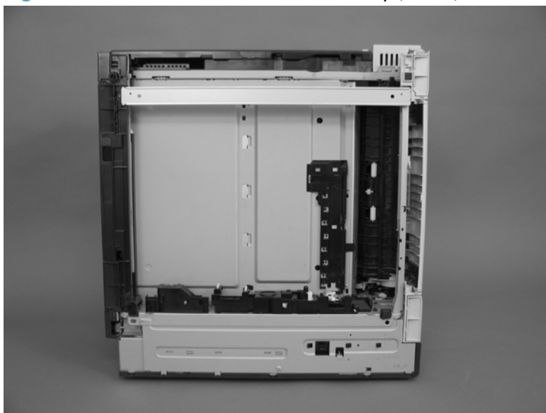
Figure 2-70 Remove the lifter-drive assembly (1 of 3)
