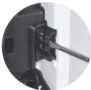
Figure 3-4 Test the front-door opening/closing switch
