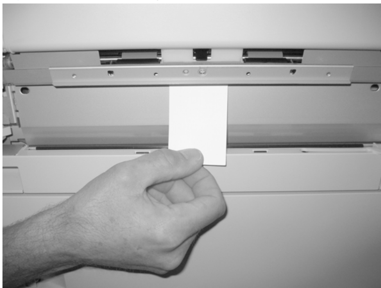
Figure 3-21 Test the Tray 3 feed sensor
