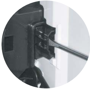
Figure 4 Test the front-door opening/closing switch
