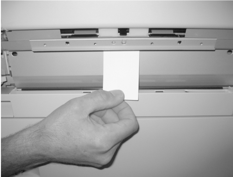
Figure 21 Test the Tray 3 feed sensor
