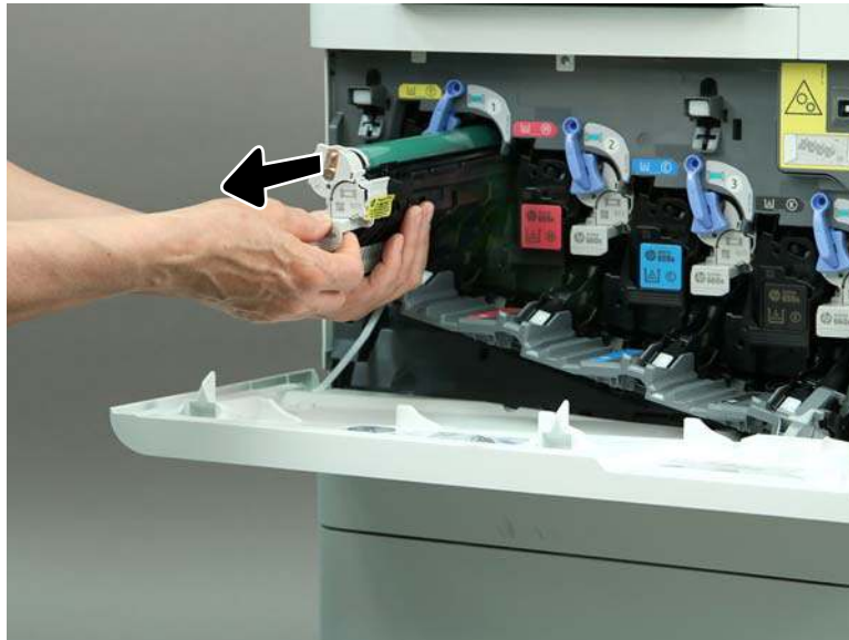
Figure 1-2774 Remove the imaging drum
