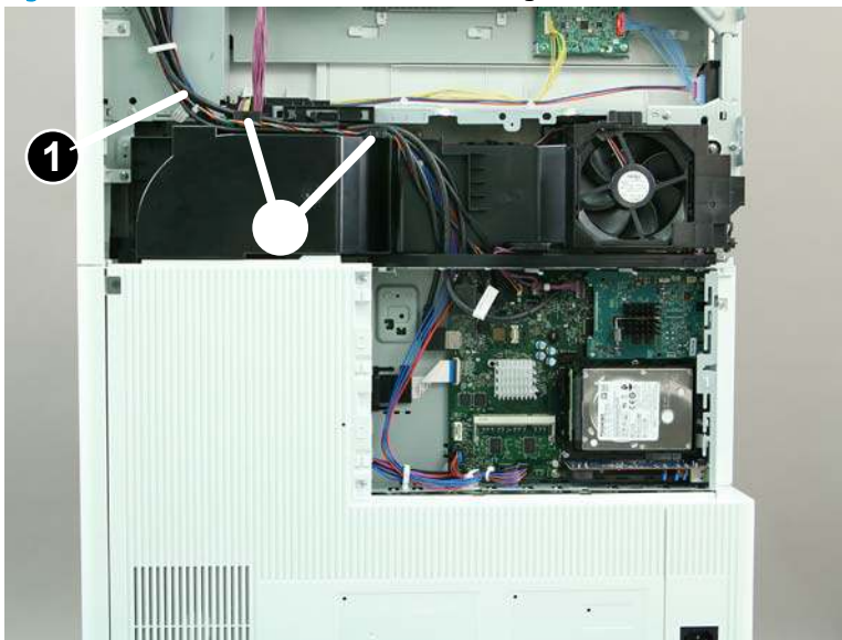
Figure 1-1326 Release the cables from the guides
