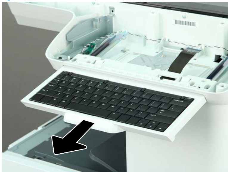
Figure 1-713 Remove the keyboard and rails
