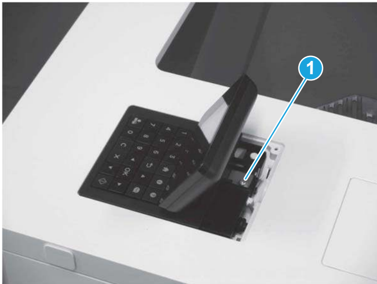
Figure 1-1729 Remove one screw
