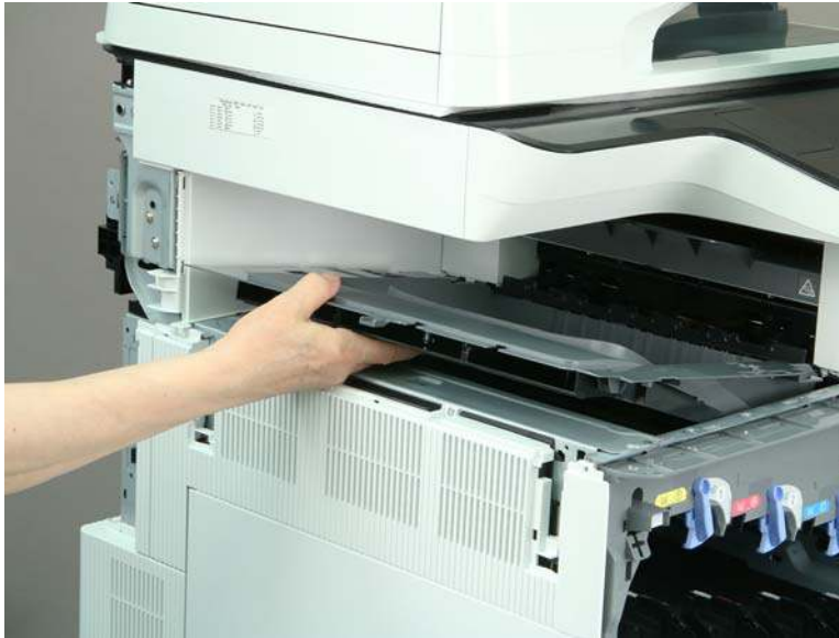
Figure 1-2389 Remove the output bin
