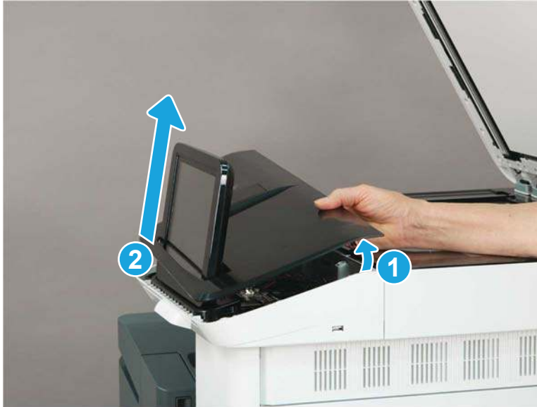
Figure 1-268 Remove the control panel cover
