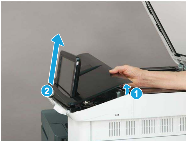
Figure 1-422 Remove the control panel cover
