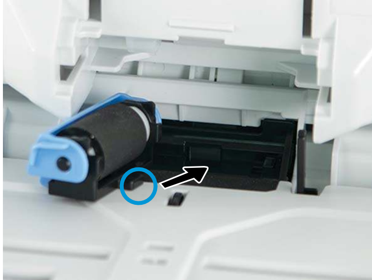
Figure 1-66 Note the tab on the roller
