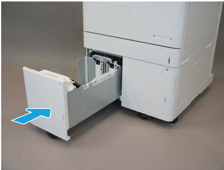
Figure 1-3462 Install the left tray
