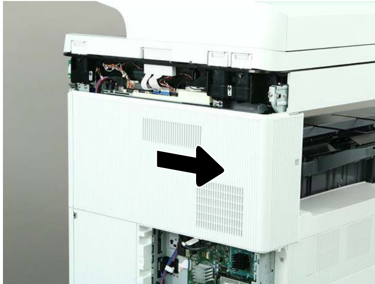
Figure 1-317 Remove the rear upper and left rear upper cover
