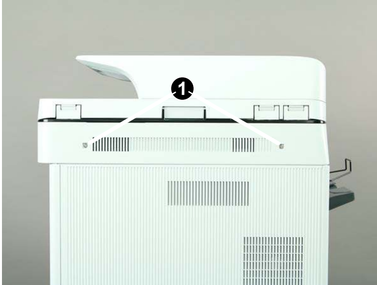
Figure 1-2259 Remove two screws
