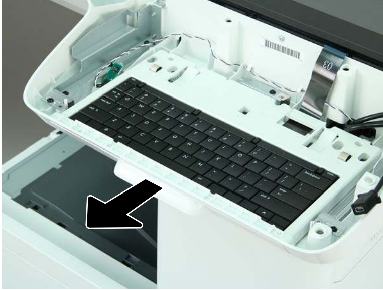
Figure 1-632 Pull the keyboard out
