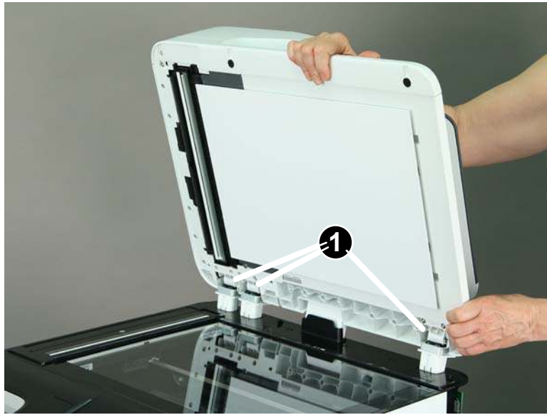
Figure 1-303 Release the hinges
