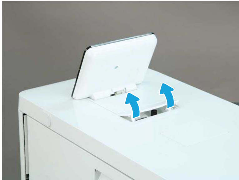
Figure 1-560 Remove the control panel cover
