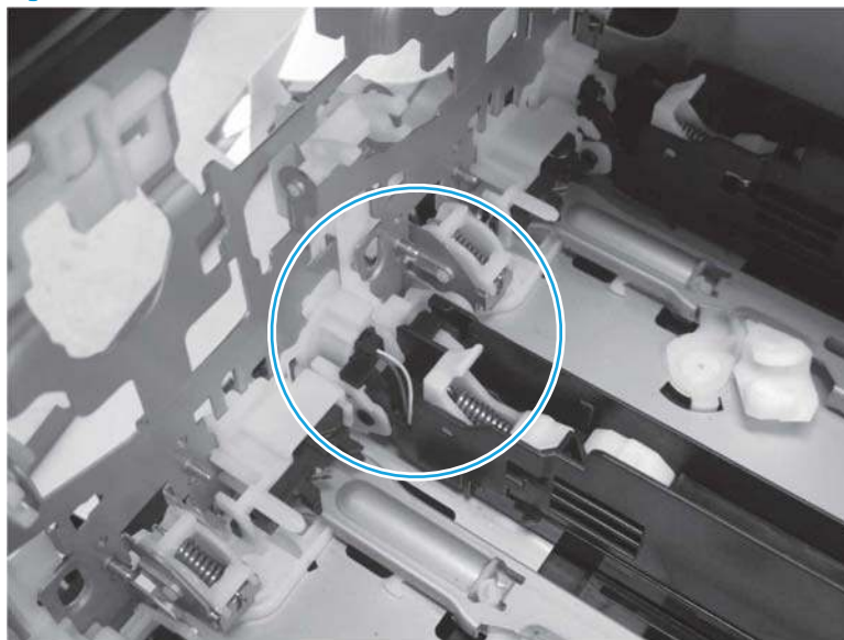
Figure 1-1084 Link arm correct installation (M751/E75245/M856/E85055/M776dn/M776z/M776zs)
