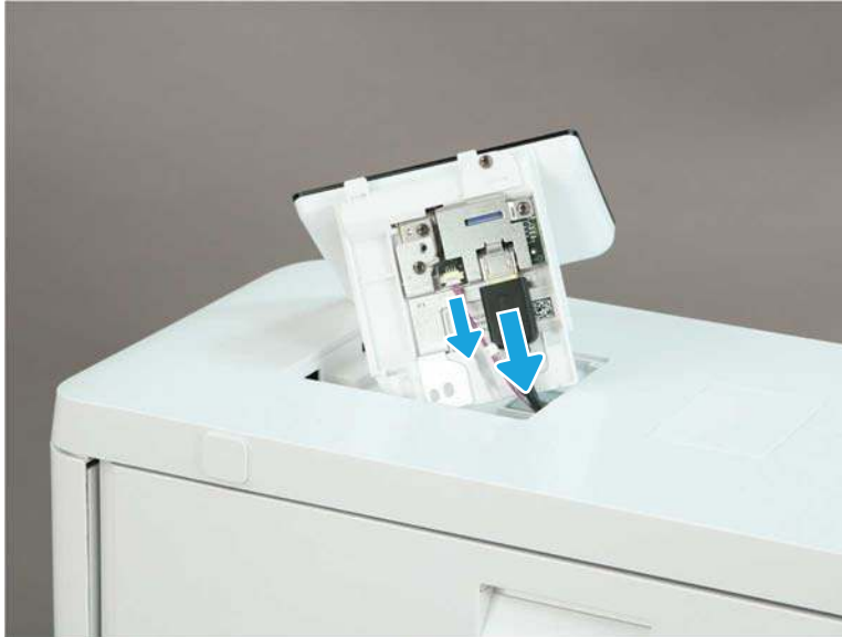
Figure 1-1524 Disconnect two connectors
