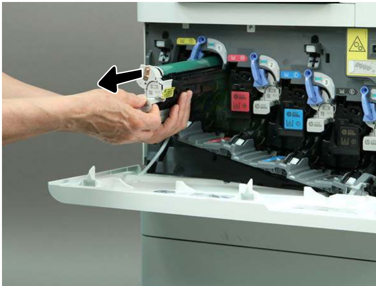
Figure 1-43 Remove the imaging drum
