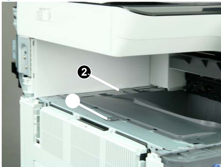
Figure 1-1070 Remove two screws
