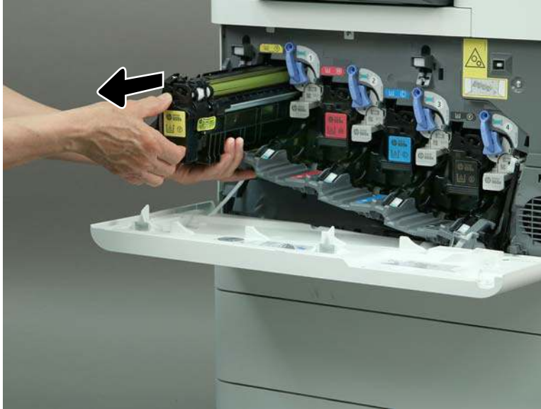
Figure 1-2543 Remove the toner cartridge
