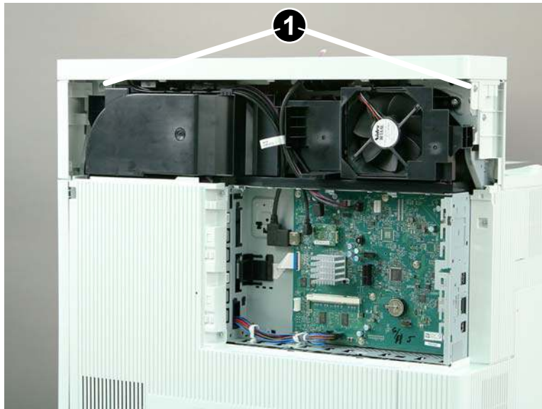
Figure 1-2228 Remove two screws
