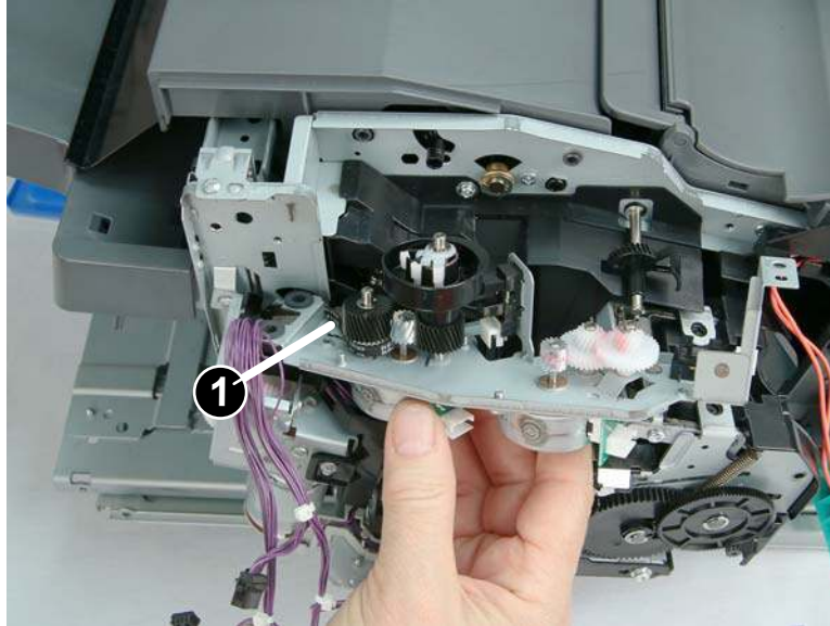
Figure 1-3030 Release the belt and remove the paddle drive assembly
