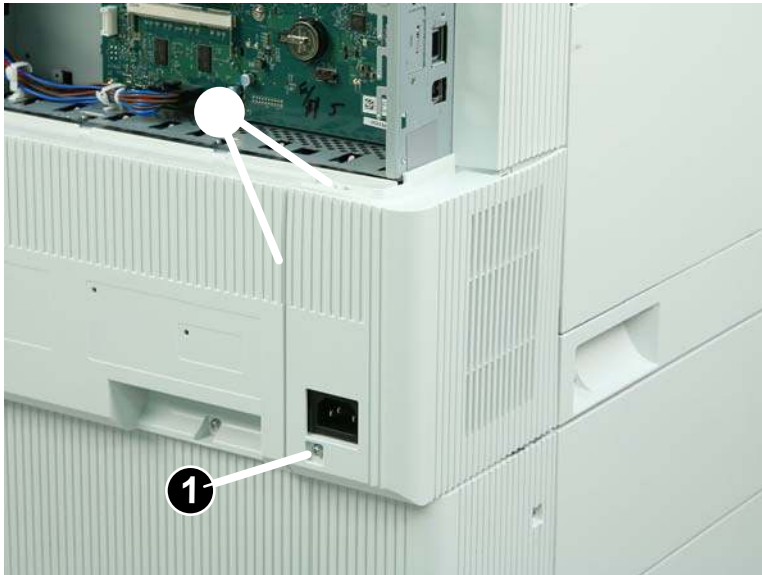
Figure 1-1337 Remove one screw and release two tabs
