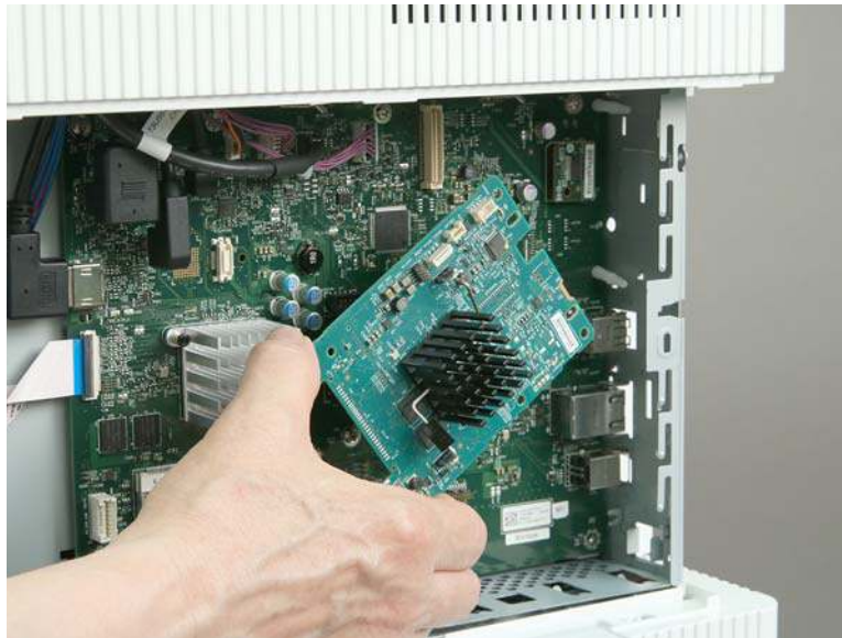
Figure 1-1231 Remove the accelerator board
