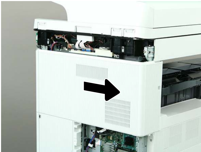
Figure 1-1152 Remove the rear upper and left rear upper cover
