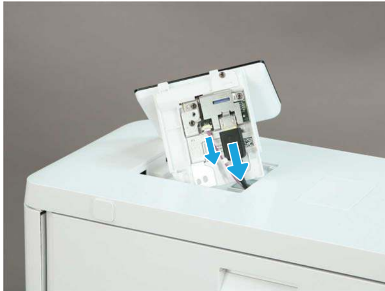
Figure 1-1978 Disconnect two connectors
