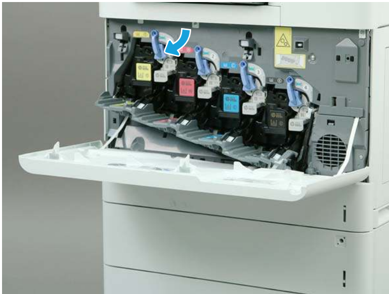
Figure 1-1443 Rotate the blue lever
