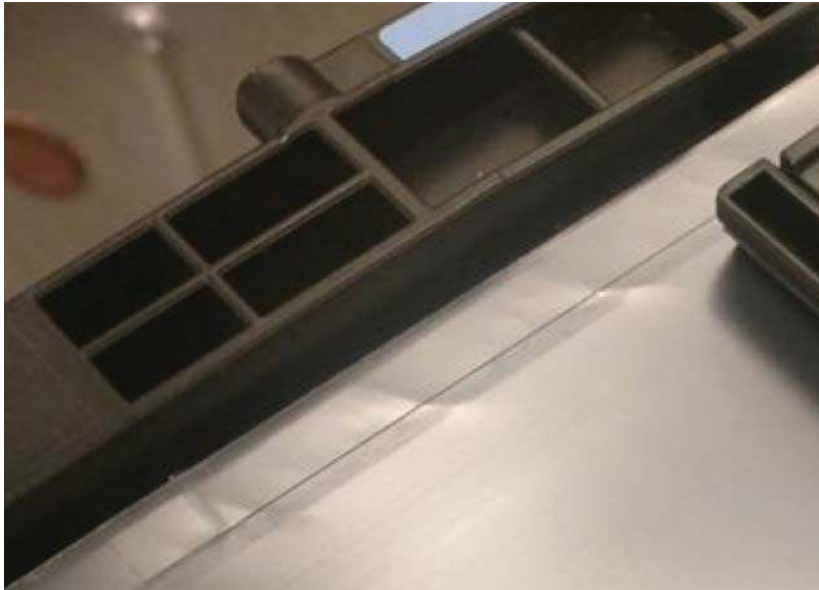
Figure 1-1200 Check for bent or creased edges
