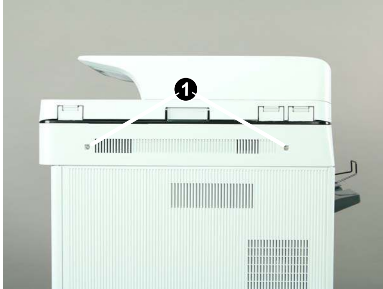
Figure 1-305 Remove two screws
