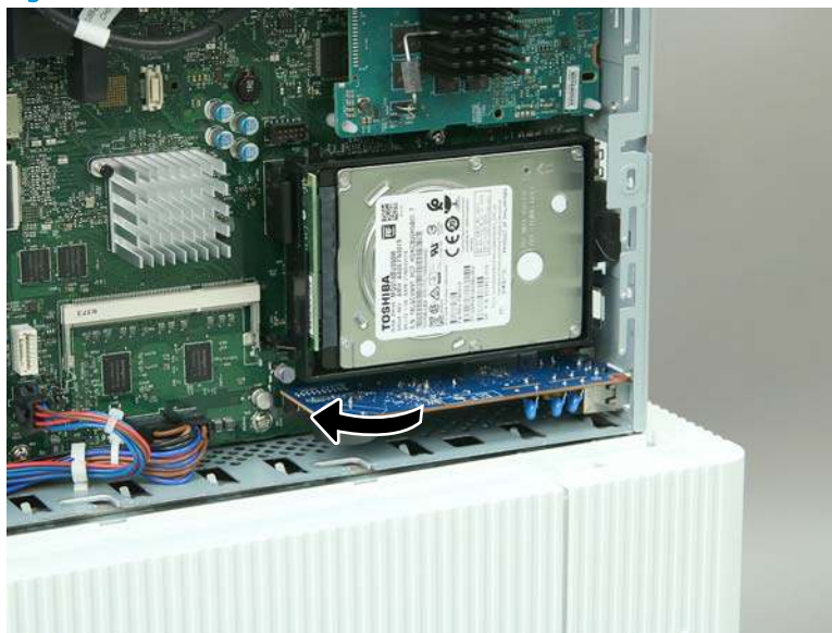
Figure 1-33 Install the fax PCA
