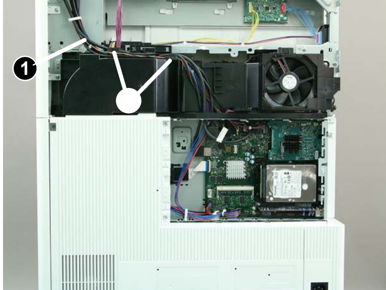
Figure 1-1265 Release the cables from the guides
