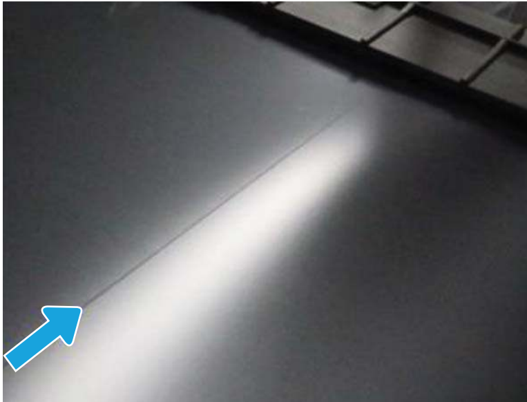
Figure 1-1197 Check for convex streak
