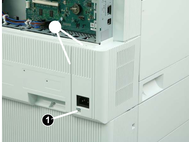
Figure 1-1851 Remove one screw and release two tabs
