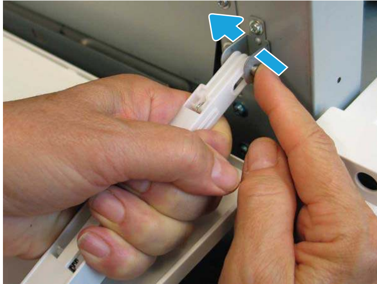
Figure 1-3491 Release the hinge arm
