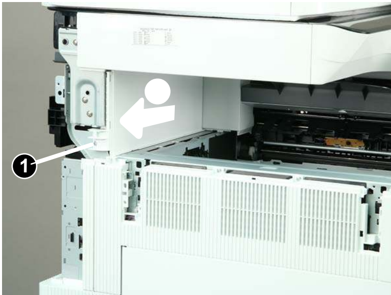
Figure 1-265 Remove the main cover
