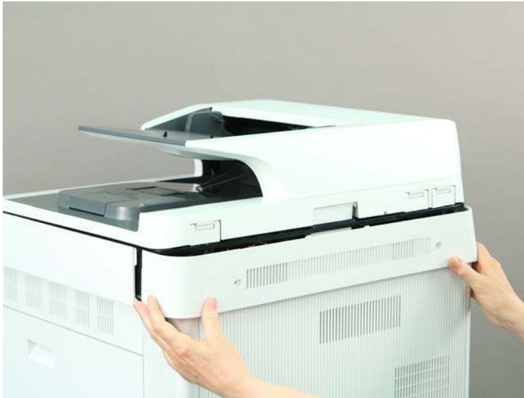
Figure 1-443 Remove the SCB cover
