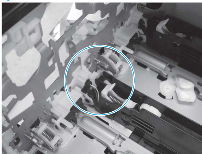
Figure 1-1040 Link arm correct installation (M751/E75245/M856/E85055/M776dn/M776z/M776zs)
