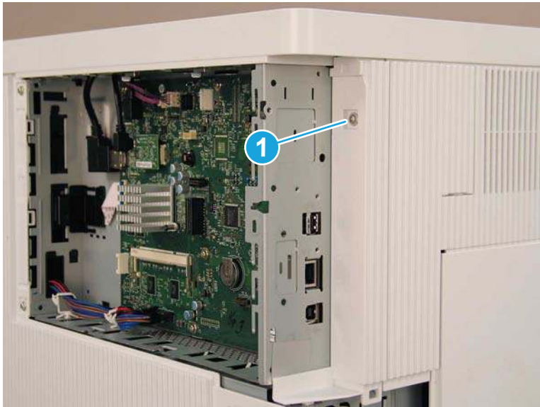
Figure 1-2176 Remove one screw
