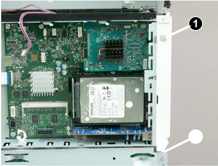
Figure 1-1249 Remove the left rear cover
