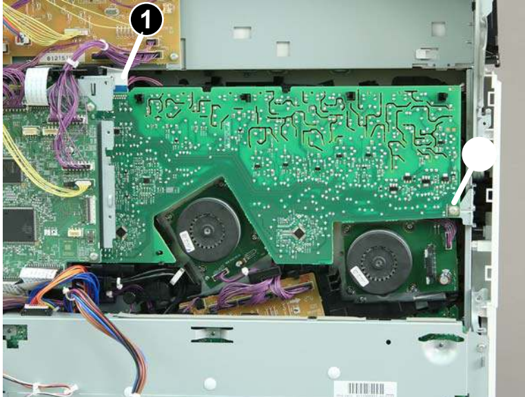
Figure 1-2955 Disconnect one connector and remove one screw
