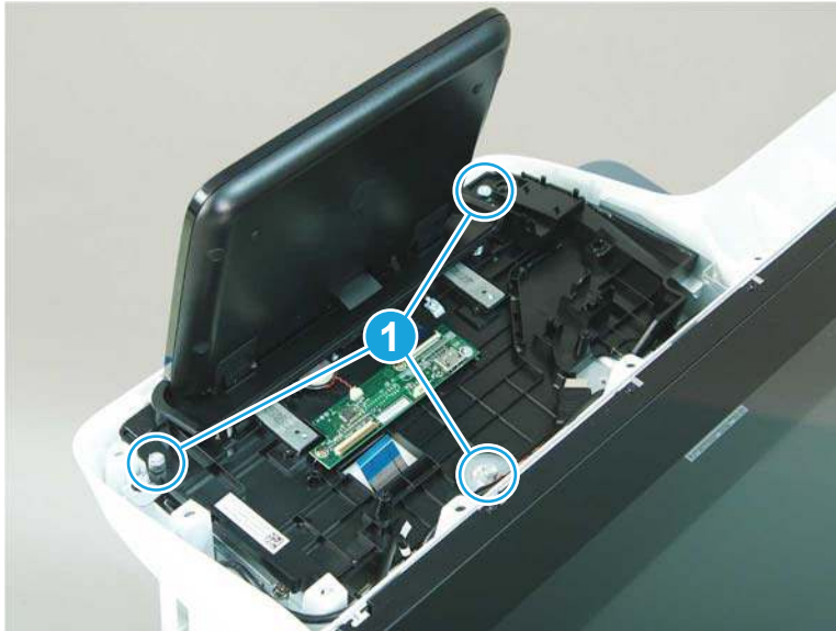
Figure 1-400 Remove three screws
