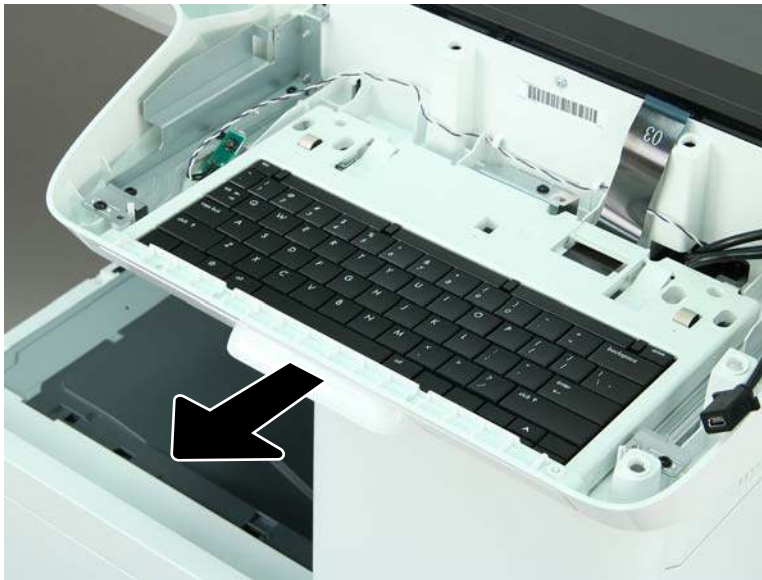
Figure 1-340 Pull the keyboard out
