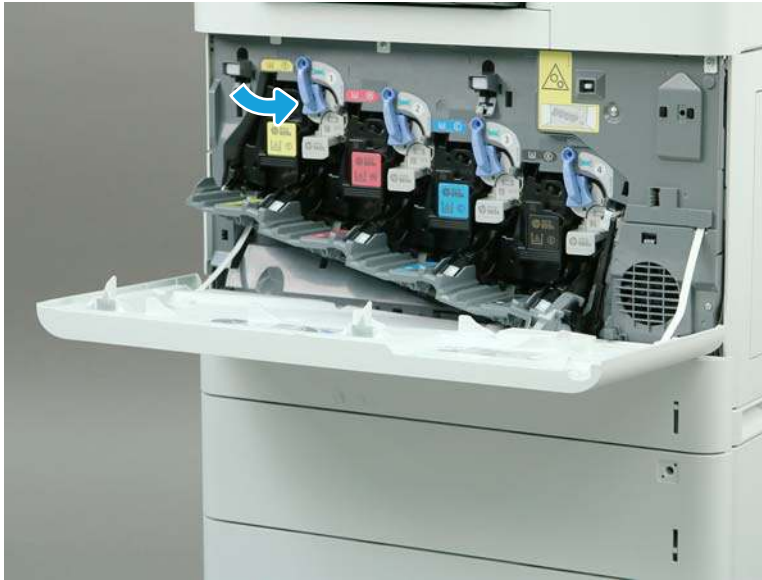
Figure 1-46 Rotate the blue lever
