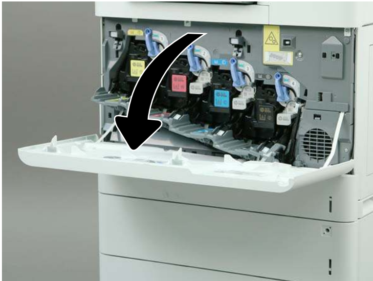
Figure 1-1048 Open the front door
