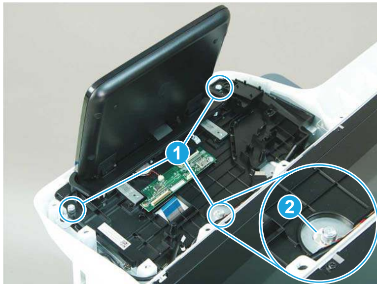
Figure 1-133 Install three screws
