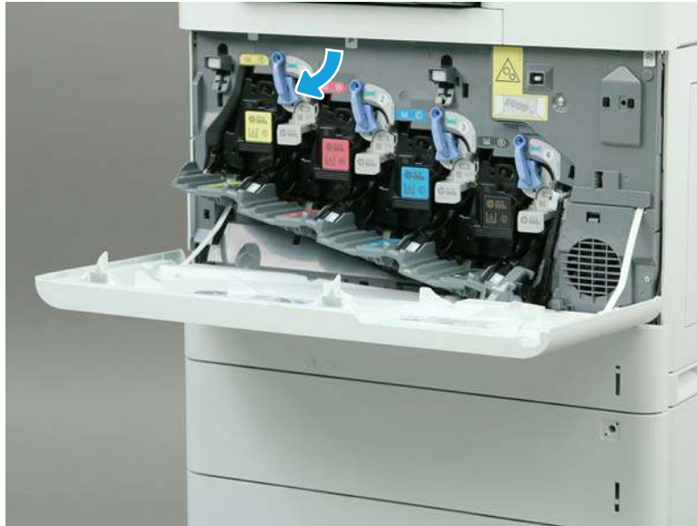
Figure 1-2322 Rotate the blue lever
