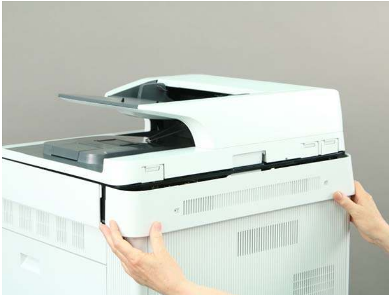
Figure 1-1780 Remove the SCB cover
