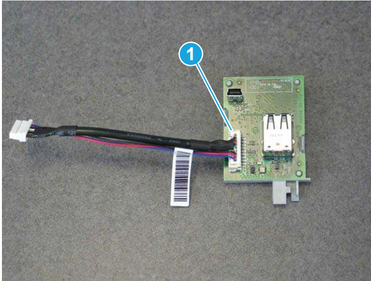
Figure 1-5 Connect the cable to the PCA
