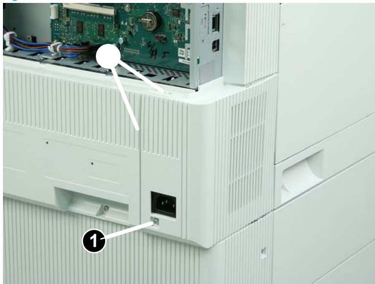
Figure 1-2879 Remove one screw and release two tabs
