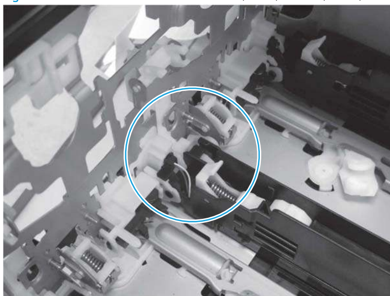
Figure 1-1016 Link arm correct installation (M751/E75245/M856/E85055/M776dn/M776z/M776zs)
