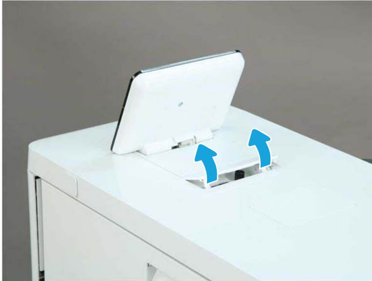
Figure 1-252 Remove the control panel cover
