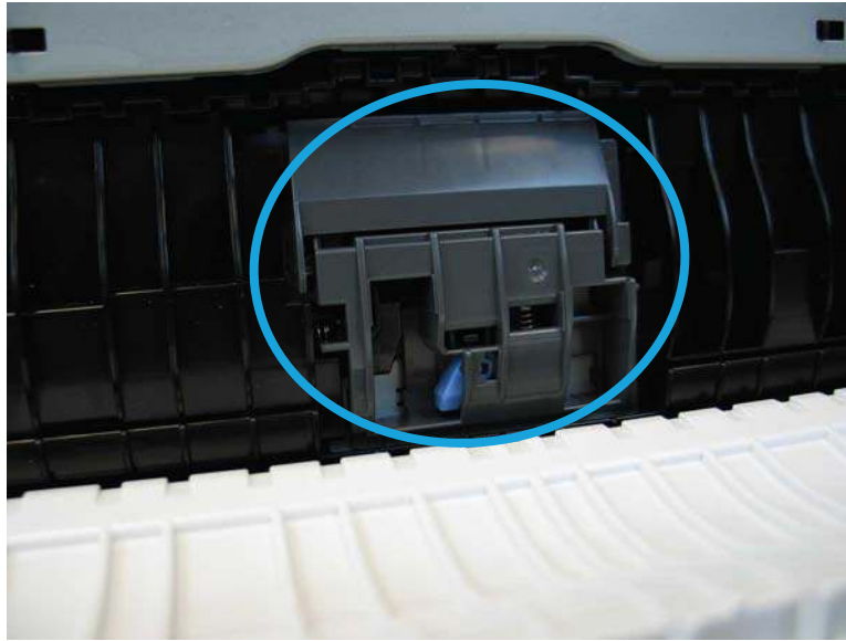
Figure 1-3205 Locate the separation roller
