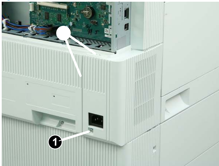
Figure 1-2168 Remove one screw and release two tabs
