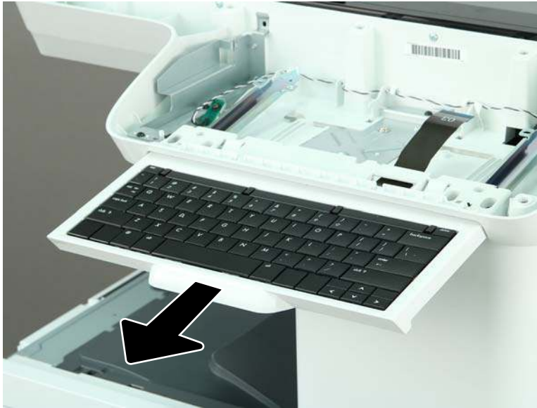
Figure 1-276 Remove the keyboard and rails
