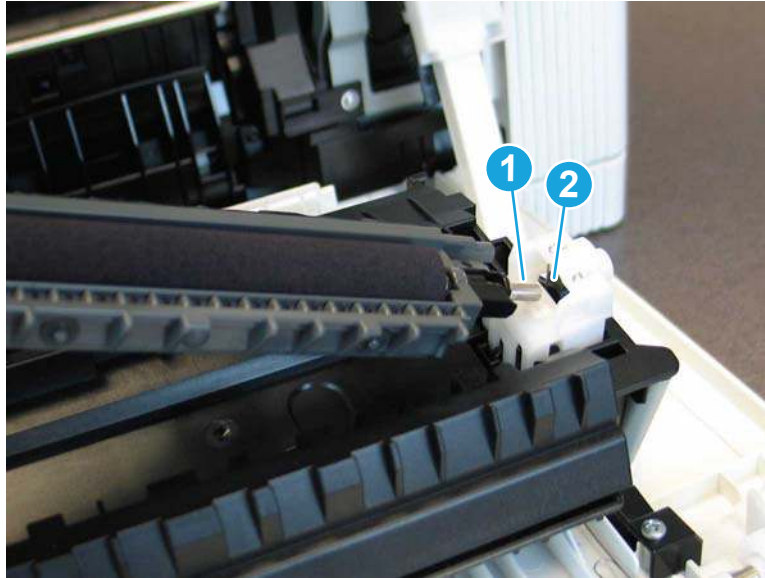
Figure 1-102 Position the secondary transfer roller
