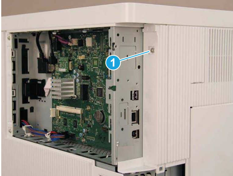
Figure 1-2239 Remove one screw
