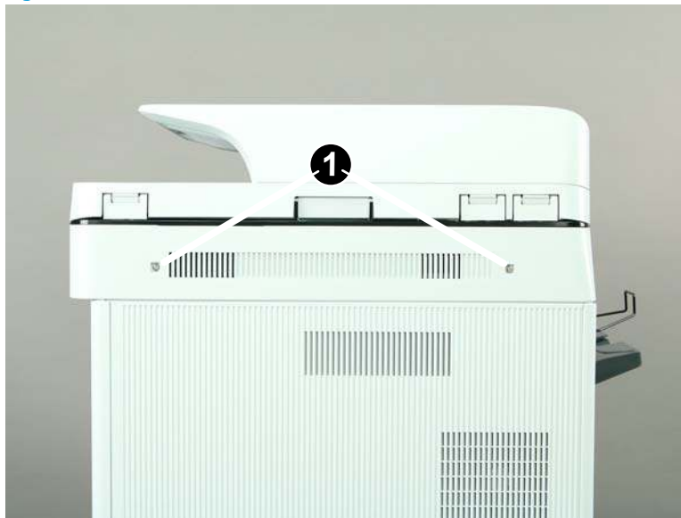
Figure 1-489 Remove two screws
