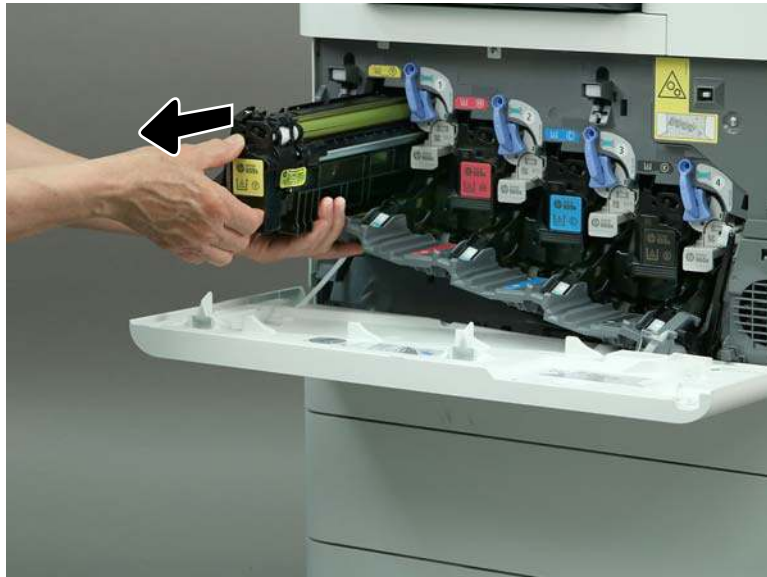
Figure 1-2590 Remove the toner cartridge
