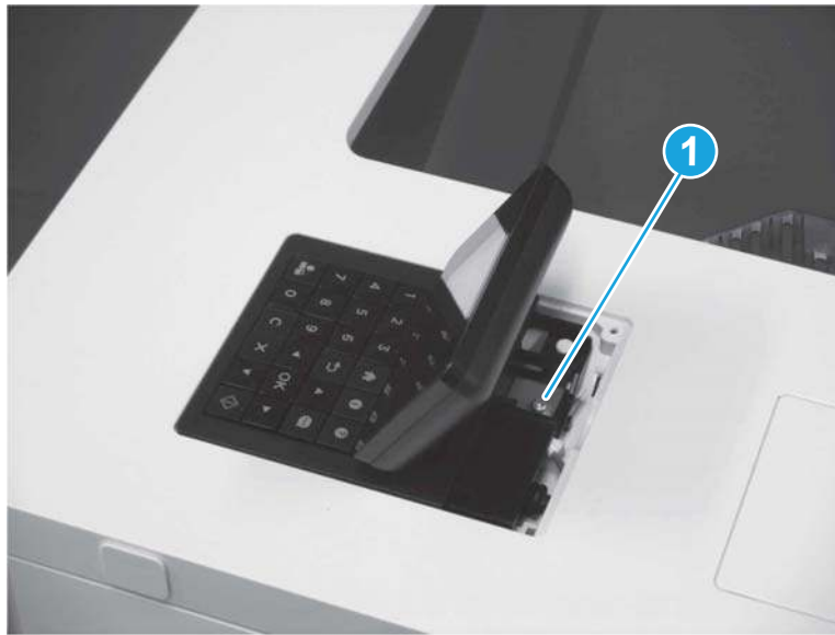
Figure 1-106 Remove one screw
