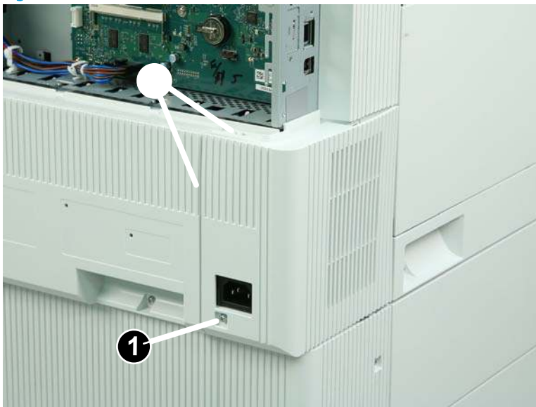
Figure 1-940 Remove one screw and release two tabs
