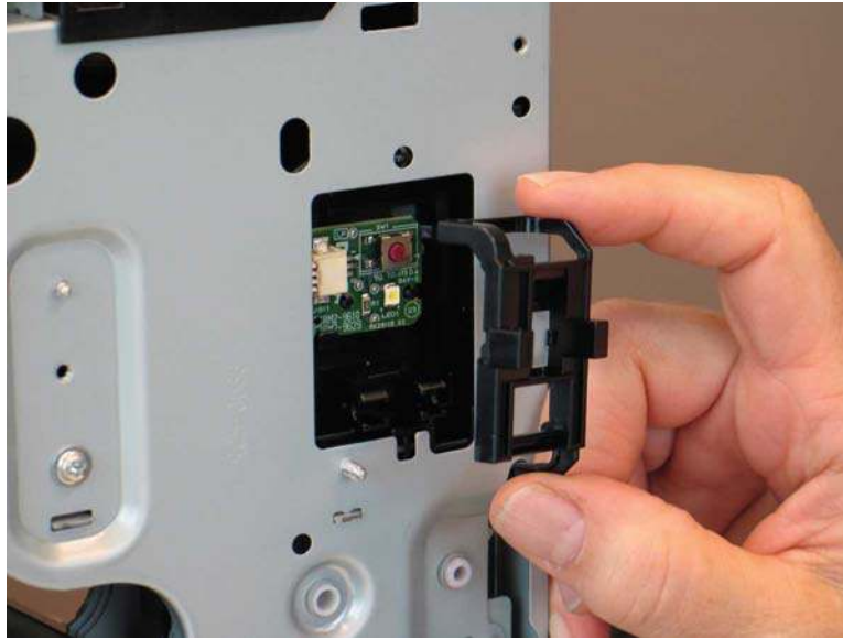
Figure 1-2476 Remove the power switch cover
