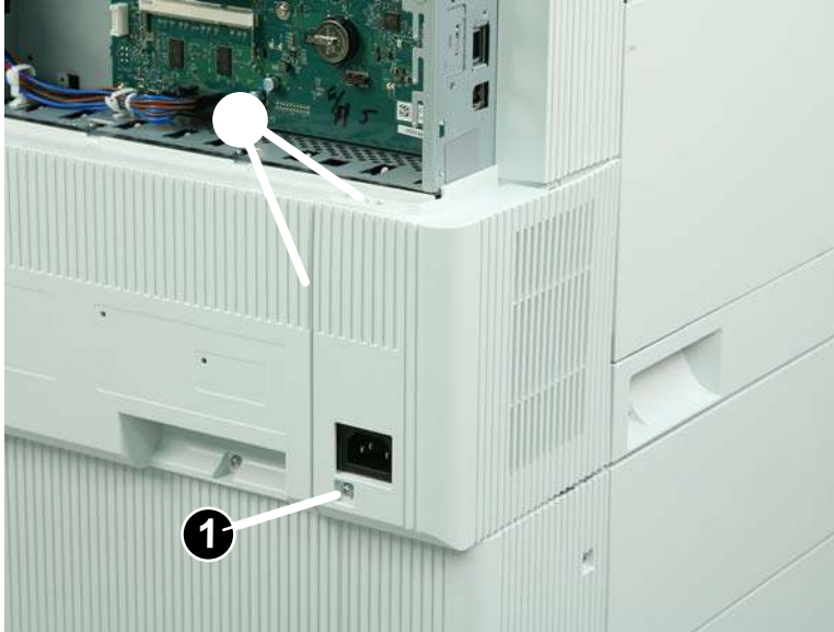
Figure 1-1700 Remove one screw and release two tabs
