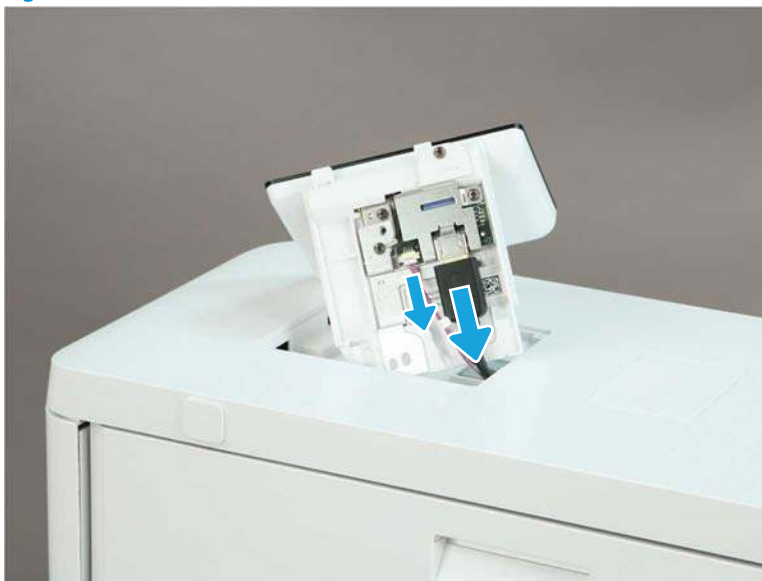
Figure 1-733 Disconnect two connectors
