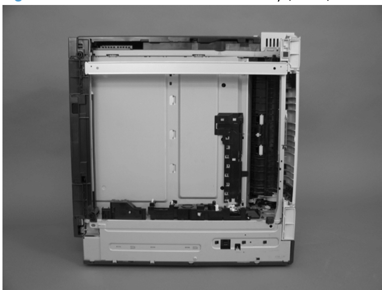
Figure 1-164 Remove the lifter-drive assembly (1 of 3)
