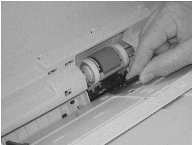
Figure 1-38 Remove the Tray 1 separation pad (4 of 4)
