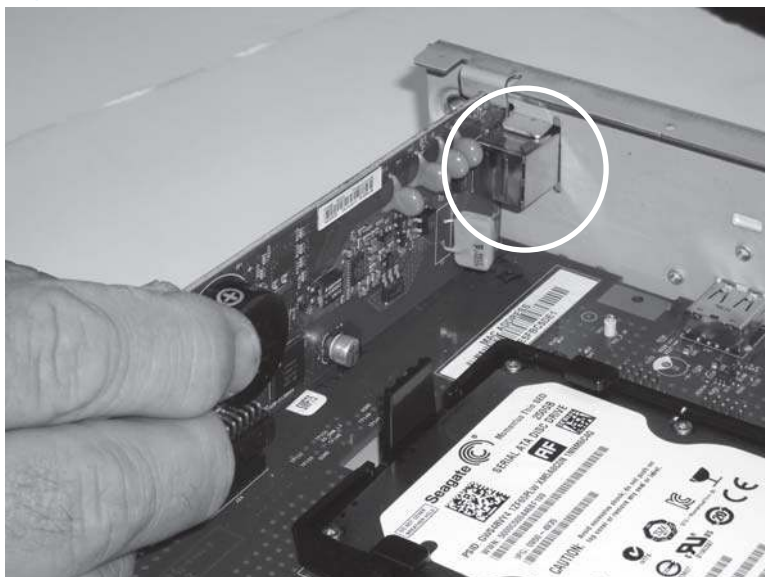
Figure 1-230 Reinstall the fax PCA
