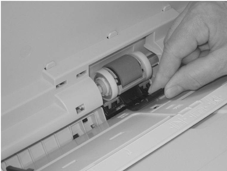
Figure 11 Remove the separation pad (Tray 1) (4 of 4)
