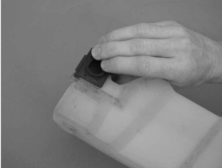
Figure 4 Remove the toner-collection unit (3 of 3)
