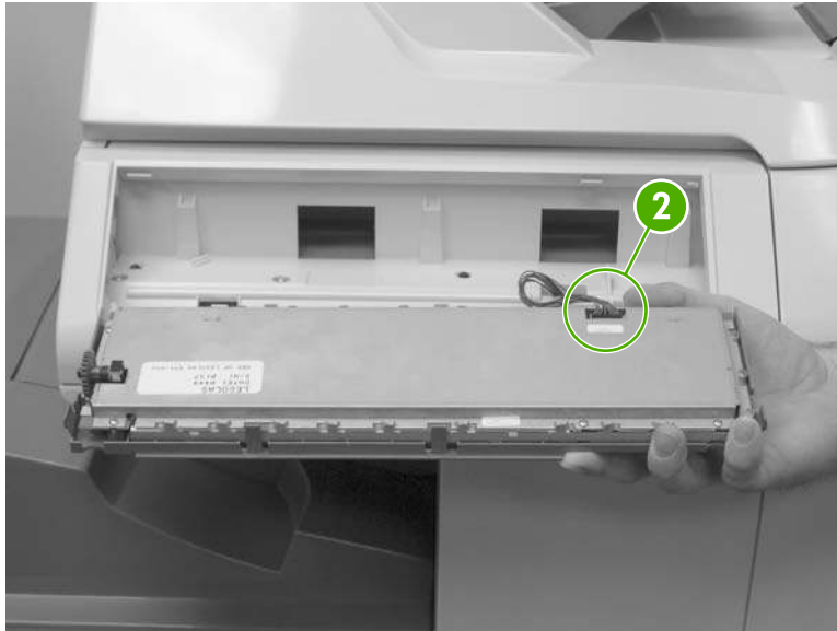
Figure 6-7 Remove the control panel (2 of 3)
