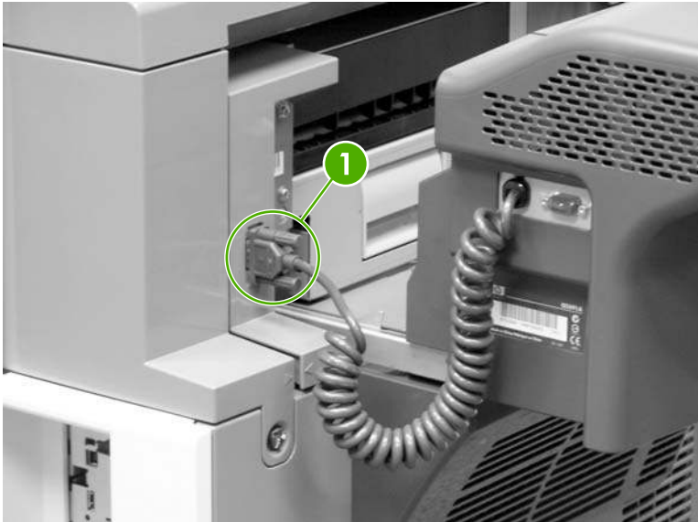
Figure 6-14 Remove the stapler/stacker (3 of 5)
