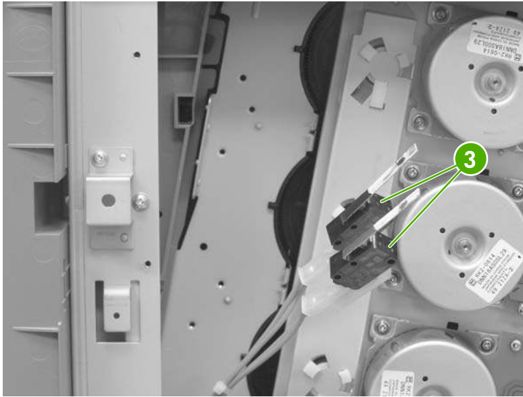
Figure 6-270 Remove the door-open switch assembly (3 of 3)
