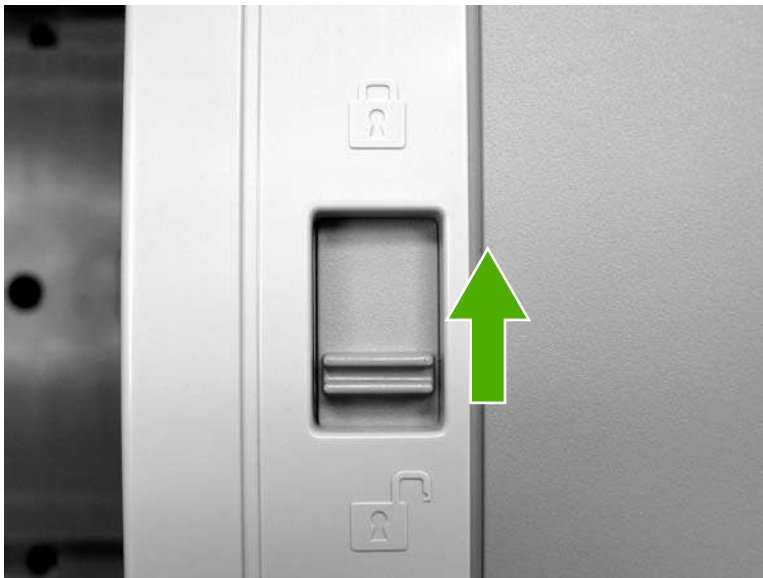
Figure 6-284 Remove the scanner right cover (1 of 2)
