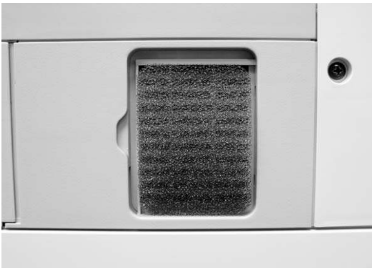
Figure 6-59 Remove the scanner filter (2 of 2)
