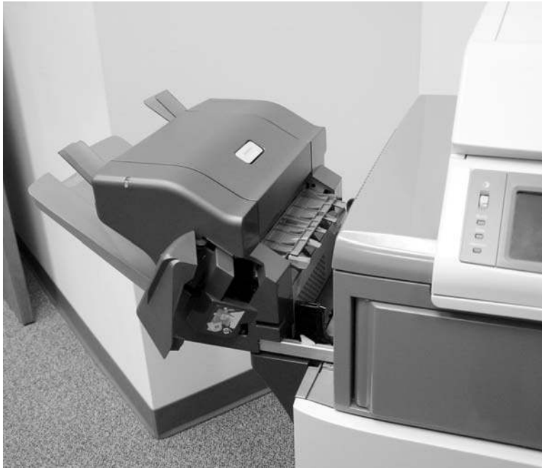
Figure 6-19 Replace the staple cartridge (3 of 3)
