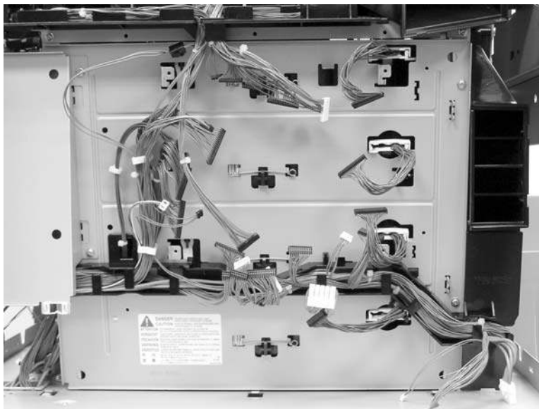
Figure 6-235 Remove the DC controller (2 of 2)
