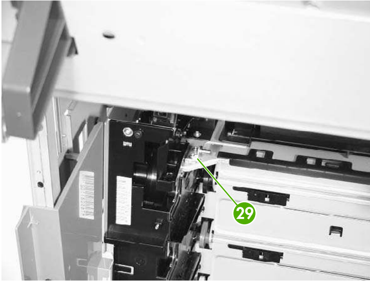
Figure 6-192 Remove the delivery assembly (13 of 15)
