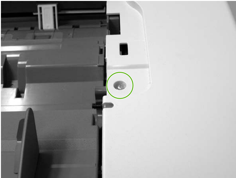
Figure 6-316 Remove the ADF rear cover (2 of 3)
