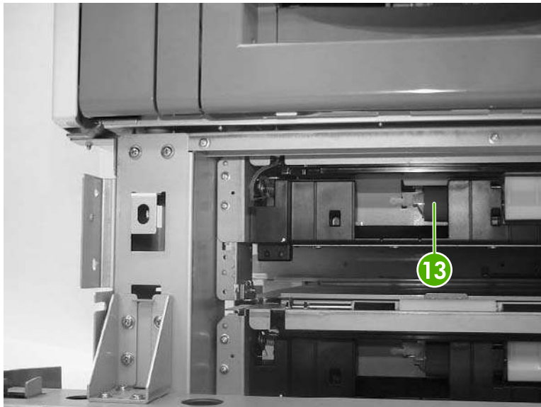
Figure 6-357 Remove the upper pickup assembly (9 of 10)
