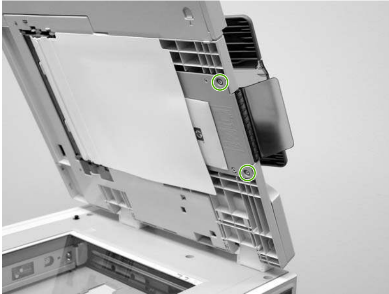
Figure 6-306 Remove the ADF output bin extension (1 of 2)
