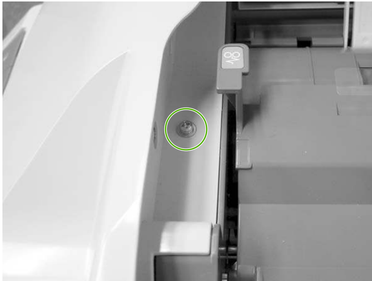
Figure 6-313 Remove the ADF front cover (1 of 2)
