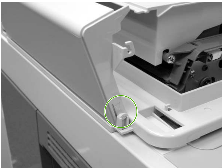
Figure 6-319 Remove the ADF left cover (2 of 2)
