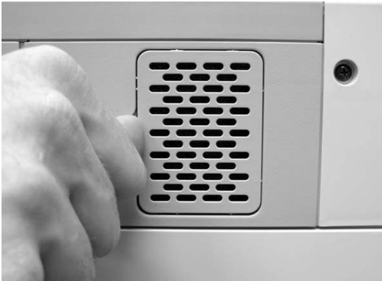
Figure 6-58 Remove the scanner filter (1 of 2)
