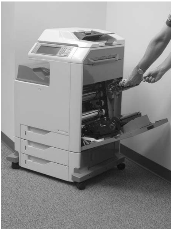
Figure 6-4 Remove the print cartridges (3 of 3)
