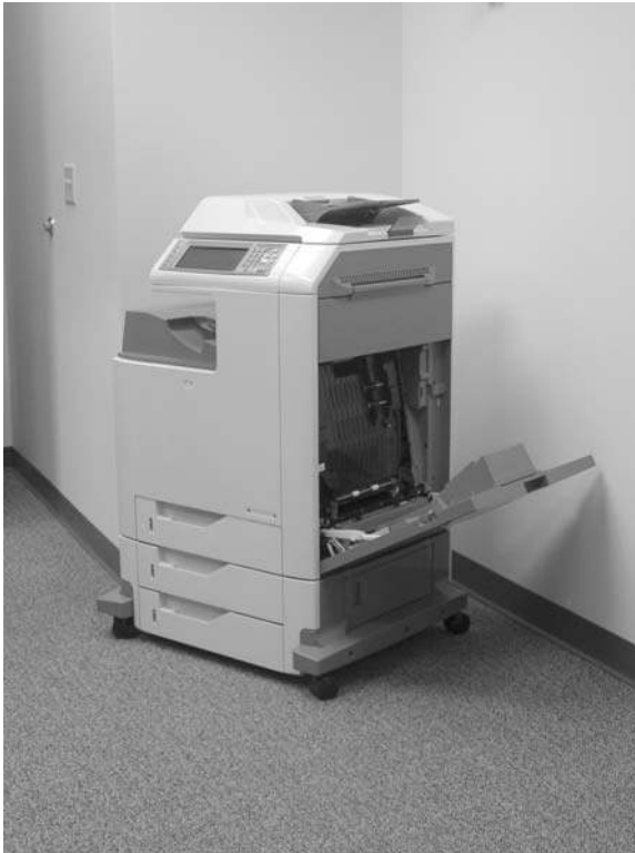
Figure 6-2 Remove the print cartridges (1 of 3)
