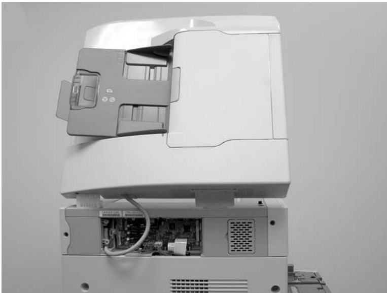
Figure 6-274 Remove the ADF assembly (3 of 3)
