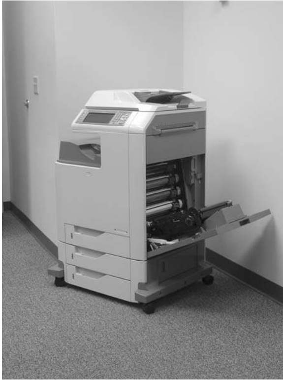
Figure 6-23 Remove the ETB assembly (1 of 4)
