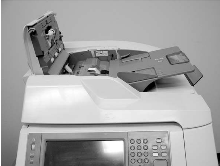
Figure 6-32 Remove the ADF pickup and feed rollers (1 of 3)
