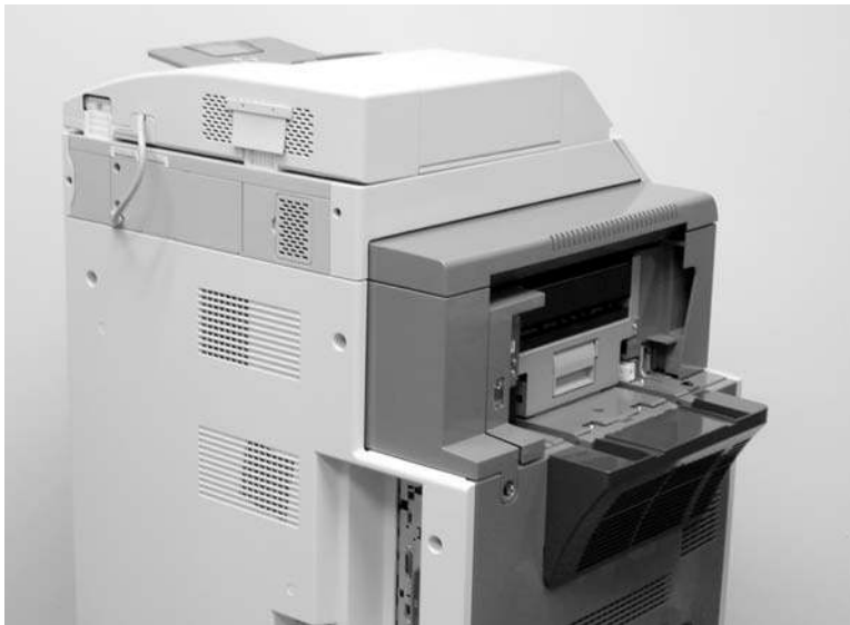
Figure 6-16 Remove the stapler/stacker (5 of 5)
