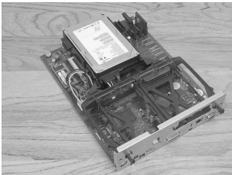
Figure 6-62 Remove the formatter (2 of 2)
