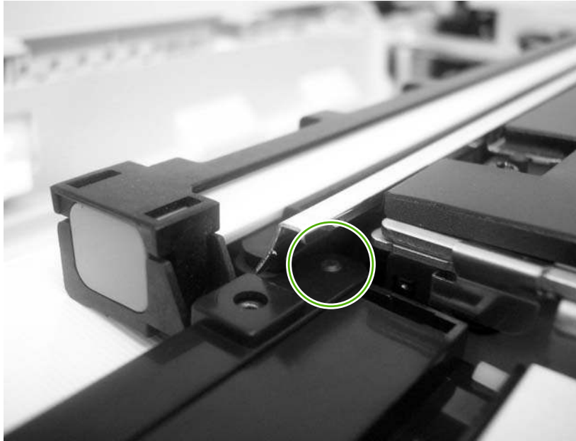
Figure 6-293 Remove the optical assembly (7 of 10)
