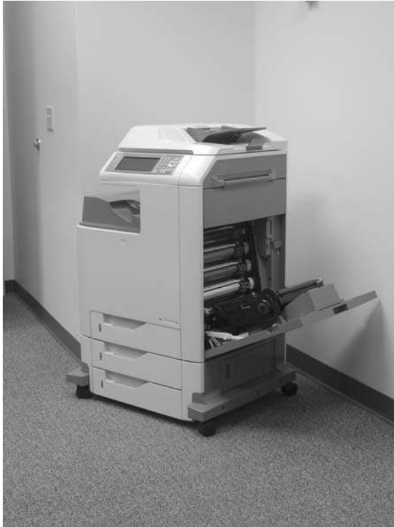
Figure 6-3 Remove the print cartridges (2 of 3)
