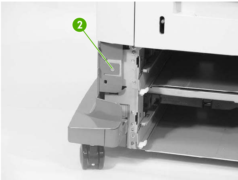
Figure 6-337 Remove the left cover (2 of 3)
