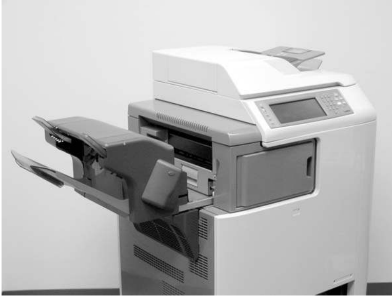
Figure 6-13 Remove the stapler/stacker (2 of 5)
