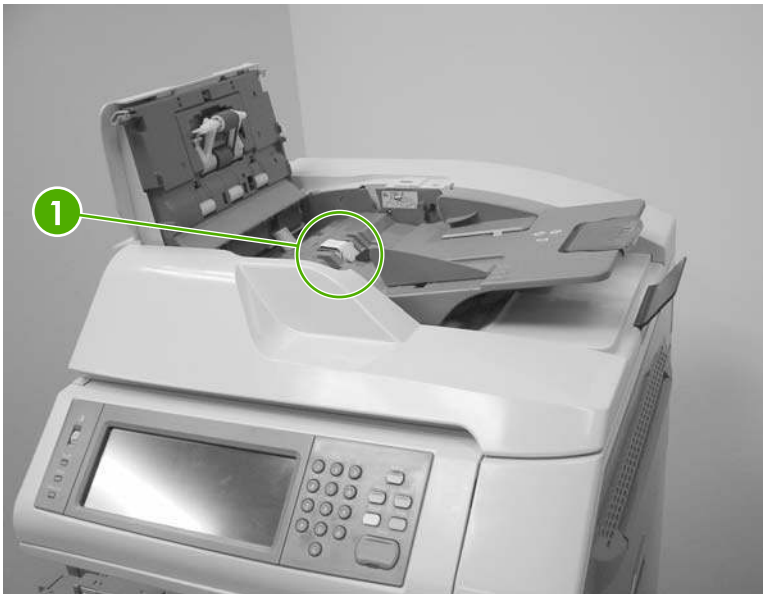
Figure 6-36 Remove the ADF separation pad (2 of 4)
