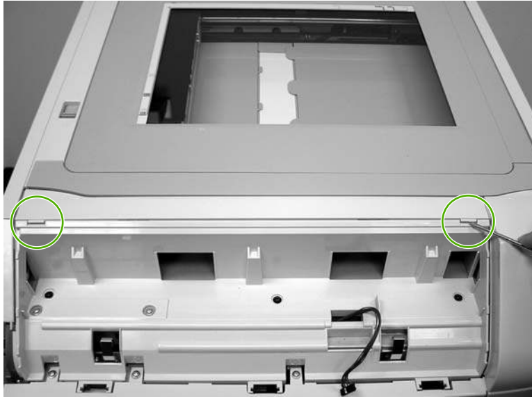
Figure 6-275 Remove the top covers (1 of 2)
