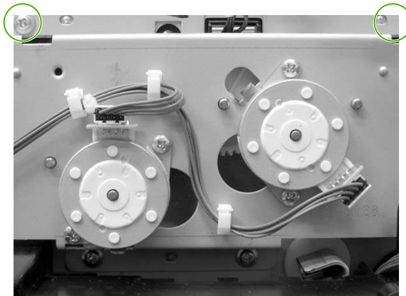
Figure 6-382 Remove the IPTU driver motors (3 of 3)
