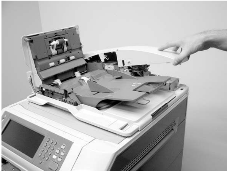
Figure 6-317 Remove the ADF rear cover (3 of 3)
