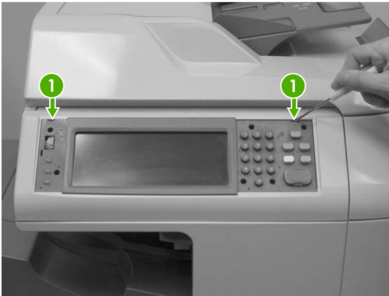
Figure 6-6 Remove the control panel (1 of 3)
