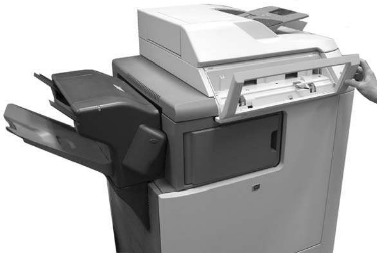
Figure 6-8 Remove the control panel (3 of 3)
