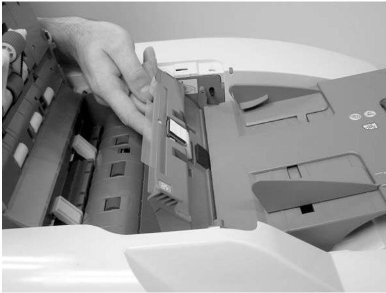
Figure 6-37 Remove the ADF separation pad (3 of 4)
