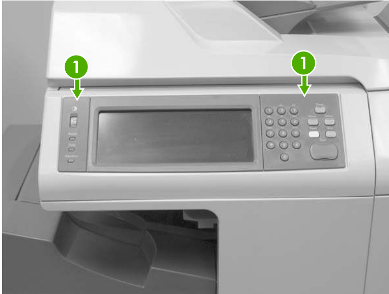
Figure 6-5 Remove the control panel overlays
