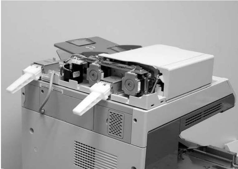
Figure 6-325 Remove the ADF hinges (1 of 3)
