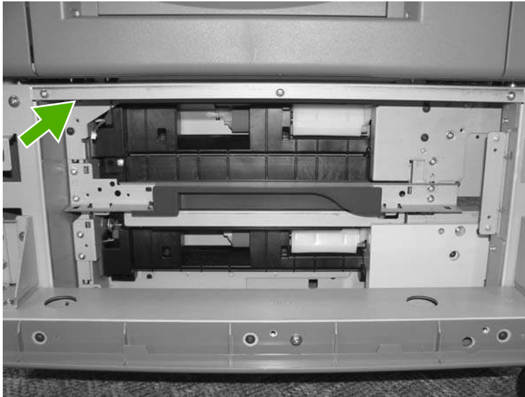
Figure 6-354 Remove the upper pickup assembly (6 of 10)
