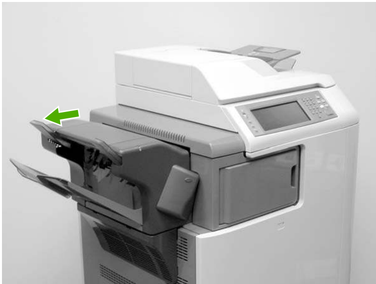
Figure 6-12 Remove the stapler/stacker (1 of 5)
