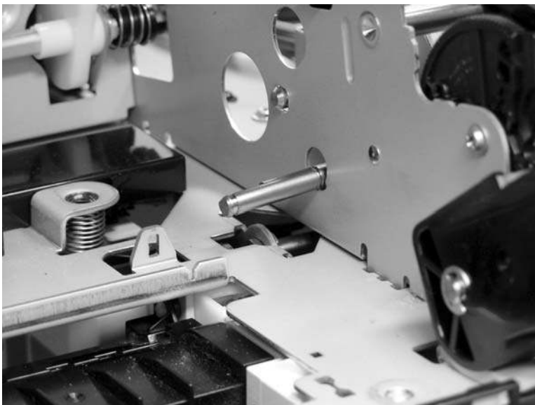
Figure 6-209 Remove the pickup motor assembly (2 of 3)
