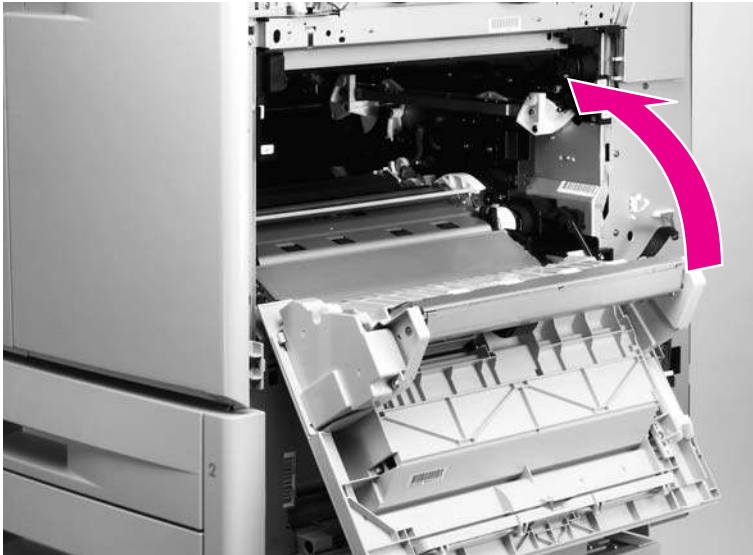
Figure 189. Gain access to the ITB door mounting screws
