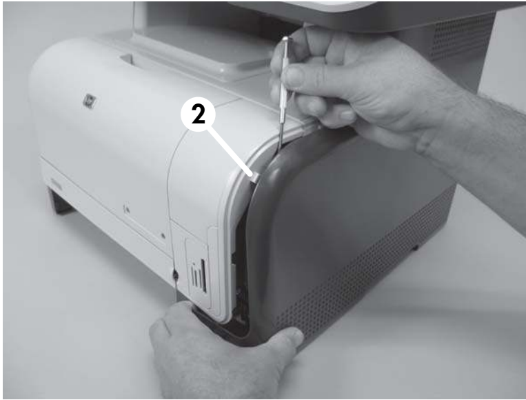
Figure 6-37 Remove the right cover (3 of 5)
