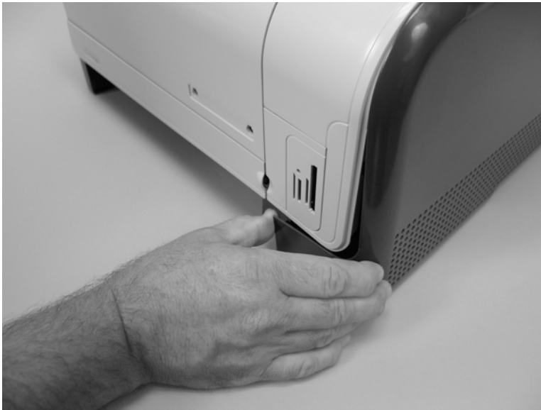
Figure 6-36 Remove the right cover (2 of 5)
