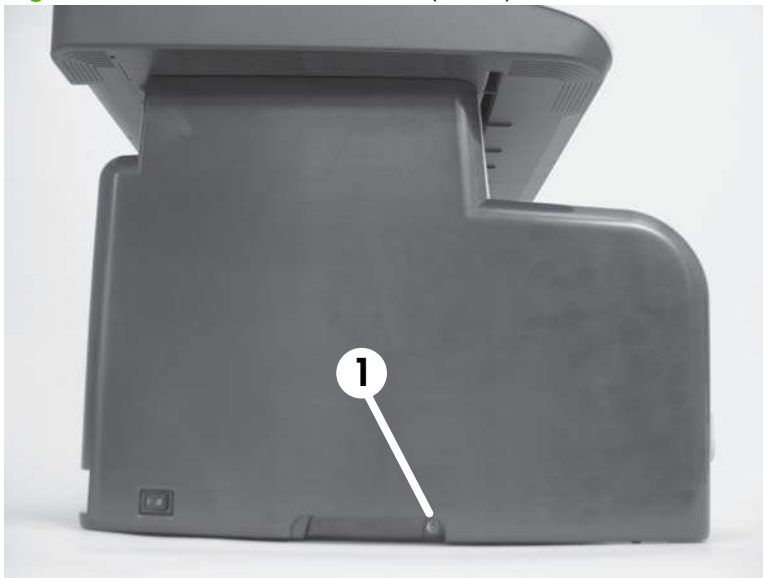
Figure 6-40 Remove the left cover (1 of 4)
