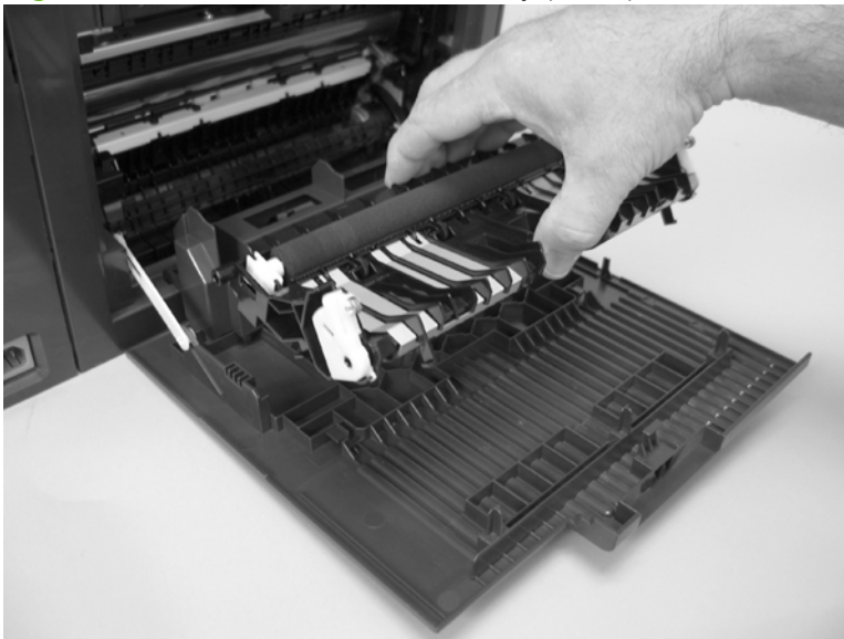
Figure 6-42 Remove the feed assembly (2 of 2)
