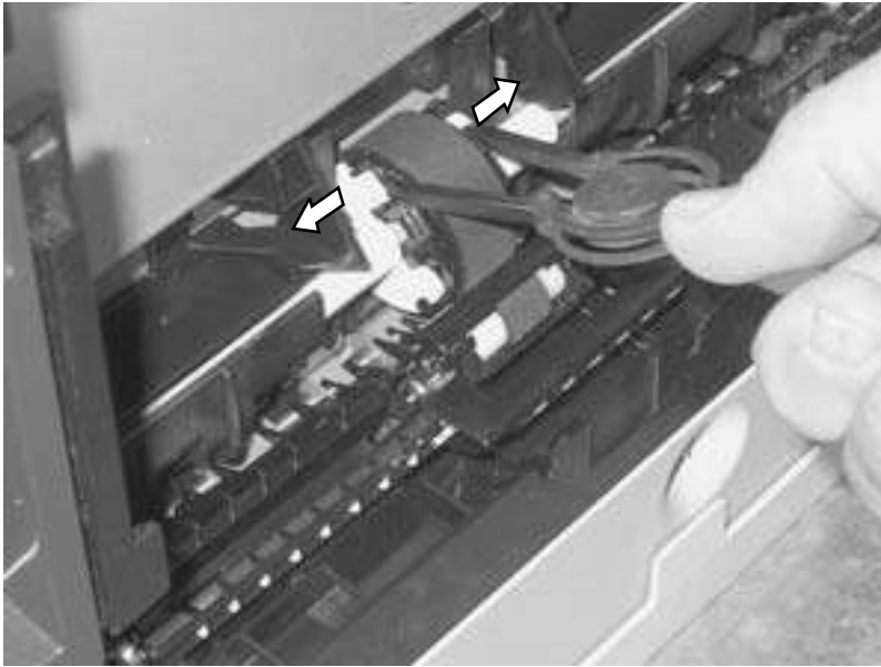
Figure 6-10 Remove the pickup roller (2 of 2)
