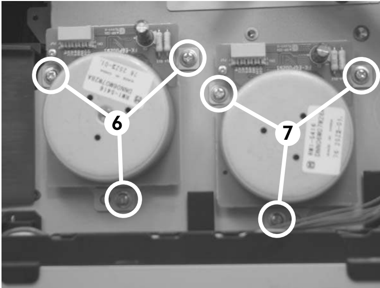
Figure 6-38 Remove motor M1 and motor M2 (3 of 3)
