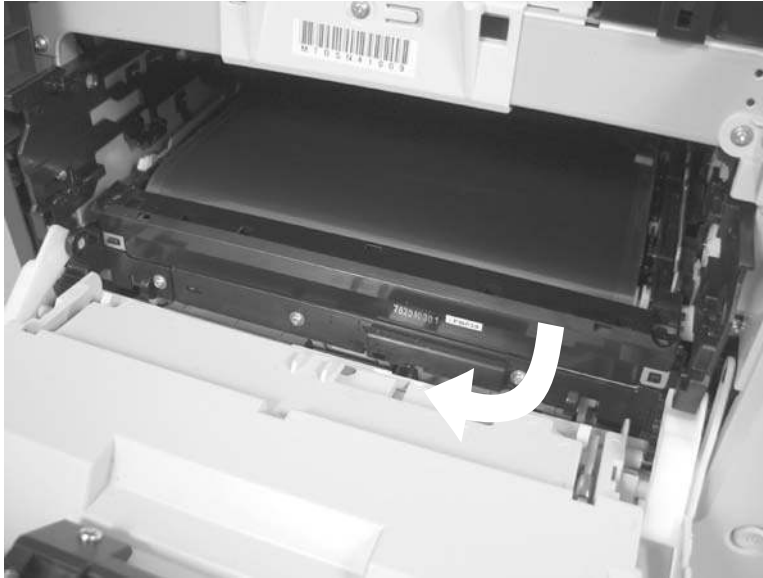
Figure 6-30 Remove the ITB (2 of 6)
