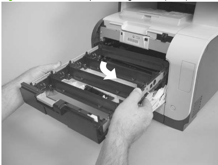
Figure 6-27 Remove the print-cartridge drawer (2 of 3)
