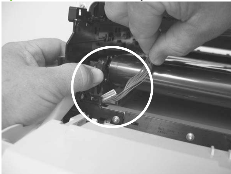
Figure 6-116 Reinstall the color-misregistration sensor assembly PCA (1 of 2)
