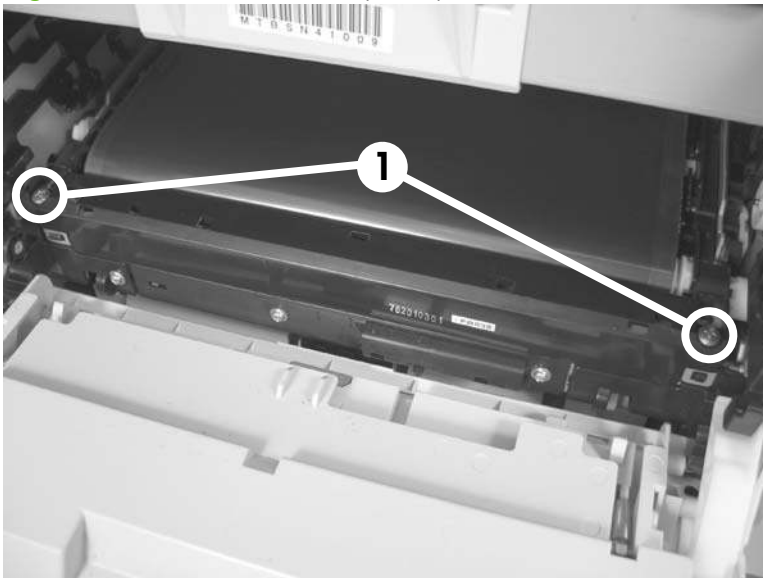
Figure 6-29 Remove the ITB (1 of 6)
