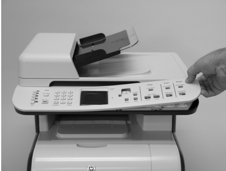
Figure 6-5 Remove the control-panel bezel
