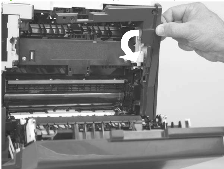
Figure 6-67 Remove the rear-upper cover (2 of 2)
