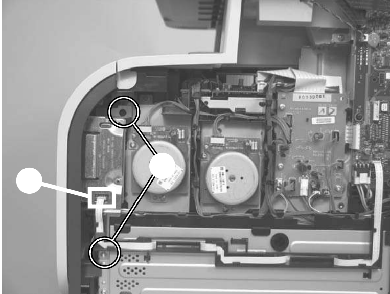
Figure 6-125 Remove the memory-card cover and PCA (1 of 7)
