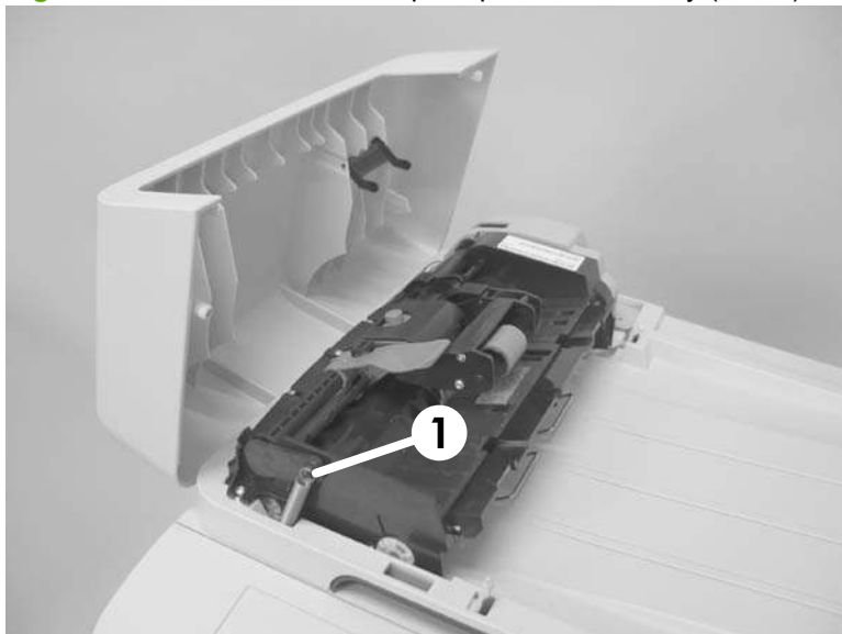
Figure 6-15 Remove the ADF pickup roller assembly (1 of 2)
