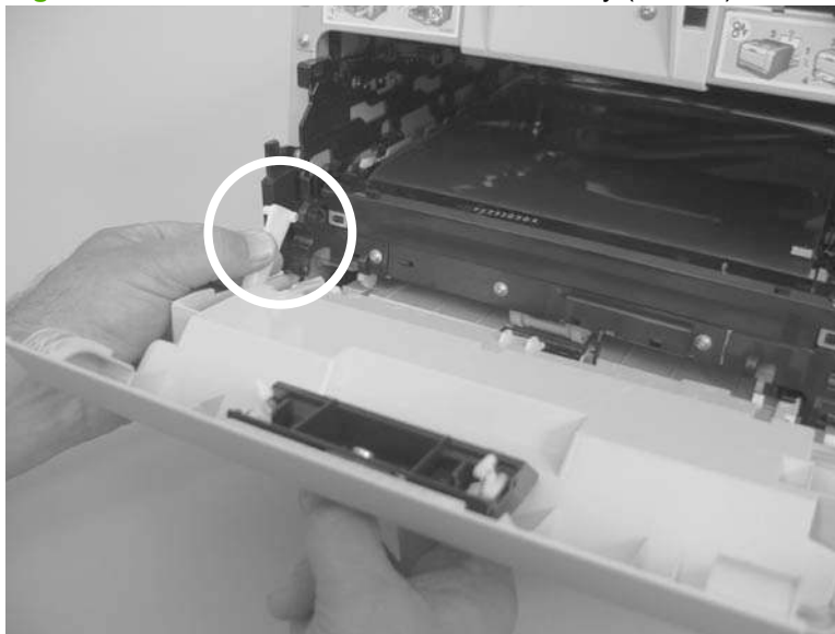
Figure 6-142 Remove the front-door assembly (9 of 10)
