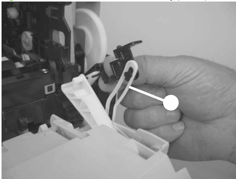
Figure 6-138 Remove the front-door assembly (5 of 10)
