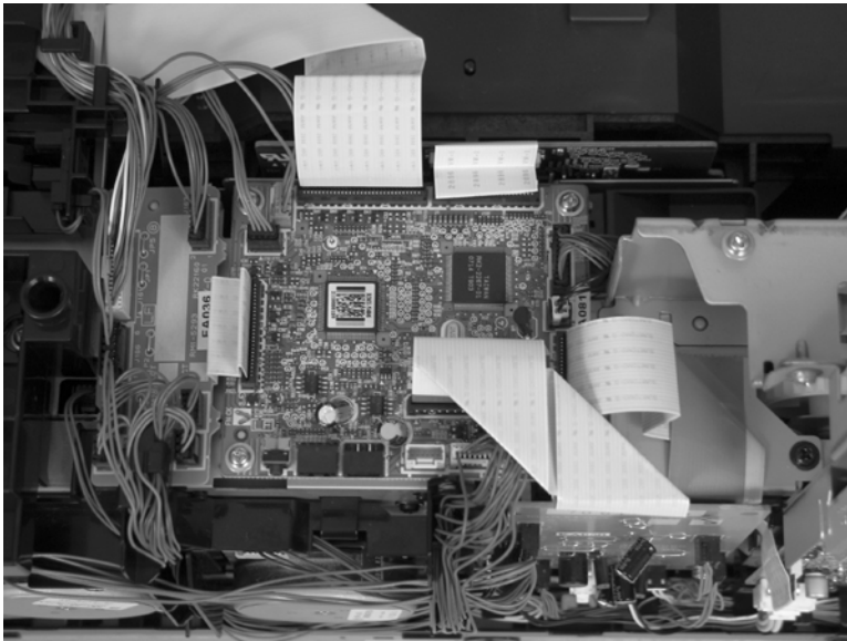
Figure 6-60 Remove the DC controller PCA (1 of 2)
