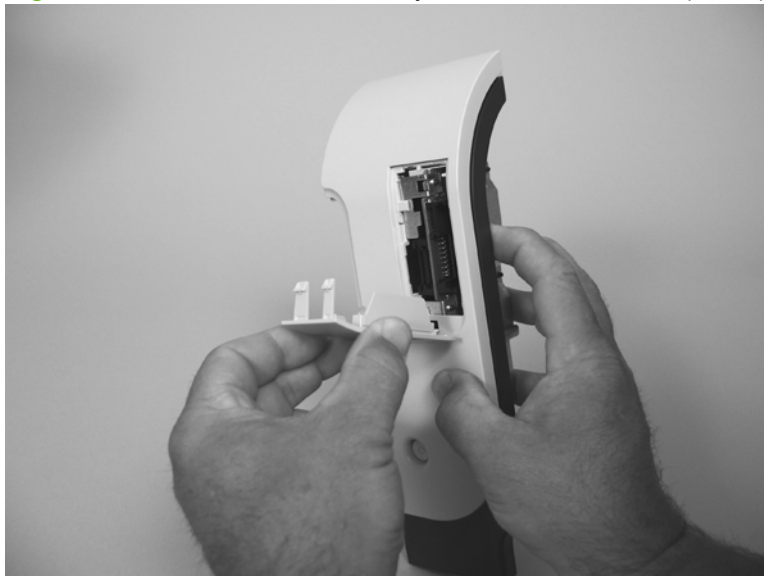
Figure 6-132 Reinstall the memory-card cover and PCA (1 of 2)
