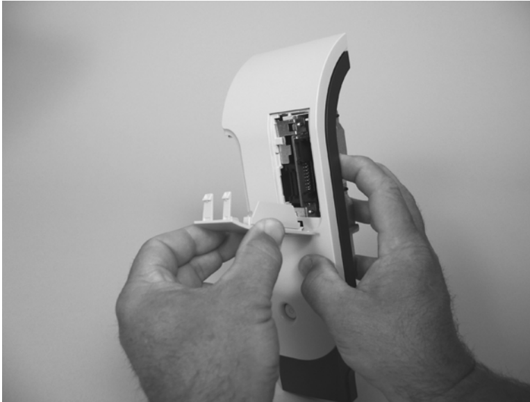
Figure 6-130 Remove the memory-card cover and PCA (6 of 7)
