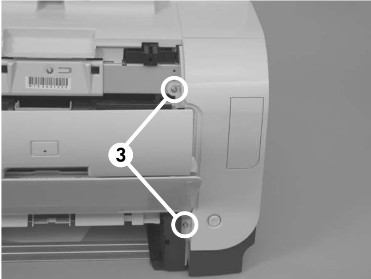
Figure 6-126 Remove the memory-card cover and PCA (2 of 7)
