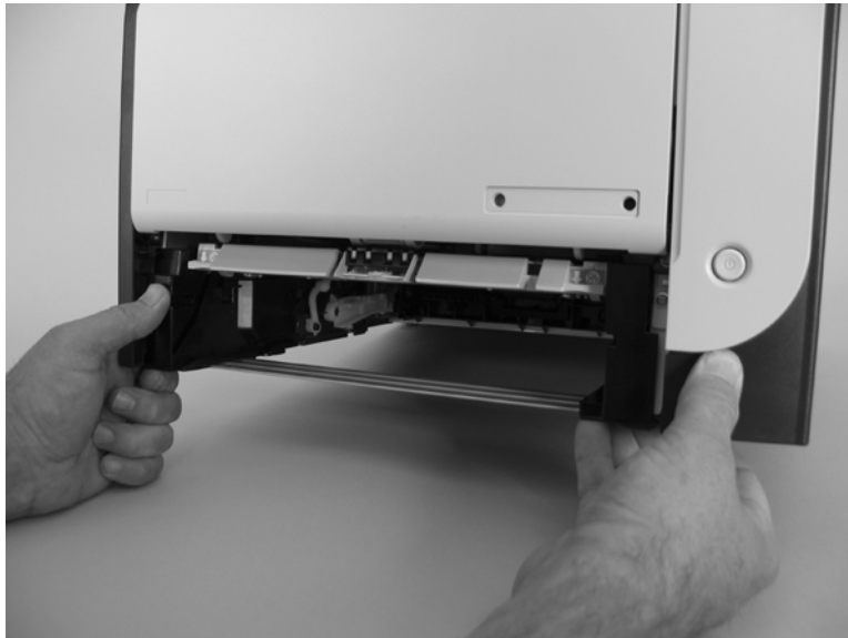
Figure 6-18 Remove the Tray 1 paper-pickup roller (2 of 3)
