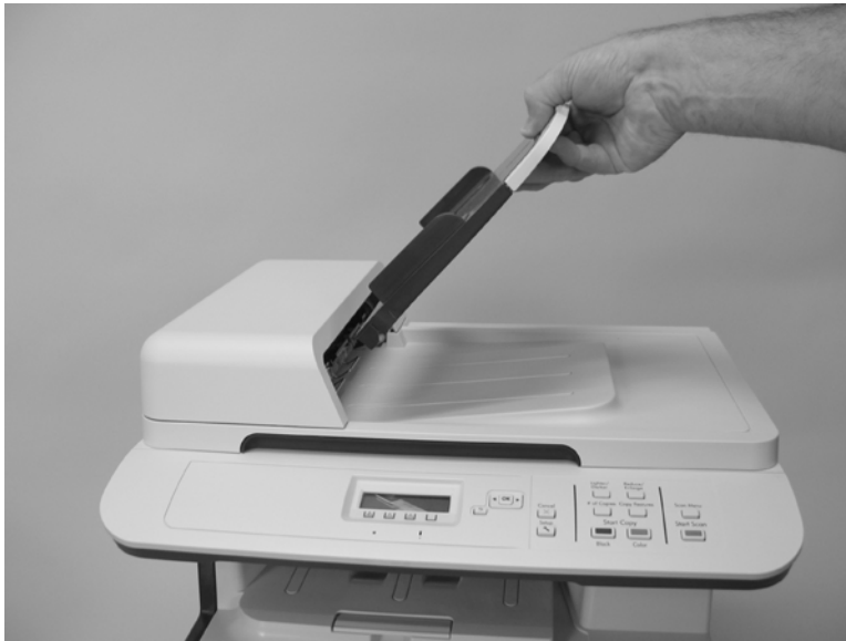
Figure 6-24 Remove the ADF input tray
