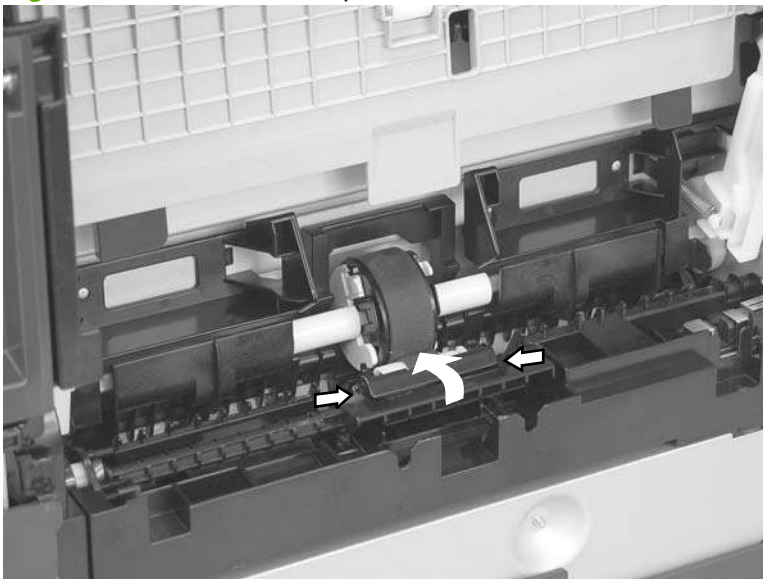
Figure 6-14 Reinstall the separation roller
