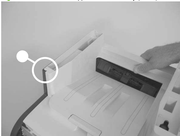
Figure 6-97 Reinstall the upper-cover assembly (1 of 3)
