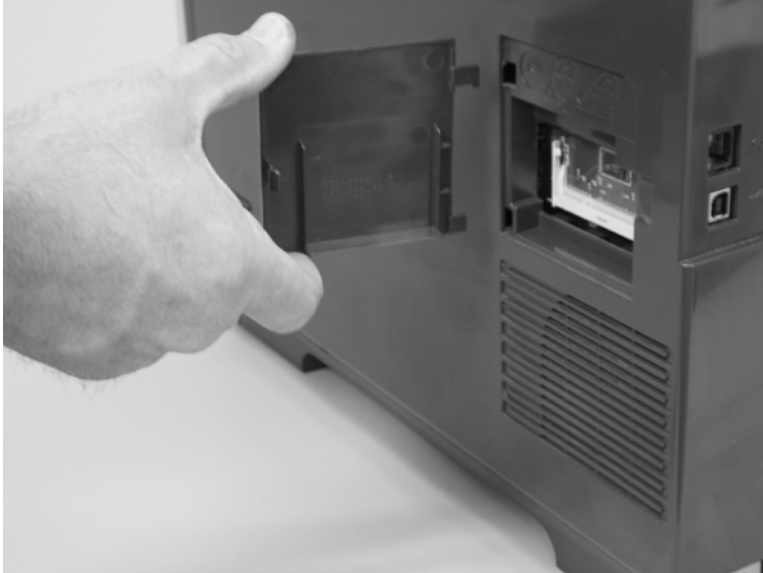
Figure 6-25 Remove the DIMM cover
