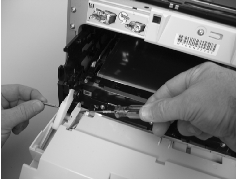
Figure 6-135 Remove the front-door assembly (2 of 10)
