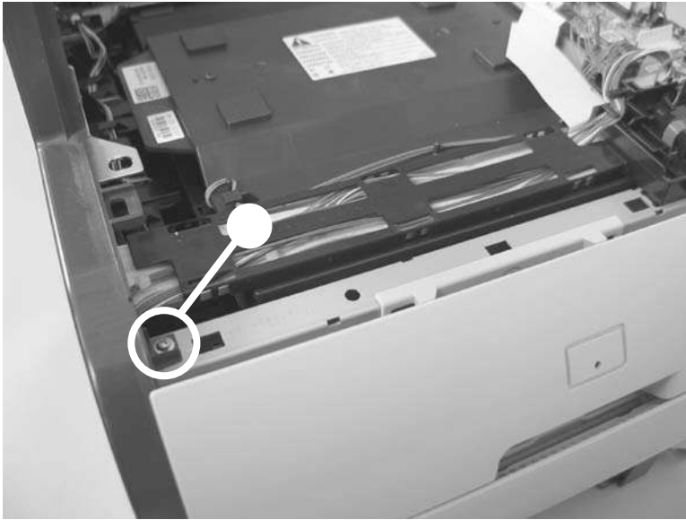
Figure 6-101 Remove the left cover (2 of 4)
