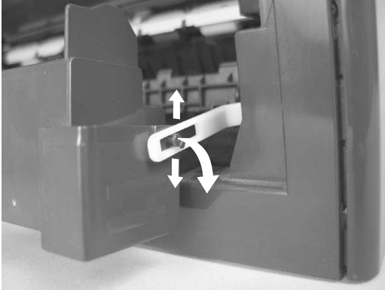
Figure 6-68 Remove the rear cover and feed guide (simplex product) (1 of 6)
