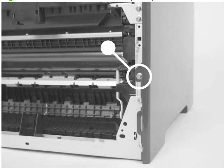
Figure 6-100 Remove the left cover (1 of 4)
