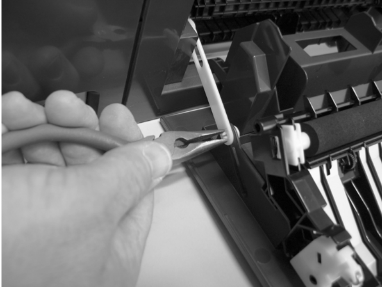
Figure 6-45 Remove the rear door (simplex product) (1 of 4)
