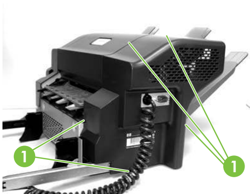
Figure 5-374 Claw locations on rear cover
