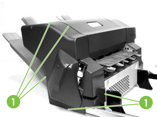
Figure 5-373 Claw locations on front cover
