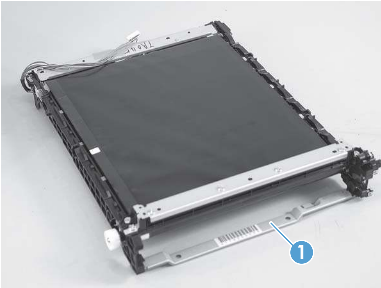
Figure 1-63 Reinstall the ITB (1 of 2)
