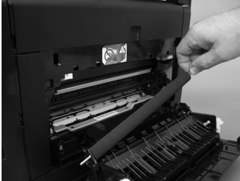
Figure 1-8 Remove the transfer roller (3 of 3)
