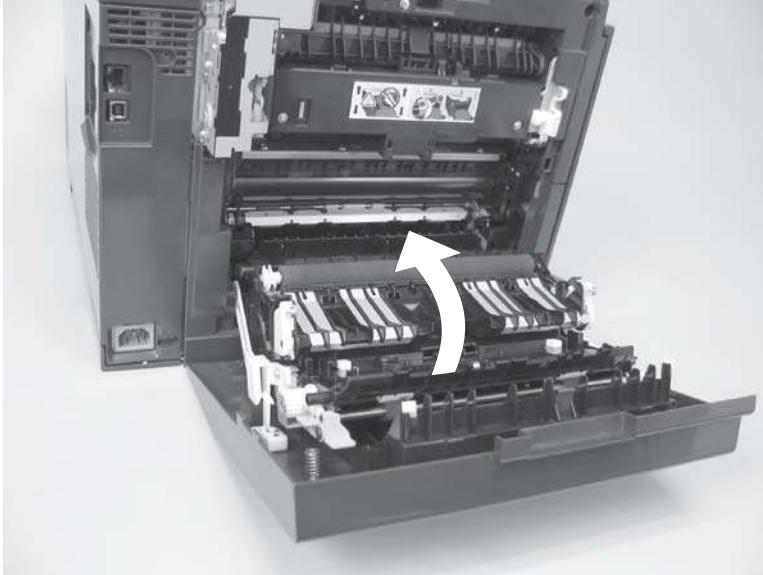
Figure 1-33 Remove the rear door (duplex product) (1 of 4)
