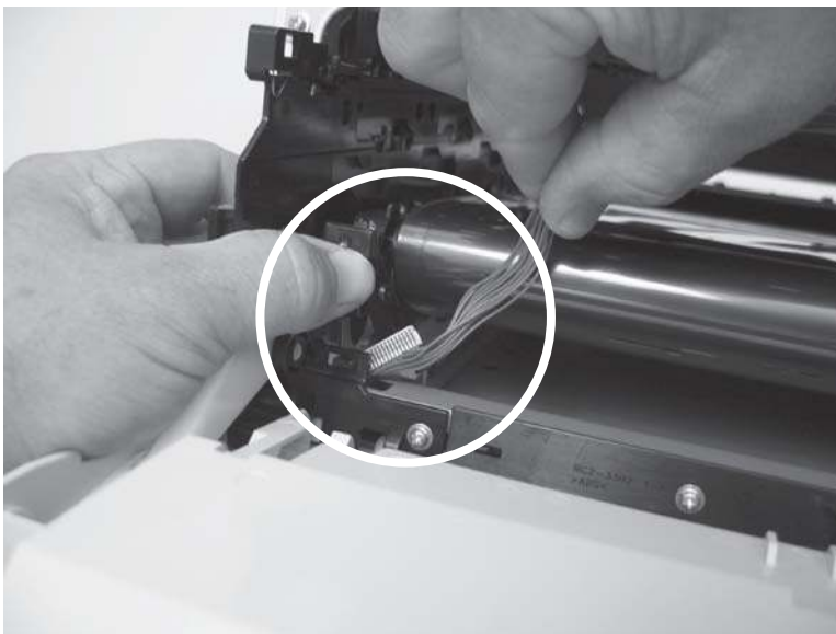
Figure 1-125 Reinstall the color-misregistration sensor assembly PCA (1 of 2)
