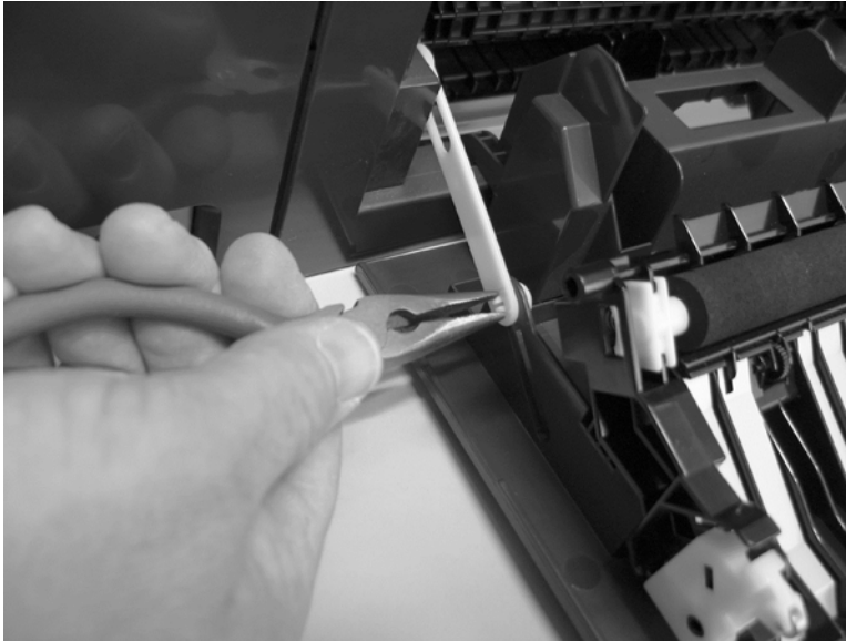
Figure 1-29 Remove the rear door (simplex product) (1 of 4)
