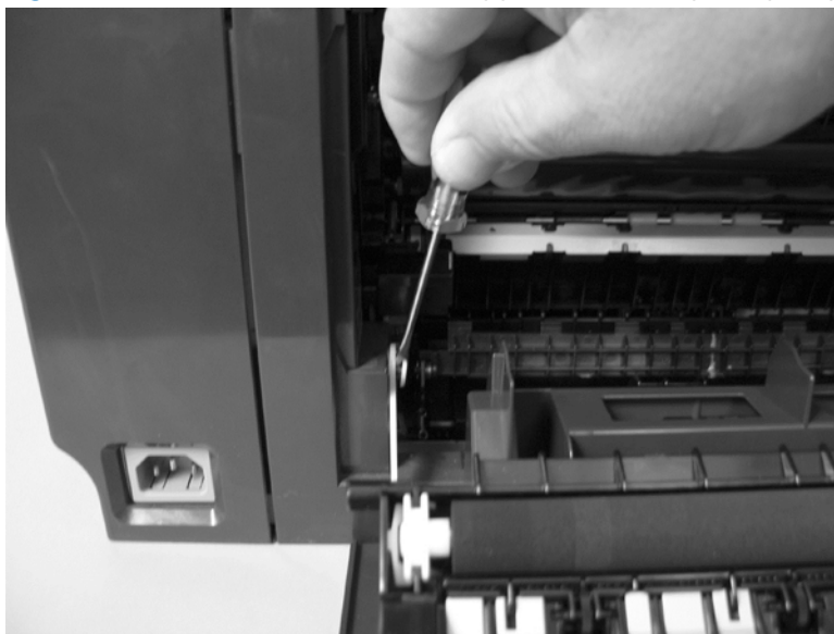
Figure 1-28 Remove the rear-door stopper and link cap (simplex product) (2 of 2)
