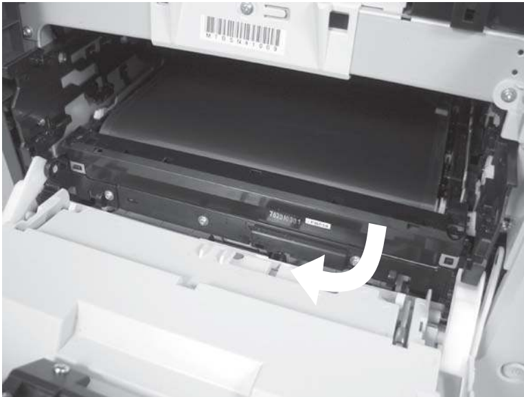
Figure 1-93 Remove the ITB (2 of 6)
