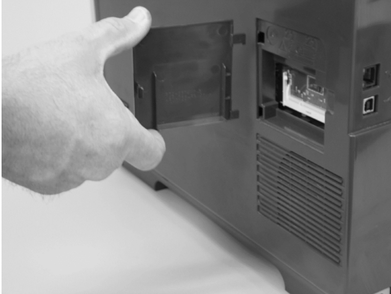
Figure 1-18 Remove the DIMM cover
