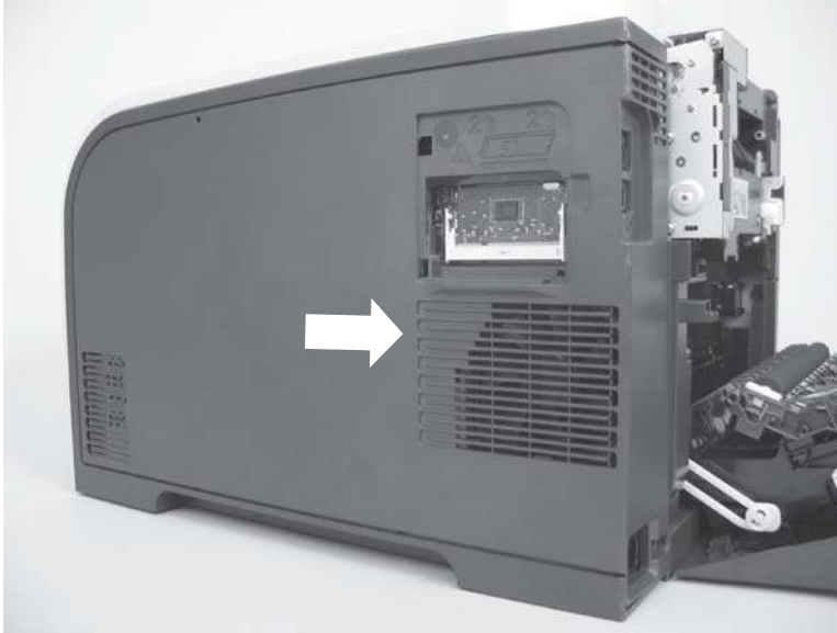
Figure 1-21 Remove the right cover (3 of 5)
