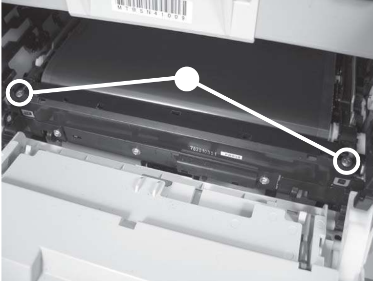
Figure 1-92 Remove the ITB (1 of 6)
