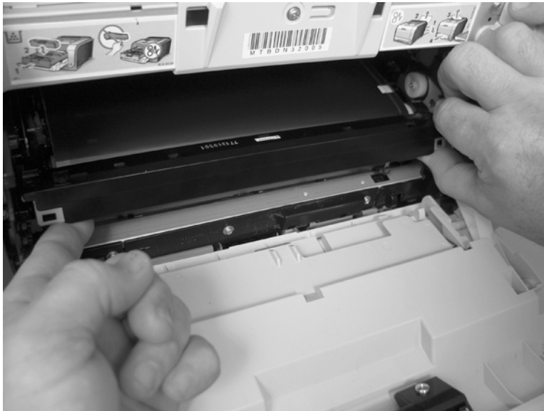
Figure 1-95 Remove the ITB (4 of 6)
