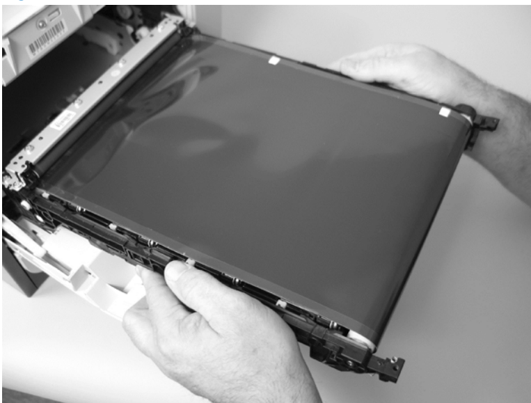
Figure 1-97 Remove the ITB (6 of 6)
