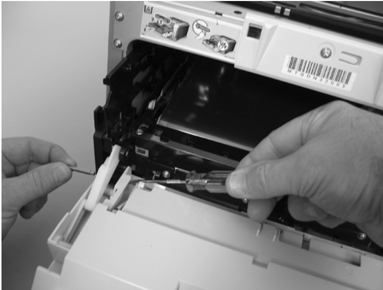
Figure 1-81 Remove the front-door assembly (2 of 10)
