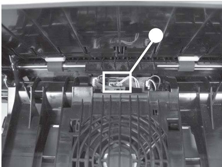
Figure 1-129 Remove the duplex reverse-drive assembly (1 of 4)
