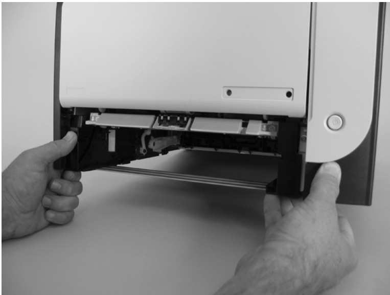
Figure 1-12 Remove the Tray 1 paper-pickup roller (2 of 3)
