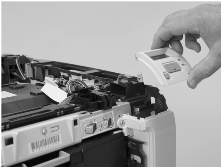
Figure 1-71 Remove the control-panel assembly (3 of 3)
