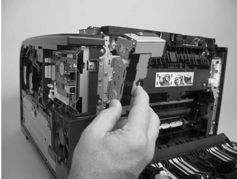
Figure 1-132 Remove the duplex reverse-drive assembly (4 of 4)
