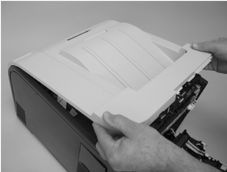
Figure 1-57 Remove the upper-cover assembly (4 of 4)
