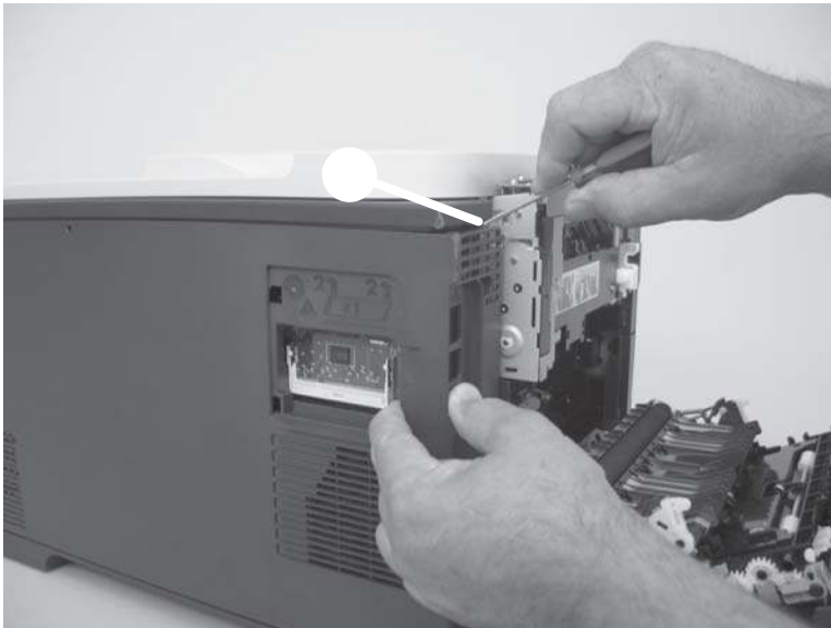
Figure 1-22 Remove the right cover (4 of 5)
