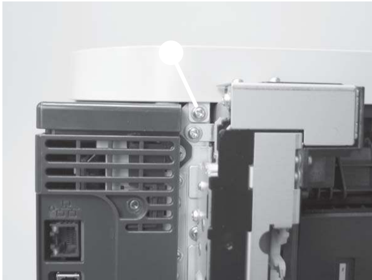
Figure 1-54 Remove the upper-cover assembly (1 of 4)
