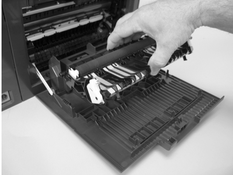
Figure 1-68 Remove the feed assembly (2 of 2)
