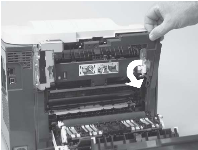
Figure 1-26 Remove the rear-upper cover (2 of 2)
