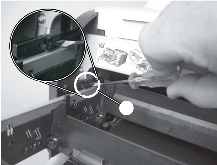
Figure 1-15 Remove the print-cartridge drawer (1 of 3)
