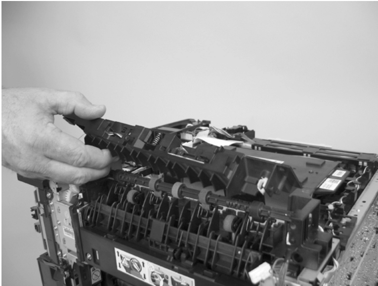
Figure 1-145 Remove the paper-delivery assembly (4 of 4)
