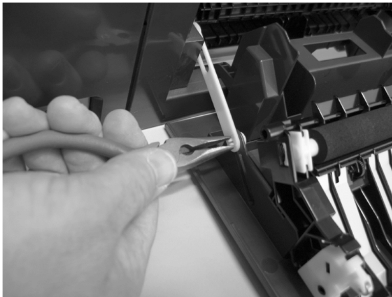
Figure 1-27 Remove the rear-door stopper and link caps (simplex product) (1 of 2)
