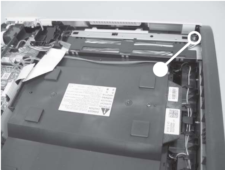
Figure 1-60 Remove the left cover (1 of 3)
