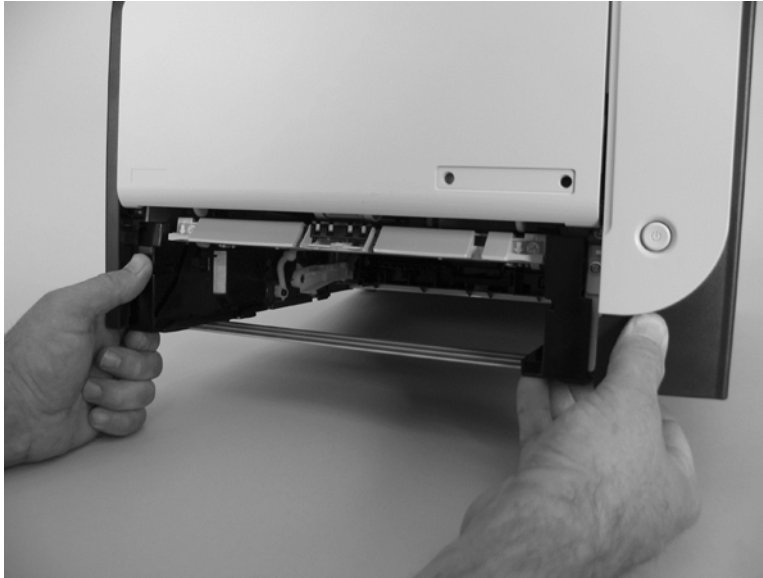
Figure 1-5 Remove the pickup roller (1 of 2)
