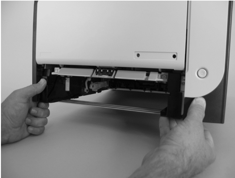
Figure 1-7 Remove the separation roller (1 of 3)
