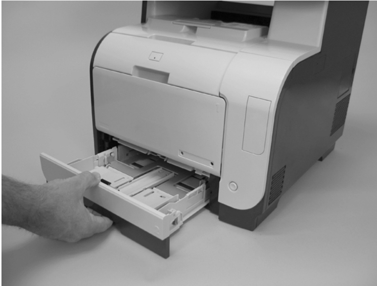
Figure 1-150 Remove the tray cassettes and optional Tray 3 assembly (1 of 2)
