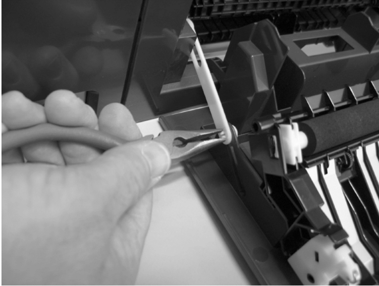
Figure 1-33 Remove the Rear-door stopper and link caps (simplex product) (1 of 2)
