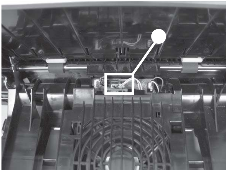
Figure 1-133 Remove the duplex-reverse drive assembly (1 of 4)
