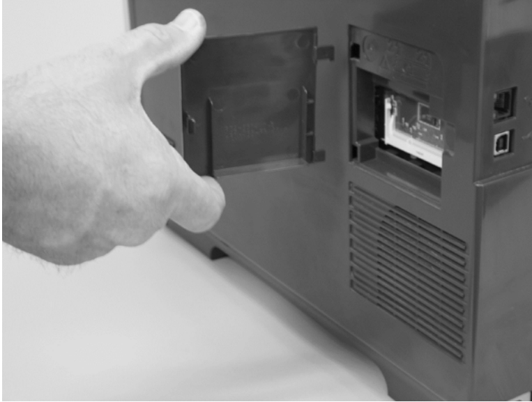
Figure 1-19 Remove the DIMM cover
