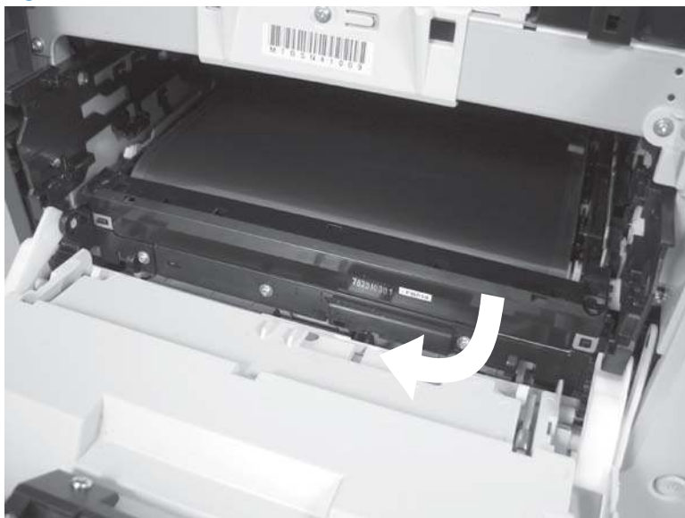
Figure 1-89 Remove the ITB (2 of 6)
