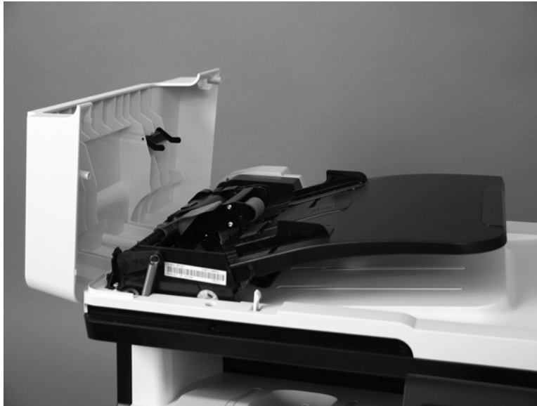
Figure 1-23 Remove the document feeder input tray (2 of 2)
