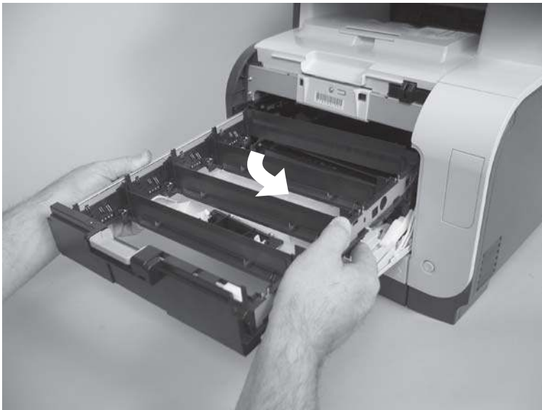
Figure 1-17 Remove the print-cartridge drawer (2 of 3)
