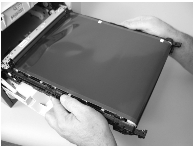
Figure 1-93 Remove the ITB (6 of 6)
