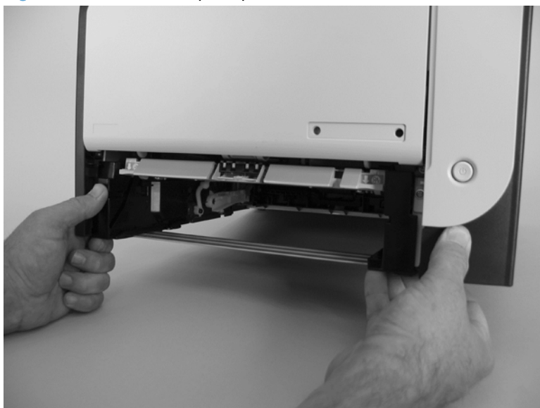
Figure 1-6 Remove the pickup roller (1 of 3)
