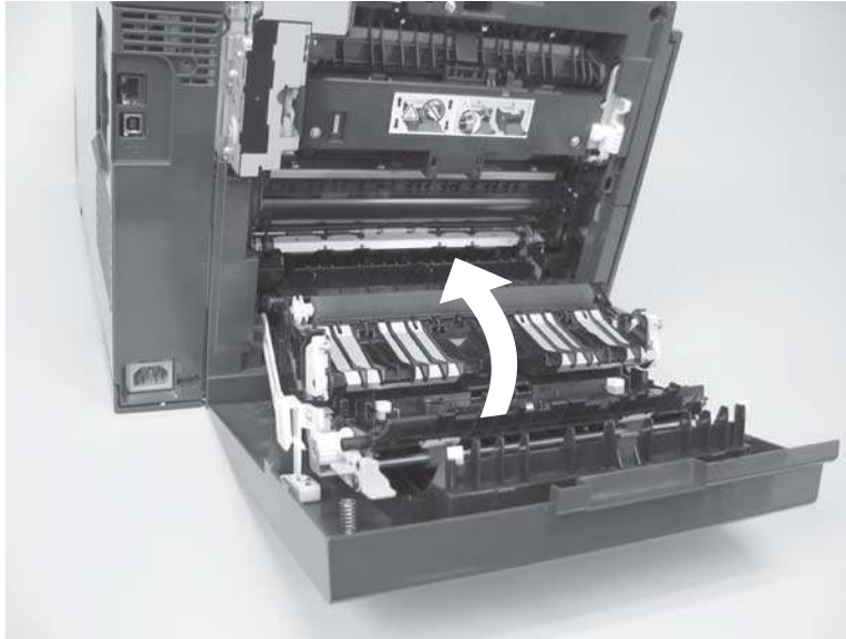
Figure 1-39 Remove the rear door (duplex product) (1 of 4)
