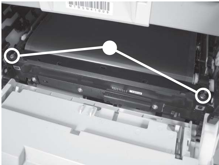
Figure 1-88 Remove the ITB (1 of 6)
