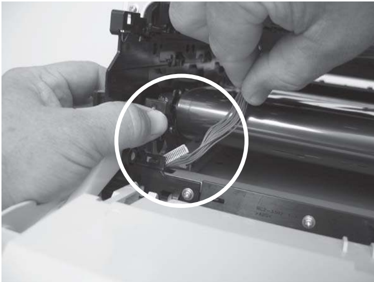
Figure 1-109 Reinstall the color-misregistration sensor assembly PCA (1 of 2)
