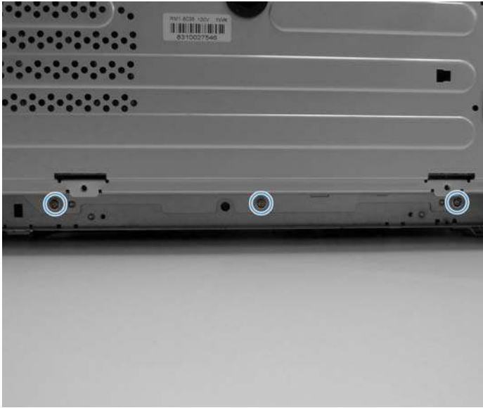
Figure 1-142 Remove the screws securing the low voltage power supply
