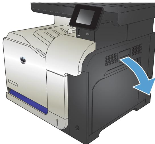
2. If paper is jammed as it enters the output bin, gently pull the paper downward to remove it.
