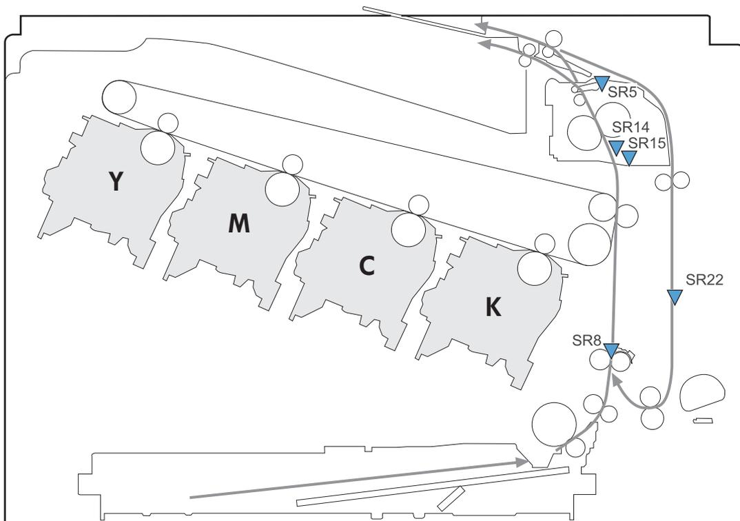
The product determines that a jam has occurred if one of these sensors detects paper at an inappropriate time. The DC controller stops the print operation and notifies the formatter.
