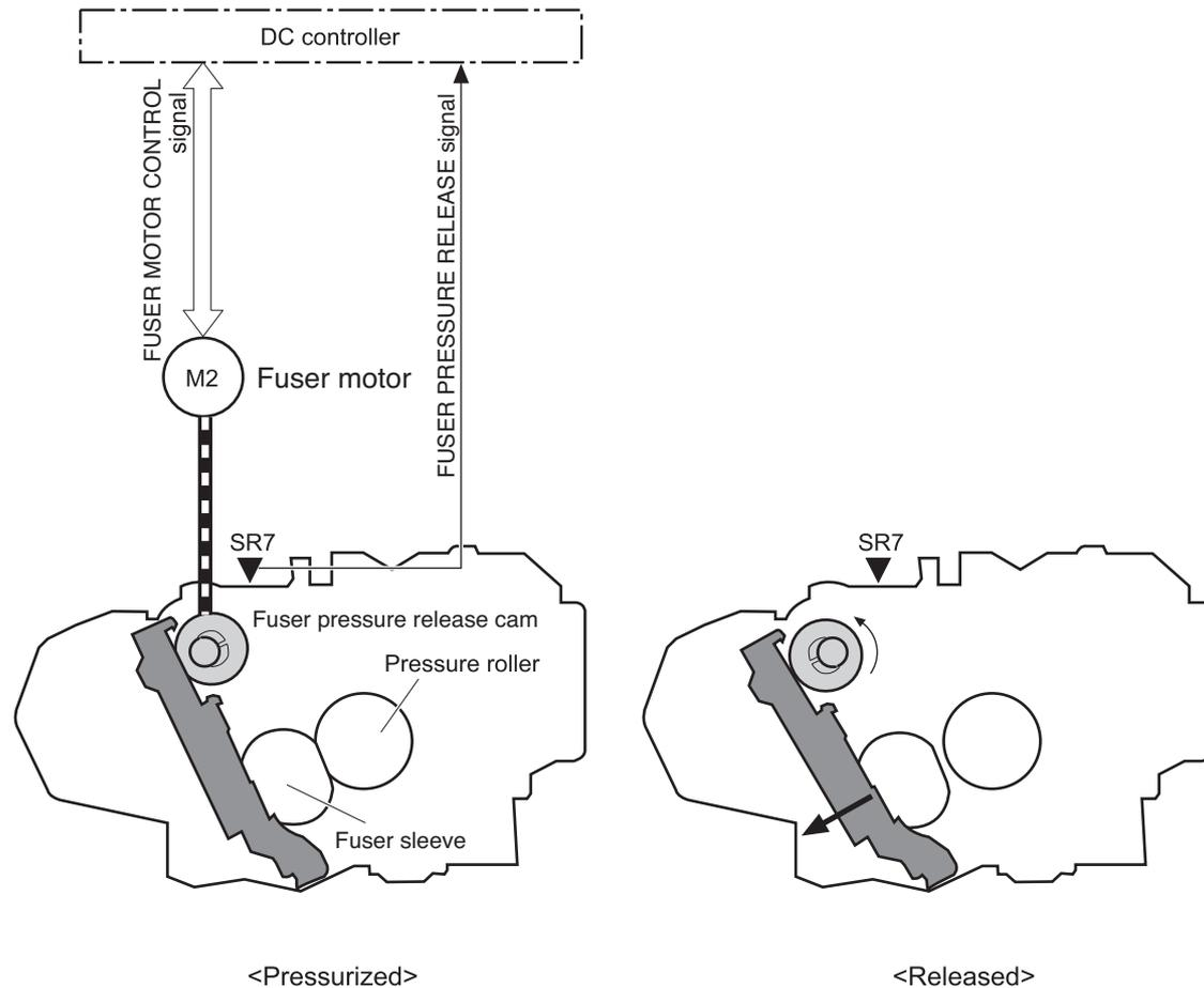
The pressure roller depressurizes under the following conditions:
