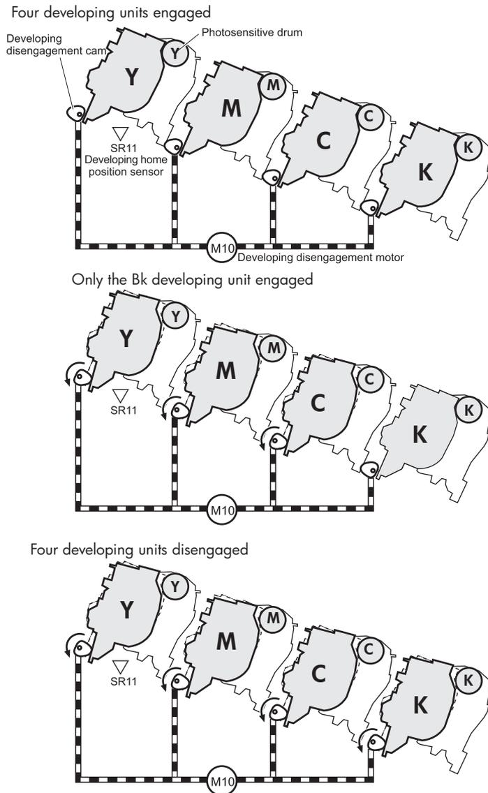
The DC controller rotates the developing disengagement motor and changes the direction of the cam according to the instructions from the formatter for each print job.
