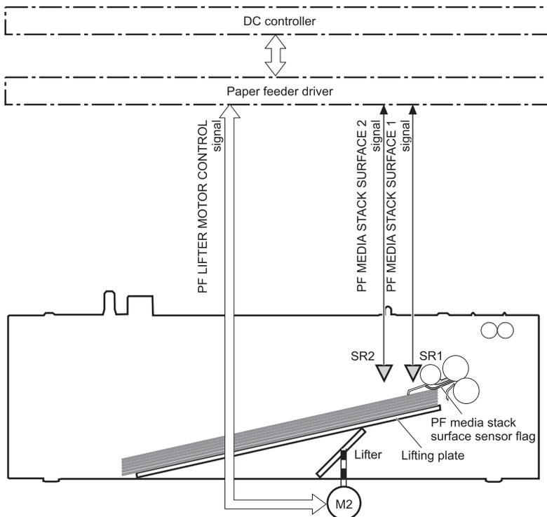
The paper-feeder driver notifies the formatter if either of the paper-feeder media-stack surface sensors fails to detect the stack surface within a specified period from when a lift-up operation starts.
