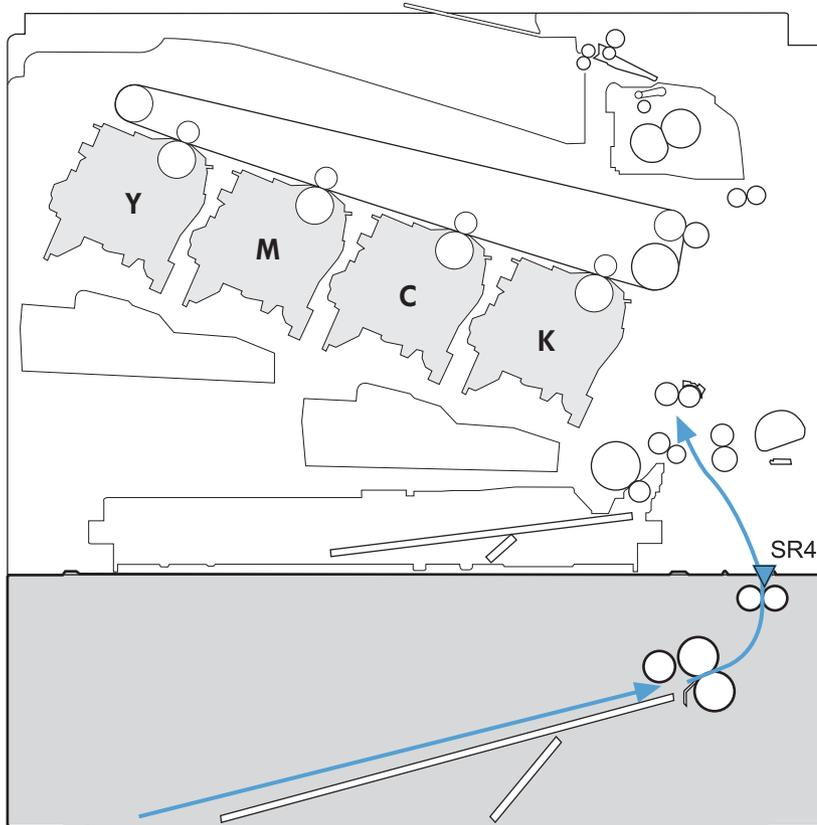
The paper-feeder driver identifies a jam if the sensor detects paper at a specified timing stored in the paper-feeder driver. The paper-feeder driver stops printing and notifies the formatter through the DC controller of the jam. The paper feeder detects the following jams:
