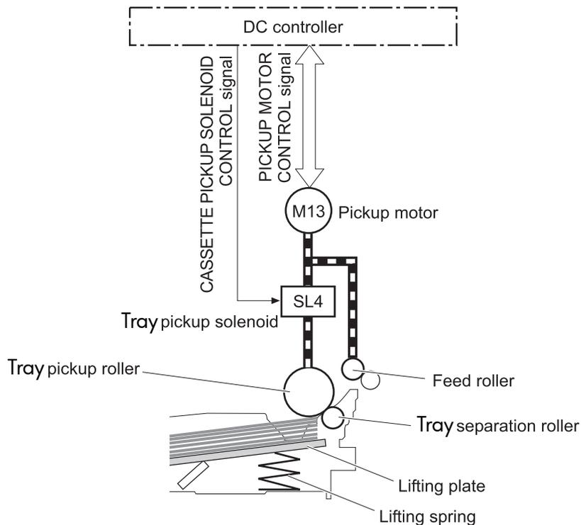
**NOTE:** The lift-up operation lifts the lifting plate to keep the stack surface of the media at a pickup position. The lifting spring helps support the lifting plate depending on the media size and amount.
