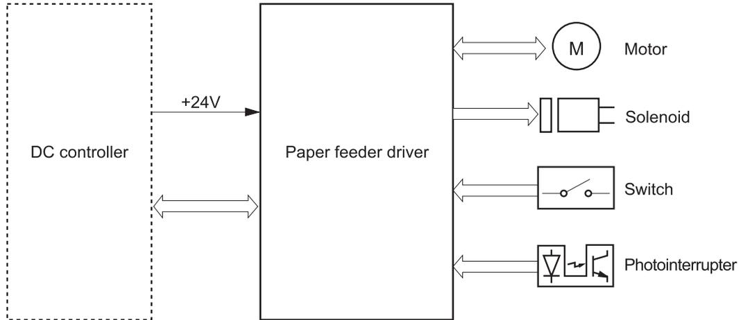
The input trays contain several motors, solenoids, sensors, and switches, as described in the following table.
