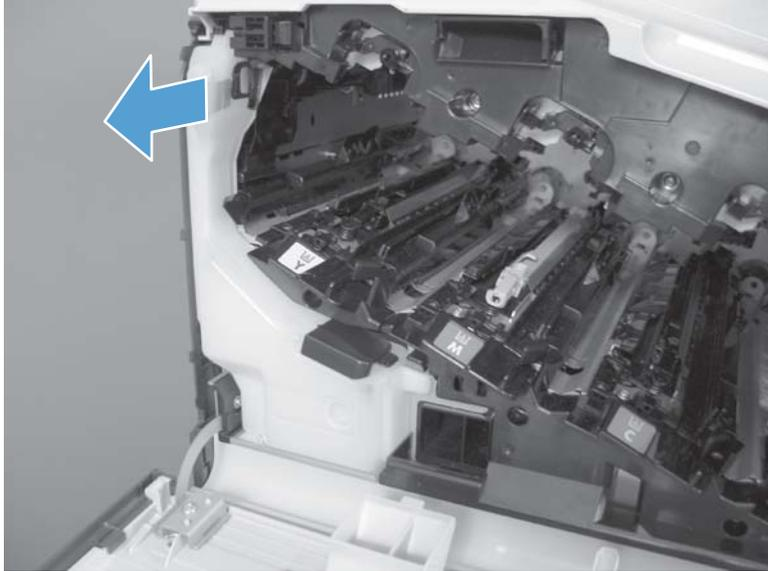
8. Install the replacement TCU obtained prior to beginning the repack the product process.
