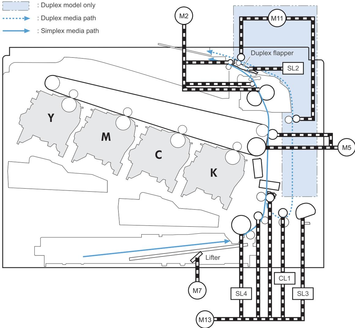
**Table 1-14 Motors and solenoids for the pickup, feed, and delivery system**
