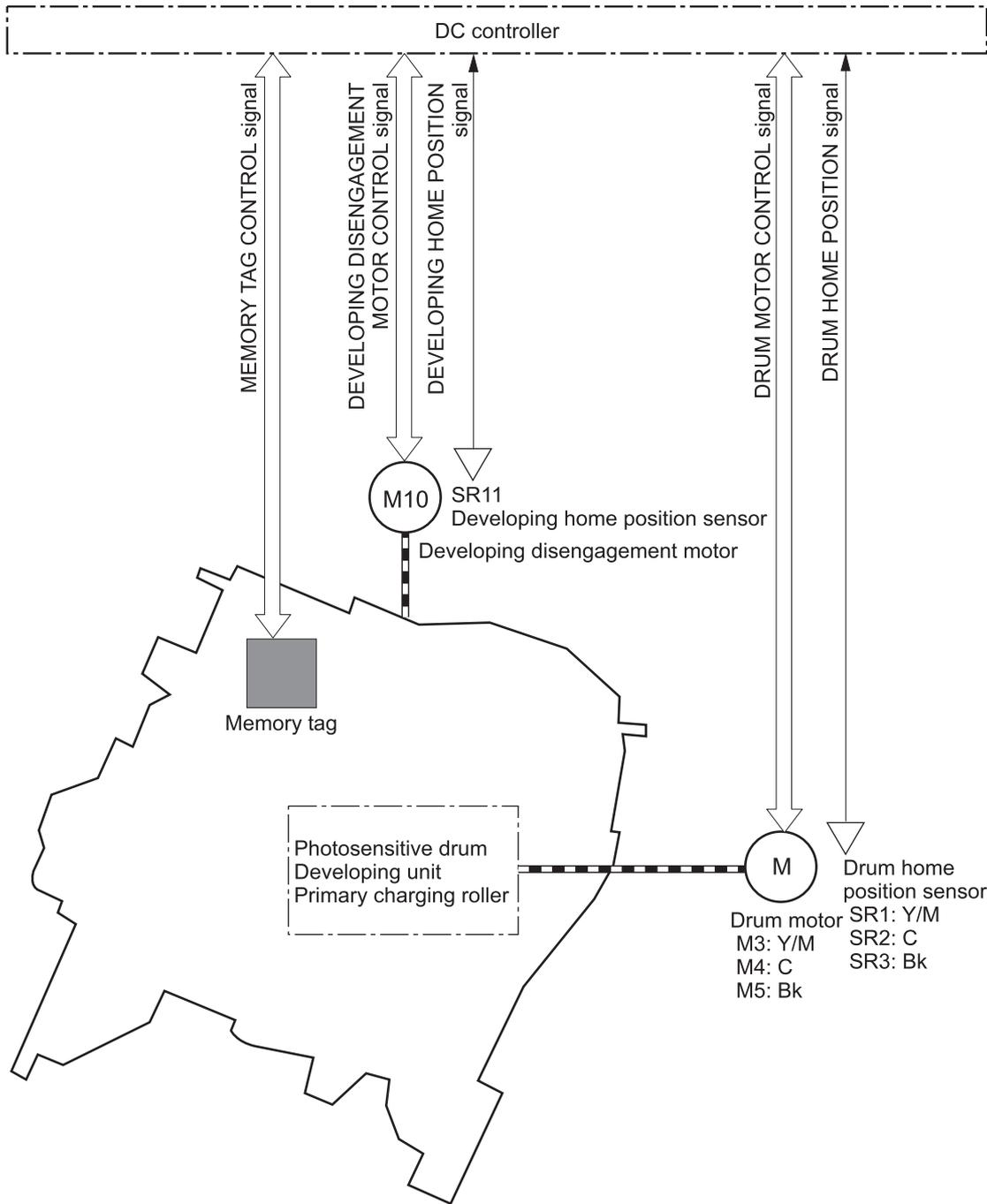
The DC controller rotates the drum motor to drive the photosensitive drum, developing unit, and primary charging roller.
