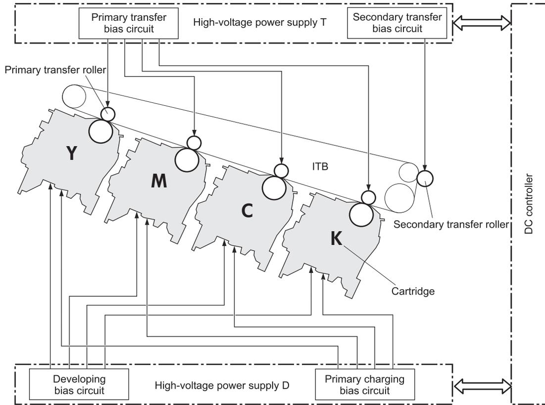
The high-voltage power supply contains several separate circuits.
