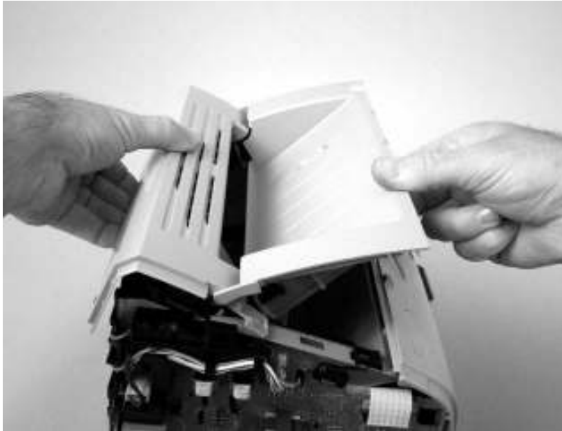
Figure 5-14 Remove the rear panel and top-cover assembly (6 of 6)
