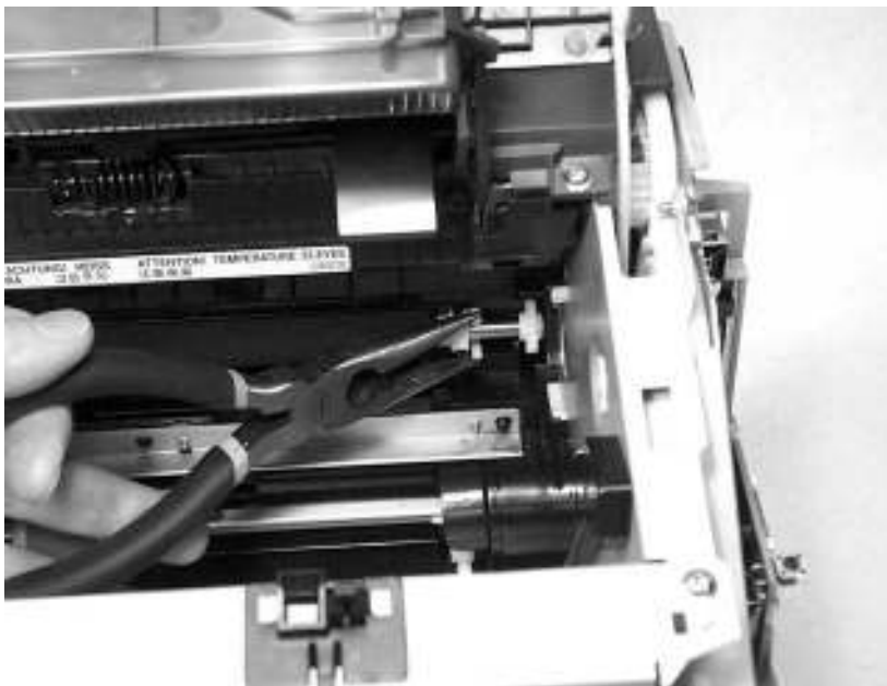
Figure 5-22 Remove the transfer roller (3 of 3)
