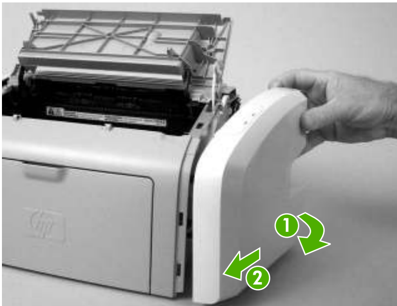
Figure 5-8 Remove the right-side cover (4 of 4; HP LJ 1020 printer shown)
