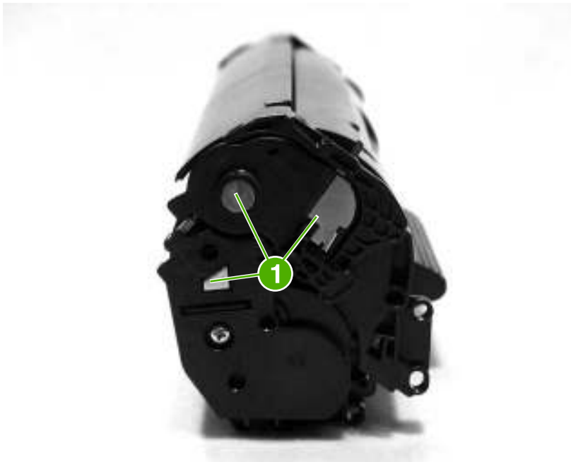
Figure 6-4 Print-cartridge high-voltage contacts
