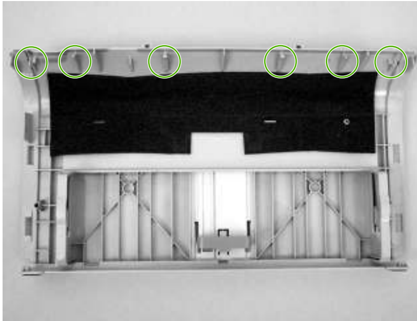
Figure 5-17 Remove the front cover (1 of 3)
