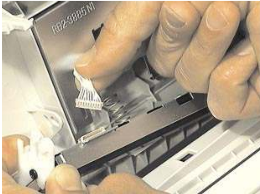
Figure 4-6 Disconnecting the CIS wire connector
