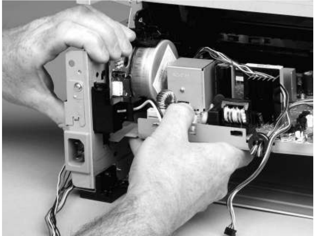
Figure 6-41. Removing the ECU (6 of 8)
