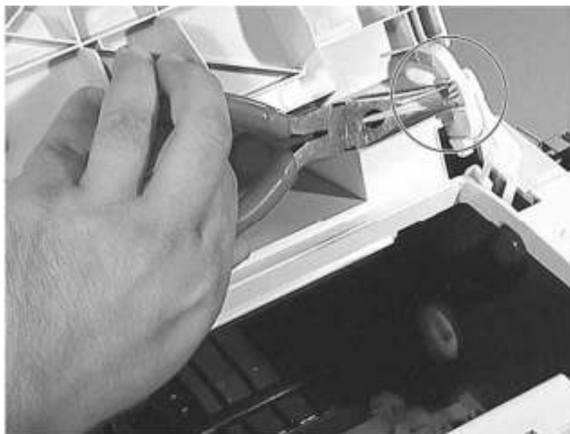
Figure 7-51 Releasing Swing Arm from Toner Cartridge Door
