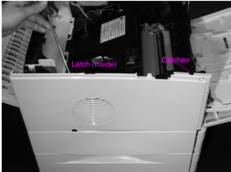
Figure 6-8 Removing the Left Side Cover
