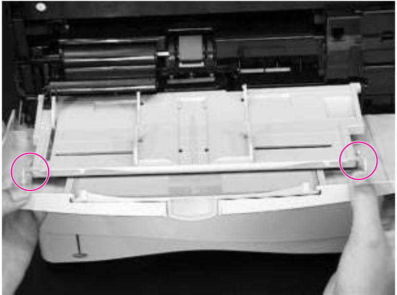
Figure 6-11 Removing Tray 1 from the Front Cover
