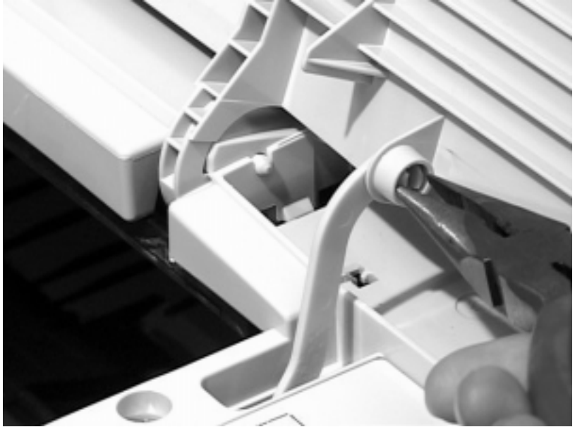
Figure 6-5 Removing the Toner Cartridge Drive Arm
