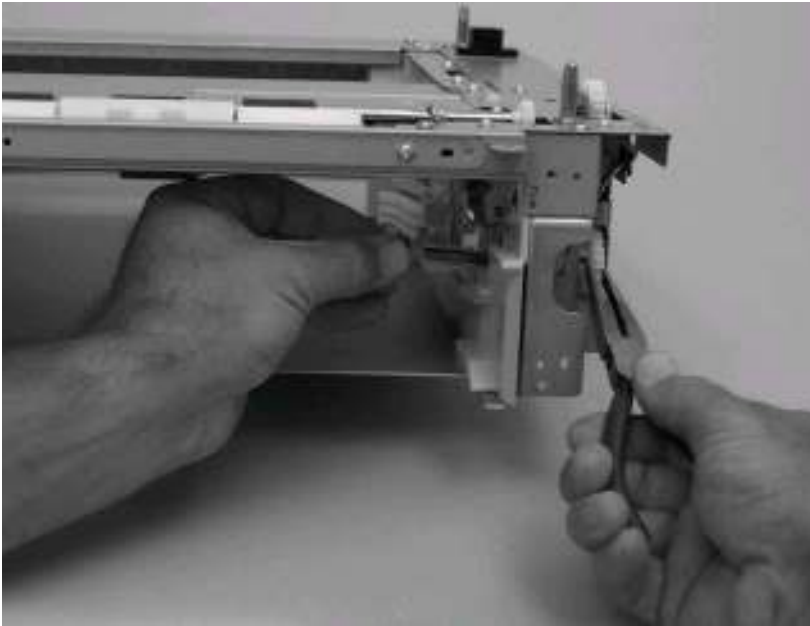
Figure 6-112 500-sheet feeder paper-pickup drive assembly (6 of 7)
