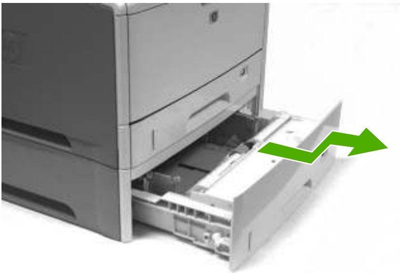
Figure 5-11 Removing the tray 3 retard roller (1 of 2)
