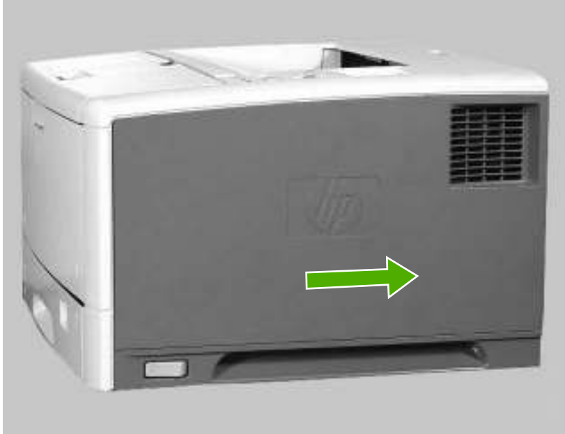
Figure 5-39 Removing the right cover
