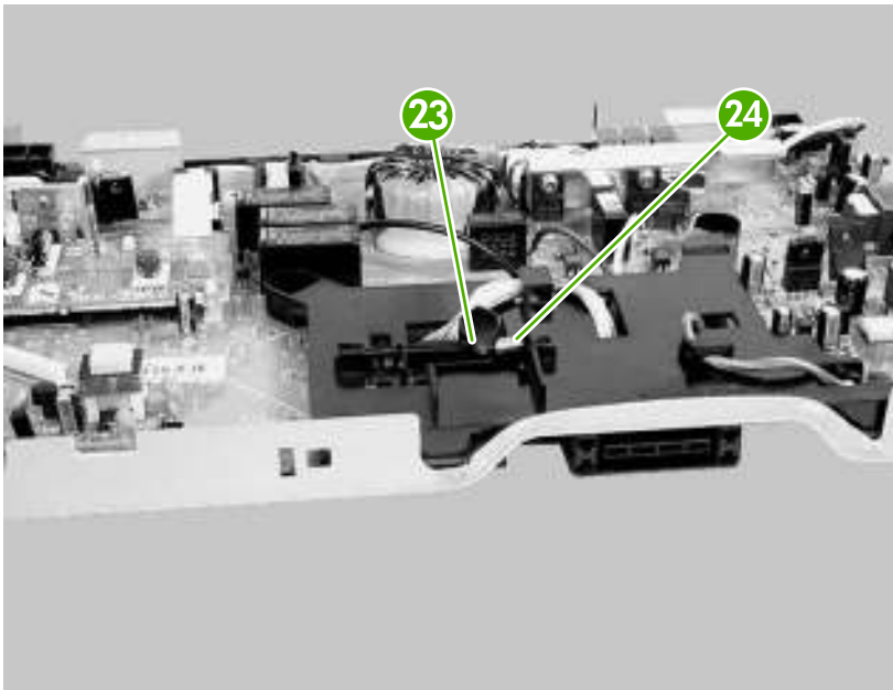
Figure 5-147 Removing the high-voltage power supply (16 of 17)
