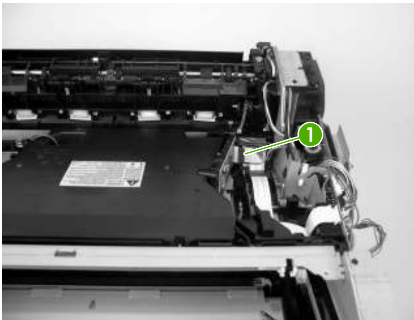
Figure 5-80 Removing the laser/scanner (1 of 3)
