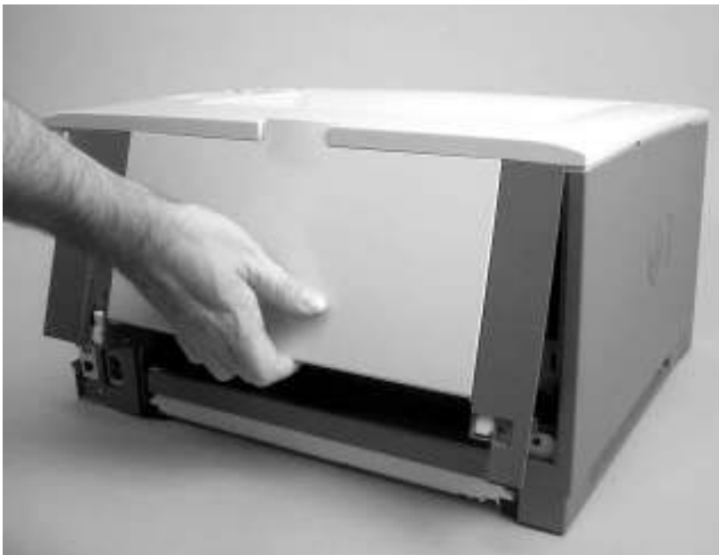
Figure 5-44 Removing the face-up bin (4 of 4)
