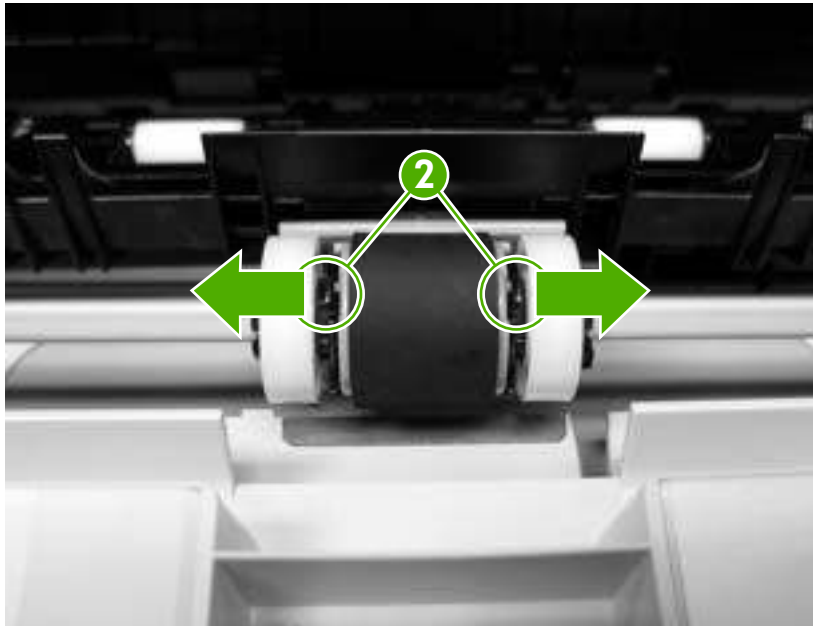
Figure 5-4 Removing the tray 1 pickup roller (2 of 3)
