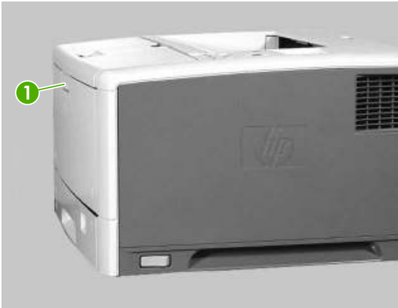
Figure 5-3 Removing the tray 1 pickup roller (1 of 3)
