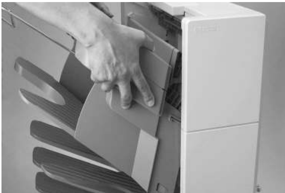
Figure 6-178 Mailbox with Stapler, Stapler Removal or Installation
