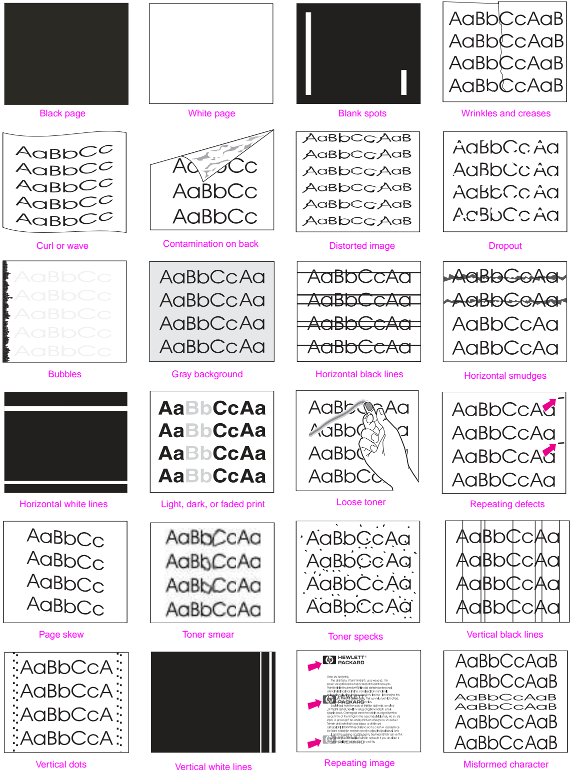
Figure 129. Image defect examples
