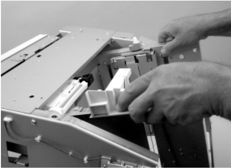
Figure 75. Remove the tray assembly (7 of 7)
