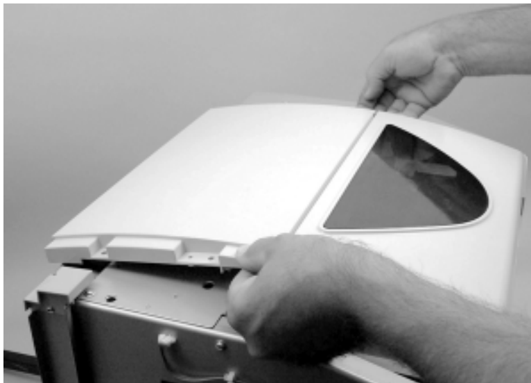
Figure 51. Remove the top-cover assembly (2 of 2)
