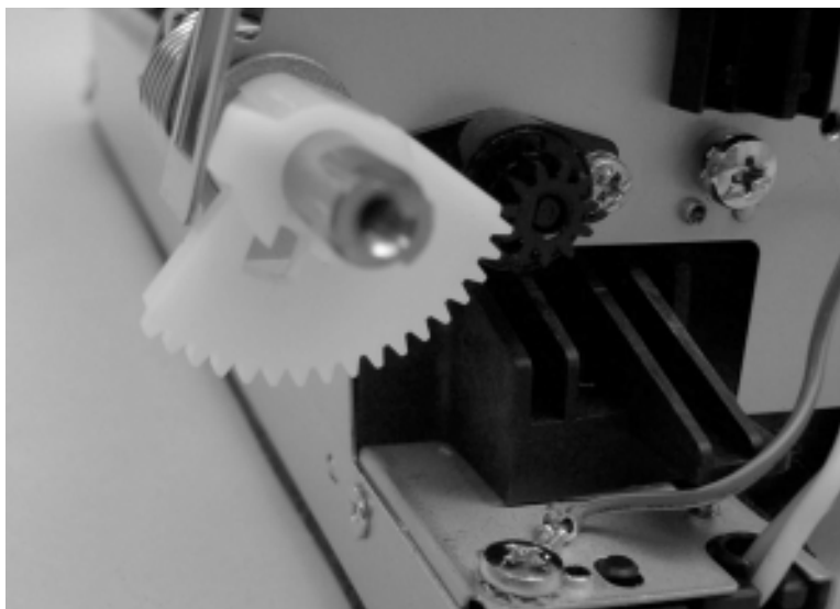
Figure 163. Reinstalling the ADF optic assembly (2 of 2)
