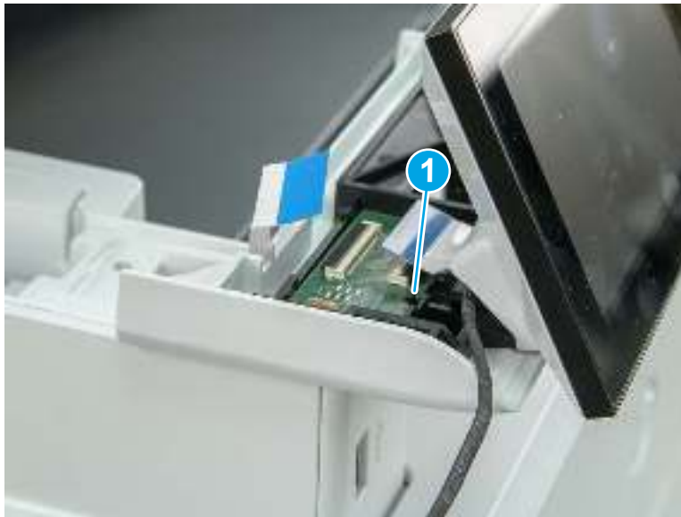
Figure 5-230 Remove the ICB
