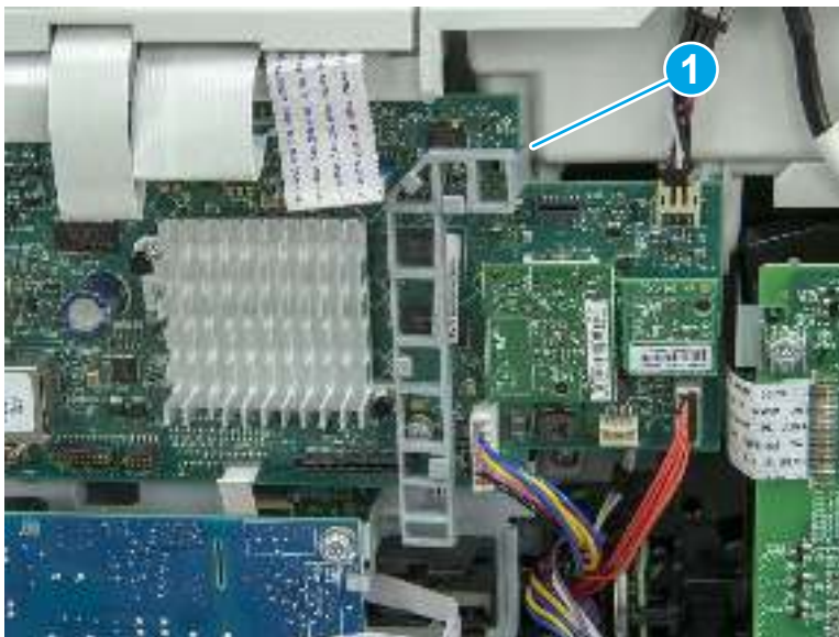
Figure 5-912 Release one tab
