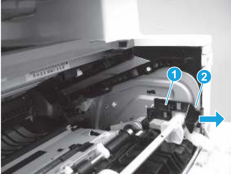
Figure 5-465 Remove the guide
