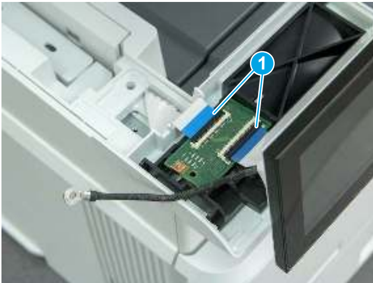
Figure 5-229 Disconnect two FFC
