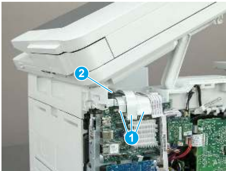
Figure 5-611 Disconnect three FFCs
