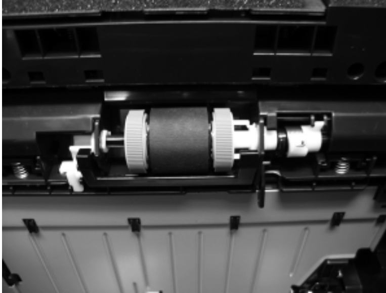
Figure 1-226 Tray 2, 3, or 4 pickup roller assembled
