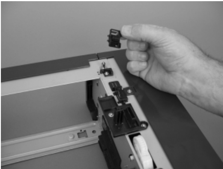
Figure 1-246 Tray 2, 3, or 4 base plate roller assembly (2 of 2)
