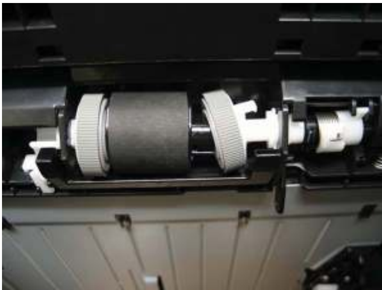
Figure 1-227 Tray 2, 3, or 4 pickup roller disassembled
