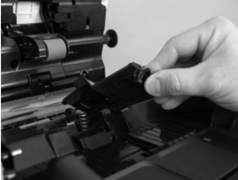
Figure 1-90 Remove the document feeder separation pad (5 of 5)
