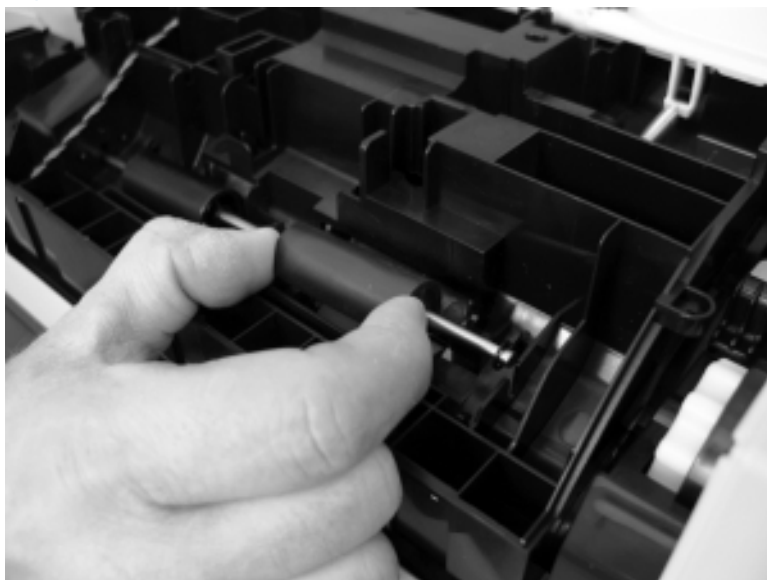
Figure 1-172 Remove the document feeder roller cover (2 of 4)
