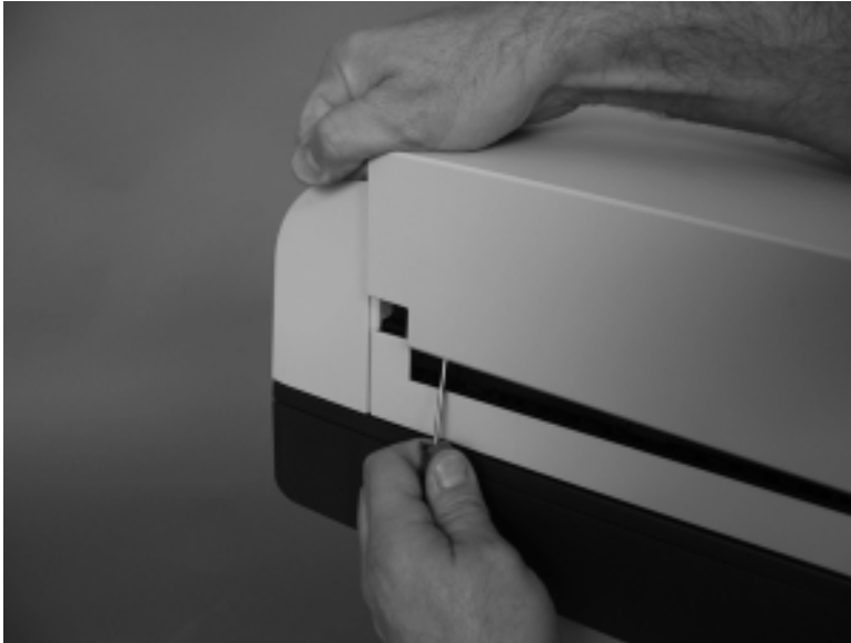
Figure 1-170 Remove the document feeder jam-access cover (5 of 5)
