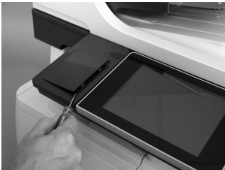
Figure 1-10 Remove the control-panel HIP cover
