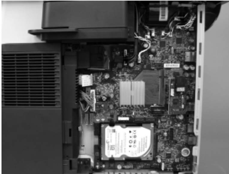
Figure 1-108 Remove the formatter PCA (3 of 4)
