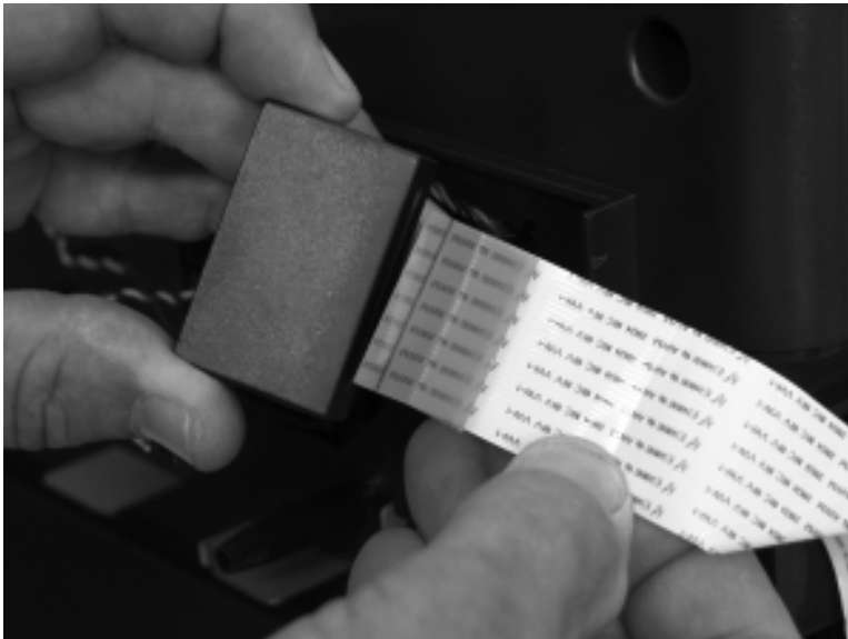
Figure 1-215 Separate the ISA assemblies (525c model; 4 of 7)
