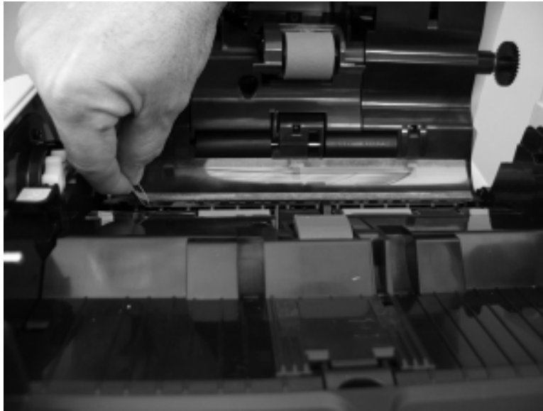
Figure 1-162 Remove the deskew mylar and separation mylar (3 of 3)
