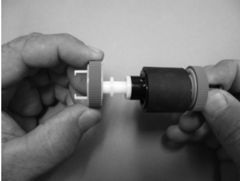
Figure 1-240 Reassemble the Tray 2, 3, or 4 pickup roller assembly (8 of 9)
