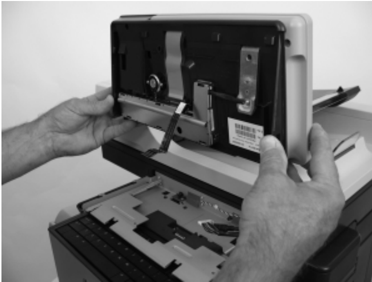
Figure 1-34 Remove the control-panel assembly (13 of 13)
