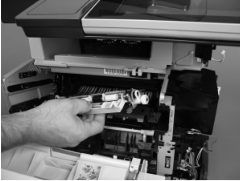
Figure 1-261 Removing the registration roller assembly (3 of 3)
