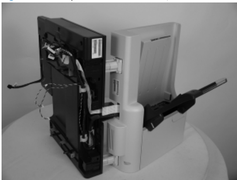
Figure 1-212 Separate the ISA assemblies (525c model; 1 of 7)
