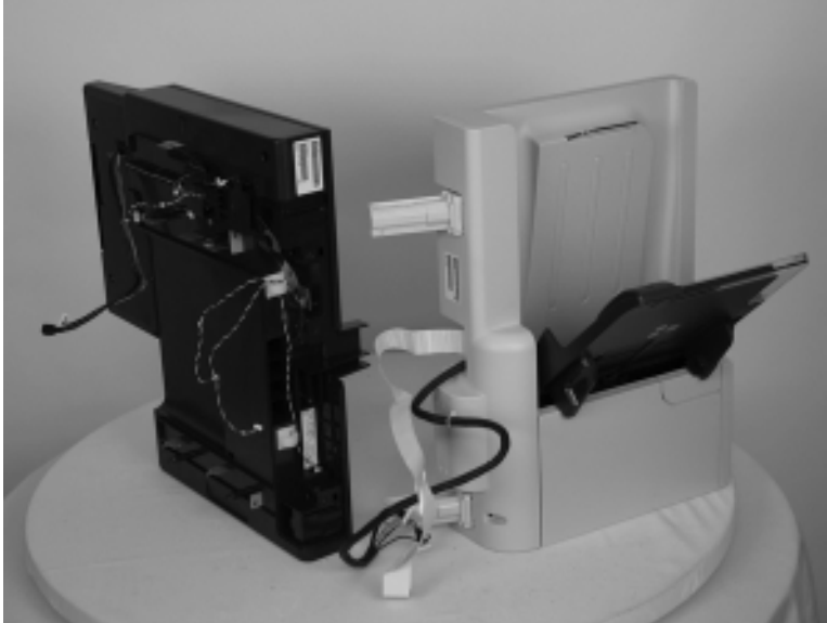
Figure 1-218 Separate the ISA assemblies (525c model; 7 of 7)
